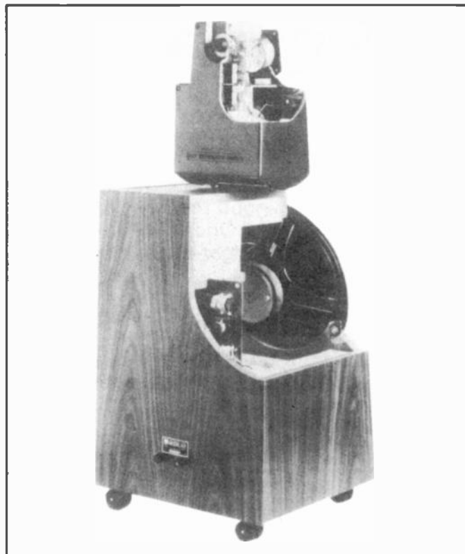
Figure 6. This revealing cutaway of the KEF 105 II loudspeaker shows the level of complexity that top-end designs can require. The bottom enclosure contains the bass-driver and crossover while the pivoted 'head' carries the (cone) midrange and the (dome) high frequency units. You can see the protection circuitry, which makes this speaker virtually invulnerable, behind the rear of the head. This is a design in which practically all the parameters concerned with an enclosure have been optimised. Even the edges of the top enclosure are rounded off, to prevent sharp corners interfering with sound dispersion. In addition, the bass-driver is 'developed' from the box in such a way that vibrations from the framework are prevented from reaching the enclosure itself, where they would colour the output.
