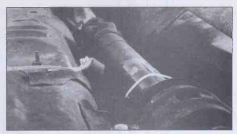
Installation of the speed sensor.
