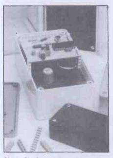
Above: Plastic mounting strips simplify the problem of securing a PCB or Veroboard within a case.
