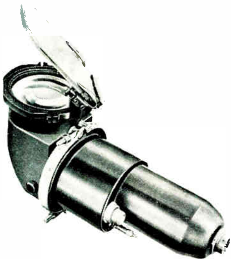
▼ The pilot's display unit showing the reflector, lens and c.r.t. mount
