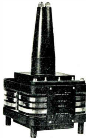
A selection of vibration generators with their associated driving and monitoring equipment will be displayed on the Goodmans stand. The VG.1K. Mk. 1 (illustrated) will be shown in operation. It has an overall weight of 1,260 lb. a maximum thrust of more than 1,000 lb and an excursion of \frac{1}{2} in (77)
