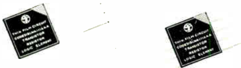
Transistor-Resistor Logic Elements (actual size).
