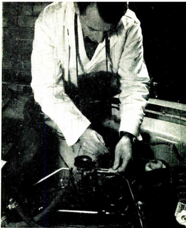
For work which cannot be taken to a bench-type marking unit, such as marking jet sizes on a modified carburettor, the portable Electromark type BT400 provides an ideal solution
