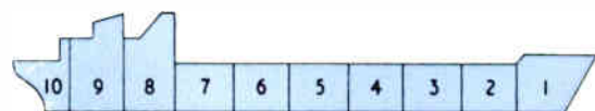
Fig. 3. A ship may be dissected into ten sections each of which is represented by an equivalent electrical network in the calculator
