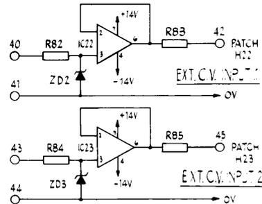
Fig. 42 Circuit Diagram of External Control Voltage Inputs
