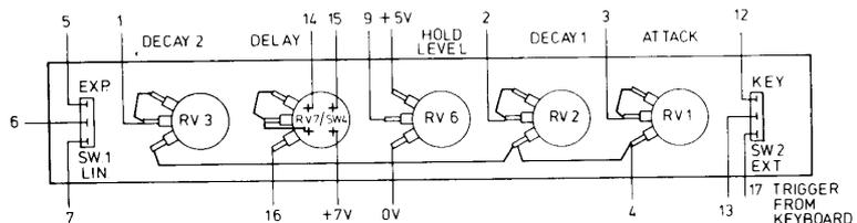
Fig. 24 Front Panel Wiring for Envelope
