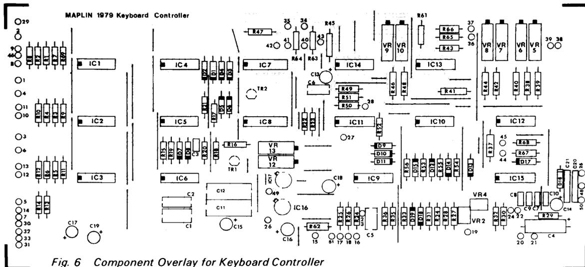
Fig. 6 Component Overlay for Keyboard Controller
