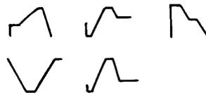
If the 'hold delay' pot, RV5, is switched off, the 'key hold' time replaces the hold delay, and, if the 'key hold' time is less than 'delay 1', then at the completion of 'delay 1', 'slope 2', and 'final level' will be selected — thus eliminating 'slope 1' and 'hold level'.
