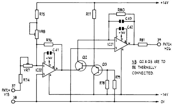
Fig. 43 Circuit Diagram of Exponential Converter
