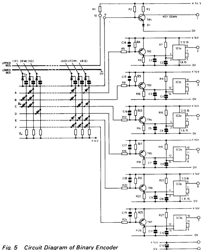
Fig. 5 Circuit Diagram of Binary Encoder
