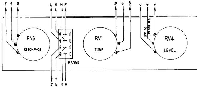
Fig. 53 Front Panel Wiring for VCF (5600S only)
