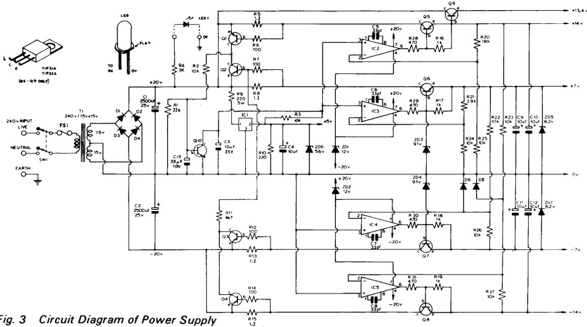
Fig. 3 Circuit Diagram of Power Supply
