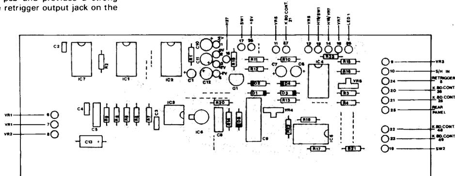
Fig. 17 Component Overlay for Sample and Noise
