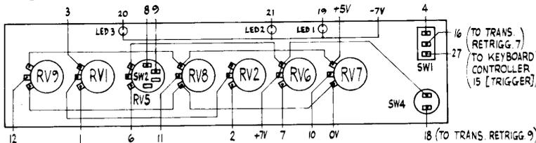
Fig. 32 Front Panel Wiring for Transient 'B'
