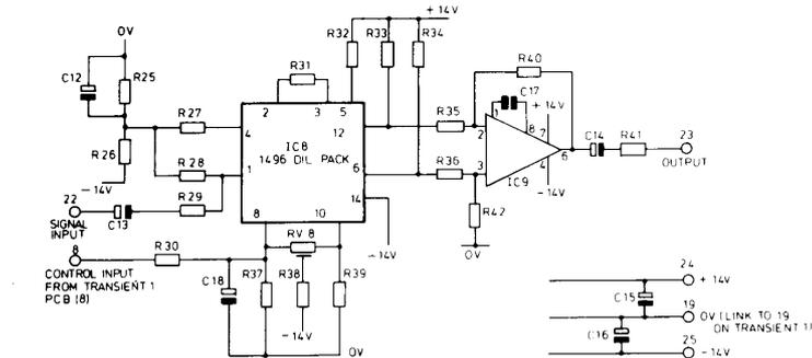
Fig. 23 Circuit Diagram of VCA Used In Envelope
