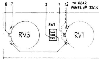
Fig. 61 Front Panel Wiring for External Inputs (3800 only)
