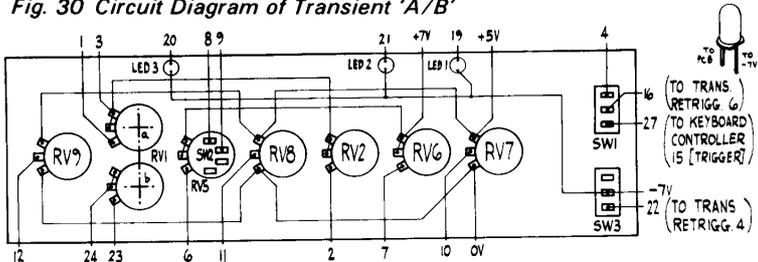
Fig. 31 Front Panel Wiring for Transient 'A'
