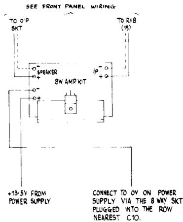
**Fig. 68 Wiring of Headphone Amplifier (3800 only)**
