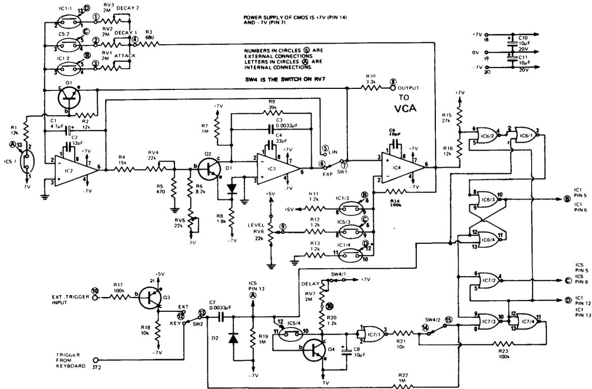
Fig. 21 Circuit Diagram of Transient Used In Envelope
