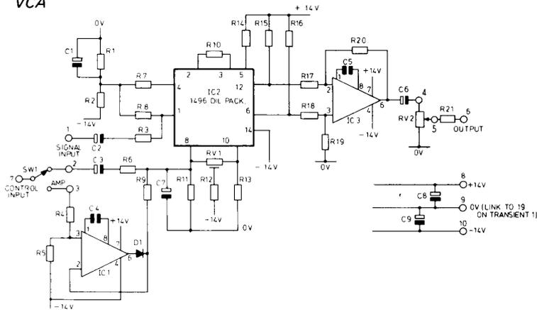
Fig. 26 Circuit Diagram of VCA
