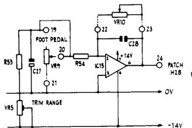
Fig. 40 Circuit Diagram of Foot Pedal Circuitry
