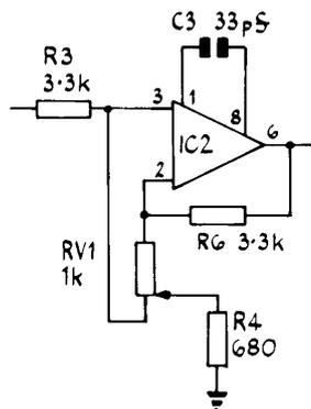
Fig. B Equivalent circuit of the equaliser with the potentiometer set for maximum cut at the resonant frequency of the network.
