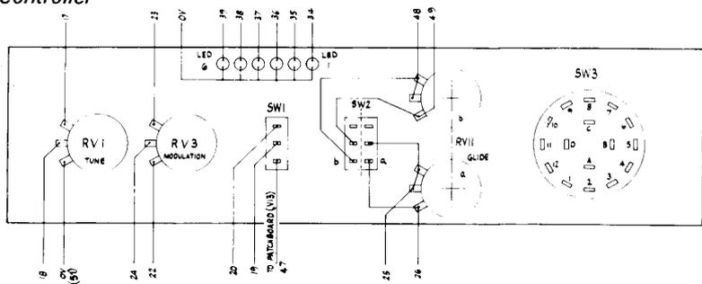
**Fig. 8** Front Panel Wiring for Keyboard Controller
