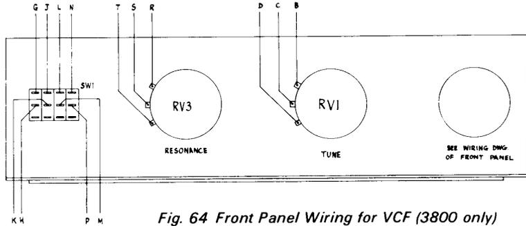
Fig. 64 Front Panel Wiring for VCF (3800 only)
