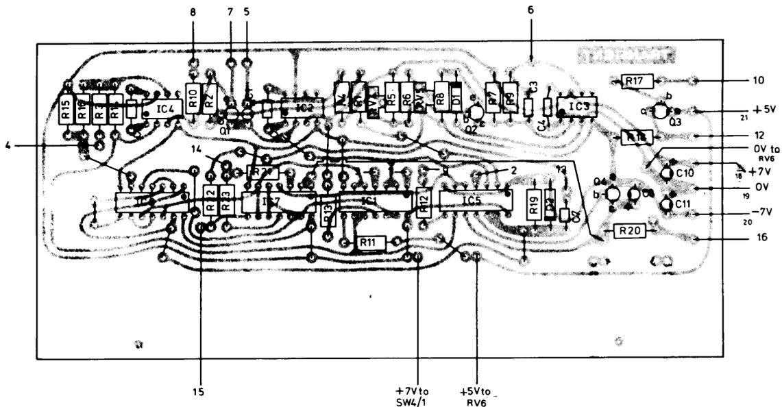
Fig. 20 Component Overlay for Transient Used In Envelope
