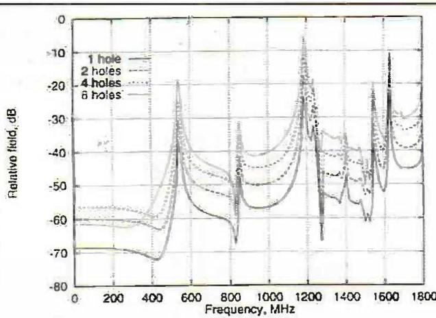
Figure 4. Effects of increasing number of holes.
