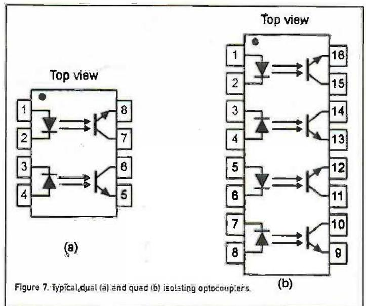
Figure 7. Typical dual (a) and quad (b) isolating optocouplers.
