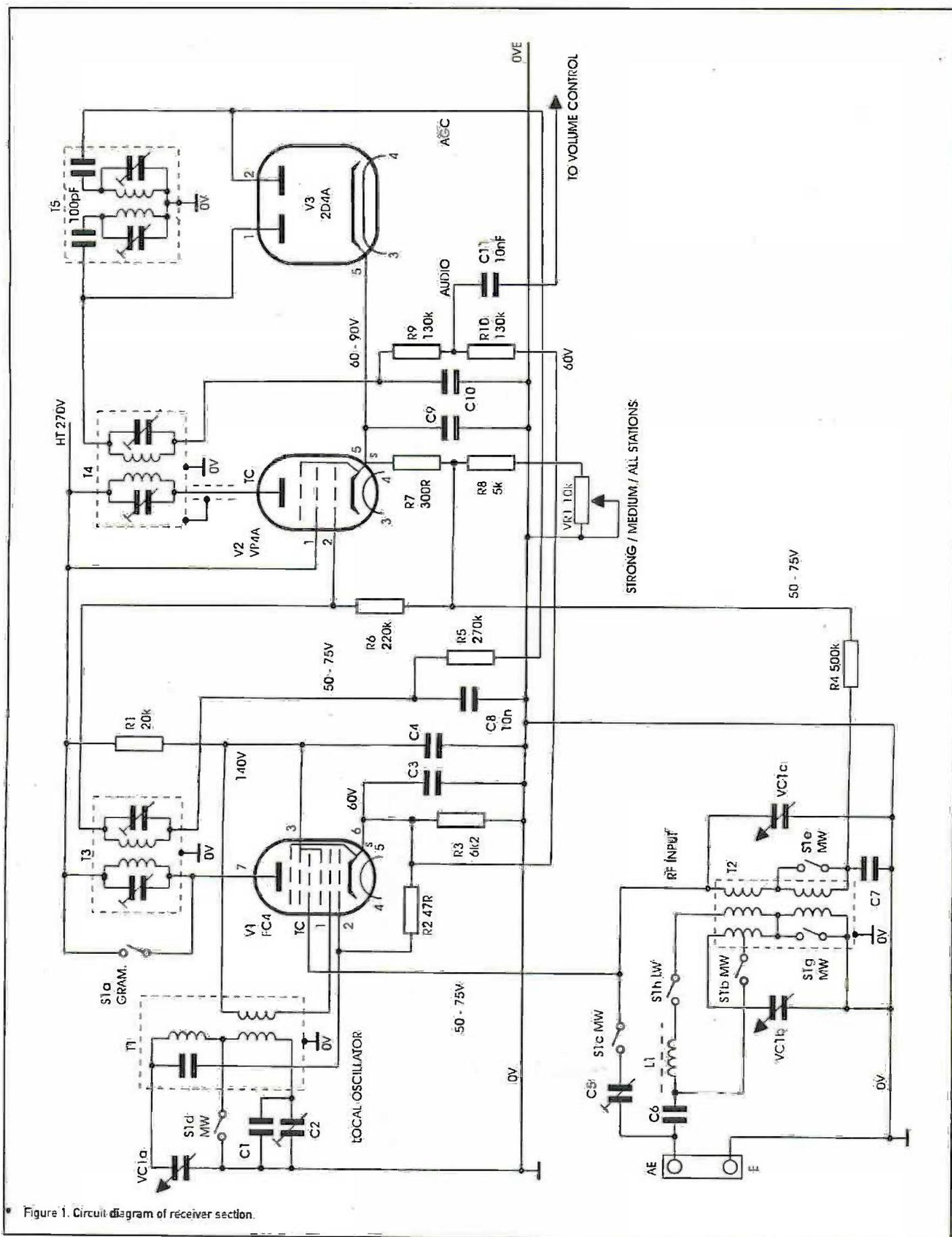
Figure 1. Circuit diagram of receiver section.
