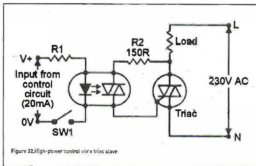
Figure 22. High-power control via a triac slave.
