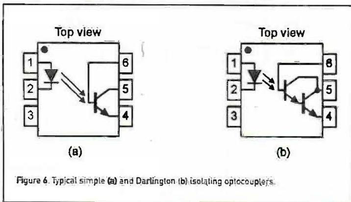
Figure 6. Typical simple (a) and Darlington (b) isolating optocouplers.
