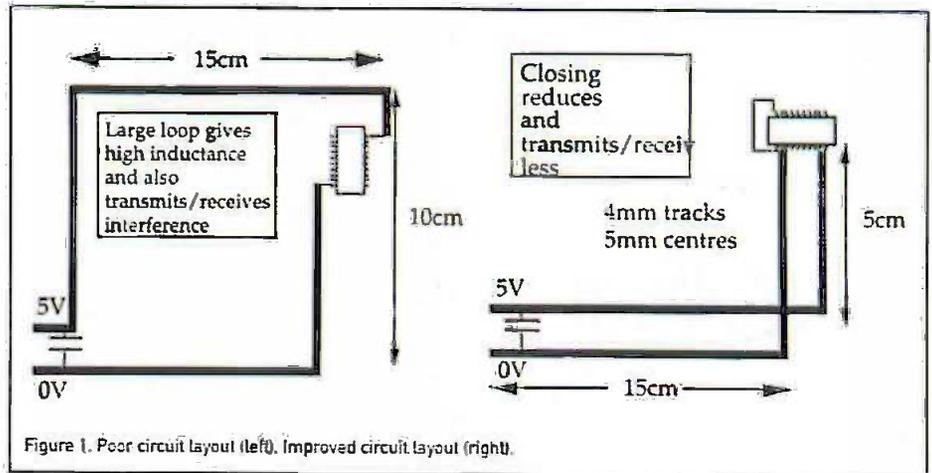
Figure 1. Poor circuit layout (left). Improved circuit layout (right).
