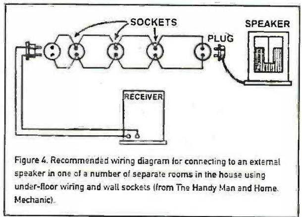
Figure 4. Recommended wiring diagram for connecting to an external speaker in one of a number of separate rooms in the house using under-floor wiring and wall sockets (from *The Handy Man and Home Mechanic*).
