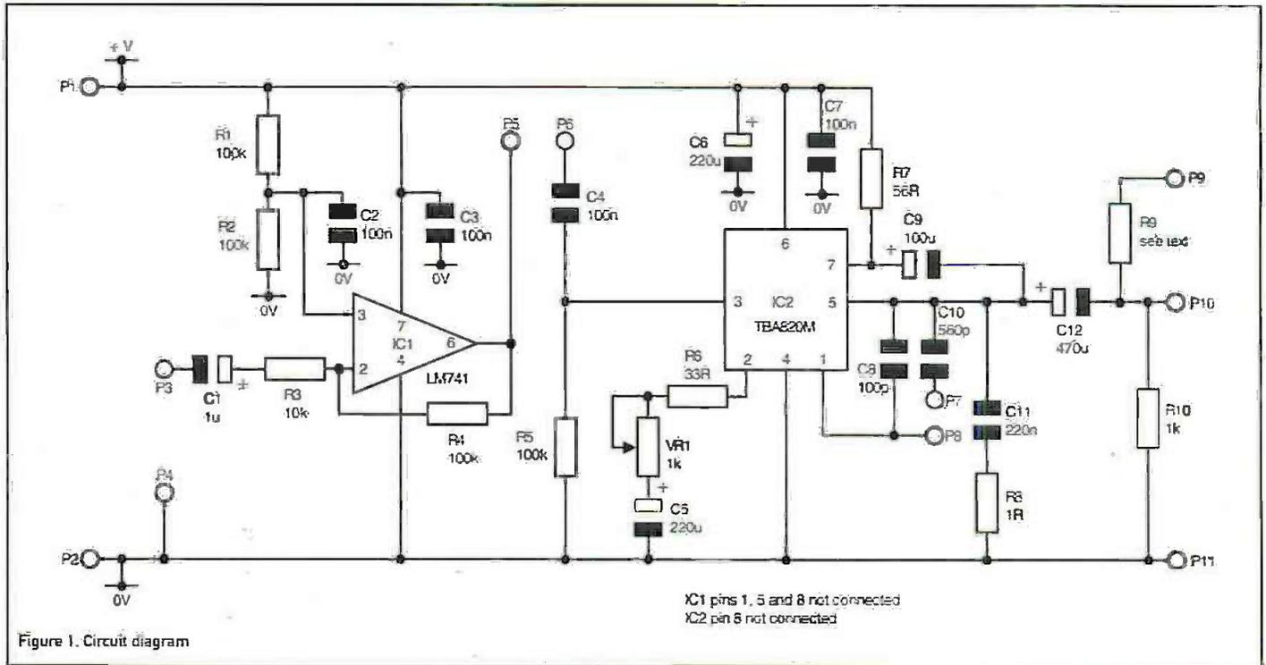
In this article we look at a low power audio amplifier with a host of different uses. The circuit is easy to construct and uses readily available components. It is ideal as a headphone amplifier, for applications such as intercoms and door phones and as an add-on to existing projects such as simple radio receivers.
