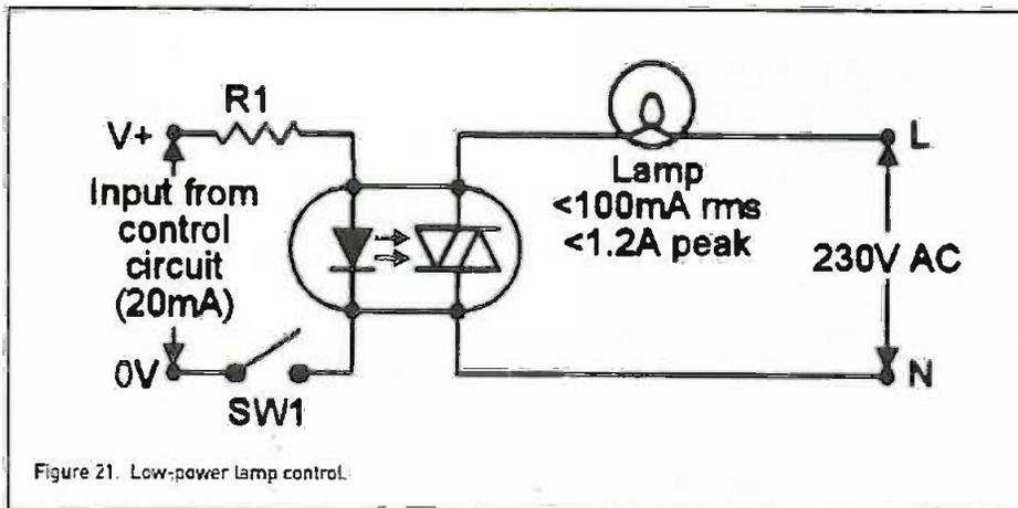
Figure 21. Low-power lamp control.
