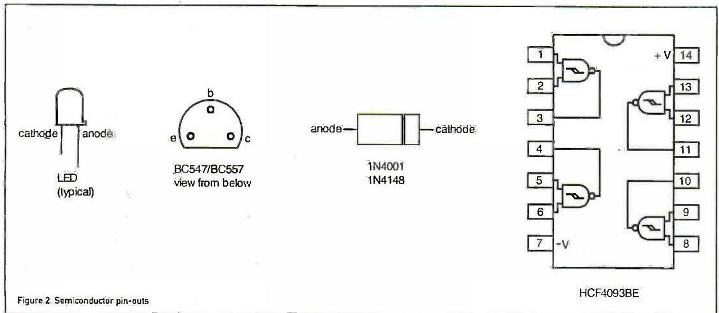
Figure 2. Semiconductor pin-outs
