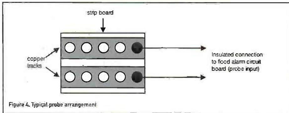
Figure 4. Typical probe arrangement
