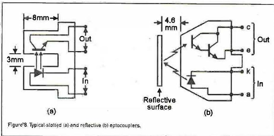
Figure 8 Typical slotted (a) and reflective (b) optocouplers.
