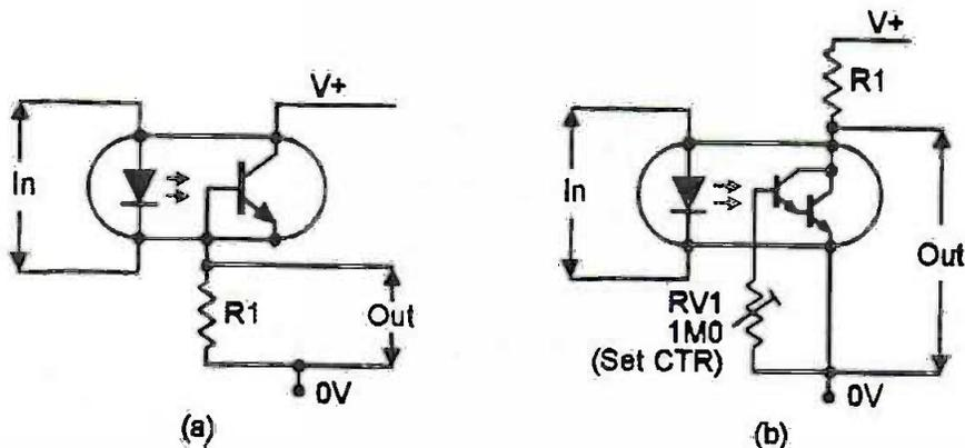
Figure 13. If its base is available, the phototransistor can be made to function as a photodiode (a), or its CTR values can be varied via RV1 (b).
