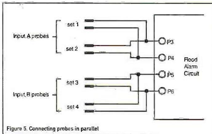
Figure 5. Connecting probes in parallel
