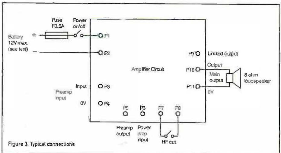
Figure 3. Typical connections
