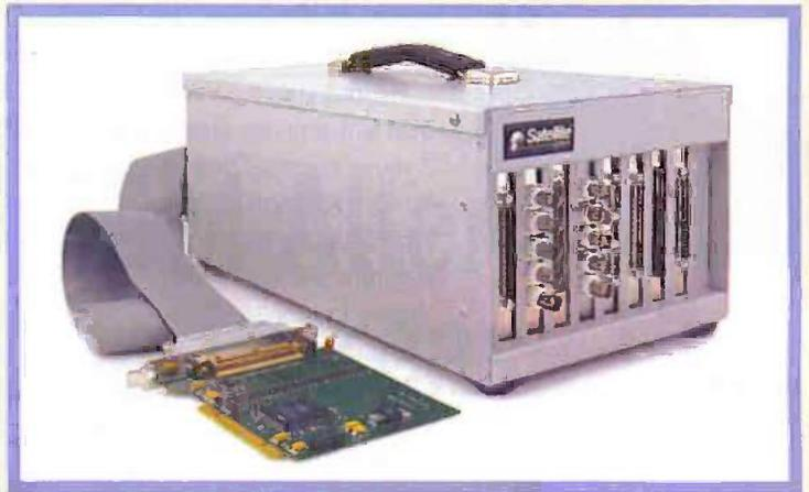
The Satellite chassis includes an internal monitoring system that continually measures power supply voltages, air temperature between each slot, and cooling fan functionality. Software supplied with the chassis allows users to easily monitor their system. The software program is accessible through VB/C++ examples and a DLL file.
