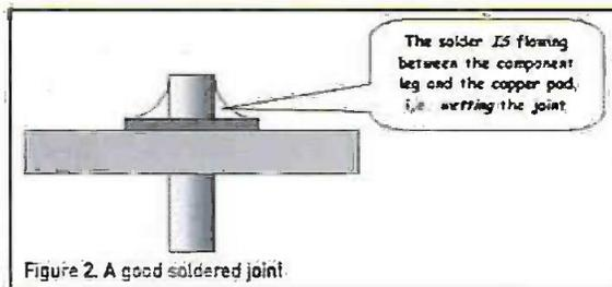
Figure 2. A good soldered joint
