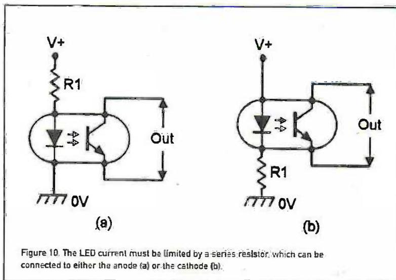
Figure 10. The LED current must be limited by a series resistor, which can be connected to either the anode (a) or the cathode (b).
