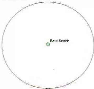
With three base stations the user can only be at one point on the signal distance perimeters giving a firm positional fix, more base stations will improve the positional accuracy
