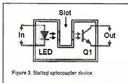
Figure 3. Slotted optocoupler device.
