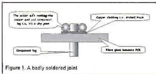
Figure 1. A badly soldered joint
