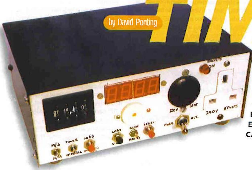
MAKING PRINTED CIRCUITS THROUGH THE PHOTOGRAPHIC PROCESS OF EXPOSING TO UV LIGHT THE SENSITISED SURFACE OF A COATED COPPER BOARD REQUIRES THE EXPOSURE TIME TO BE CAREFULLY CONTROLLED.
