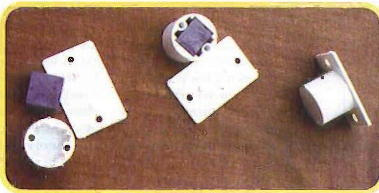
round version of magnetic reed switches normally used as door-open sensors in a burglar alarm system. Each reed switch comes as a pair: the magnetic half is the one with no connection terminals. Conveniently the flat face peels away from the cylindrical section, revealing a small magnet only fractionally thicker than the material of the door. Cutting into the door edge a square which is slightly
