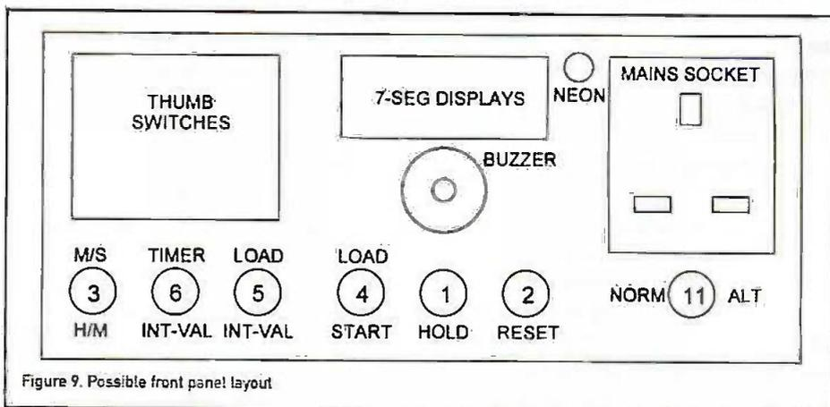
Figure 9. Possible front panel layout
