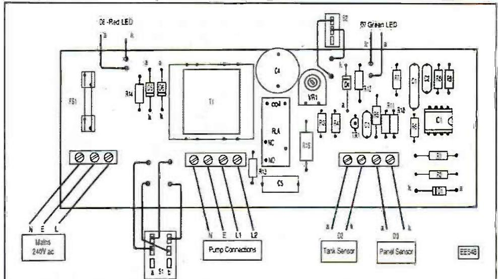
Figure 5. Component layout and interwiring details
