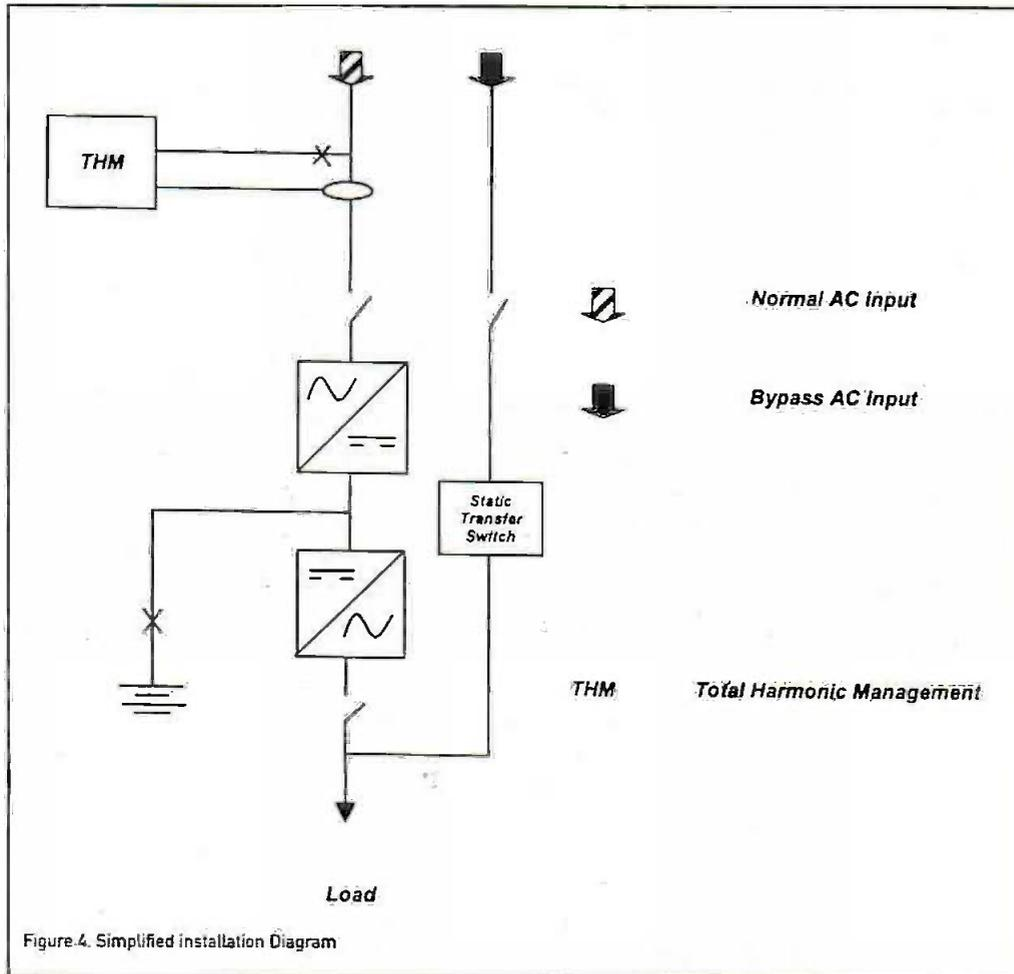
Figure 4. Simplified installation Diagram
