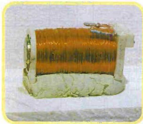
Use Milliput Putty to secure the electro-magnet
