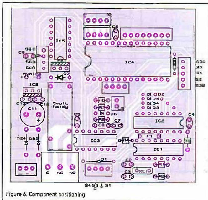
Figure 6. Component positioning
