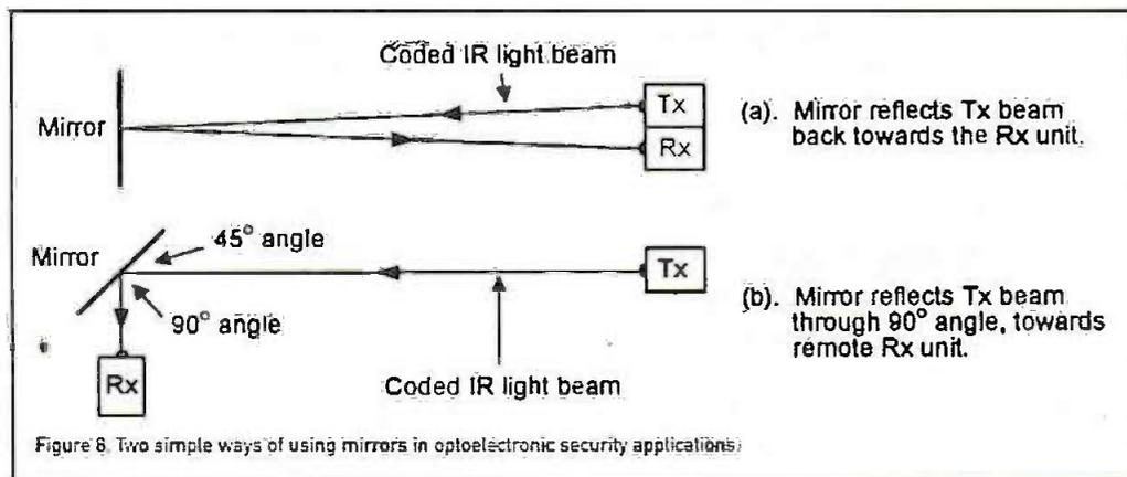
Figure 8. Two simple ways of using mirrors in optoelectronic security applications.
