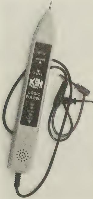
Photo 15 CMOS/TTL logic pulser which may be used to inject pulses into digital circuits. This device is similar in appearance to a logic probe. Maplin order code: YU56L (matching logic probe, Maplin order code: FY73Q)
