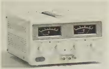
Photo 1 30 V 6 A regulated d.c. power supply. The power supply has separate voltage and current controls. The line and load regulation is typically better than 0.02 per cent. Maplin order code: GW14Q
