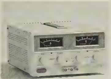
Photo 2 Dual tracking power supply capable of delivering up to 30 V at 3 A. The two supplies may be operated independently or configured so that the output voltages are accurately tracked (in this mode, the right-hand power supply is the 'master' while the left-hand supply is the 'slave'). Maplin order code: GW11M
