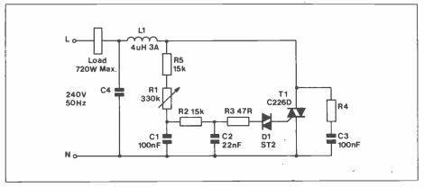
Figure 13. Lamp-dimmer or speed-controller for an AC series commutator motor
