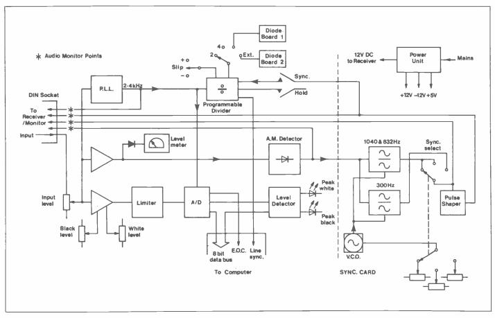
Figure 2. Decoder Block Schematic.
