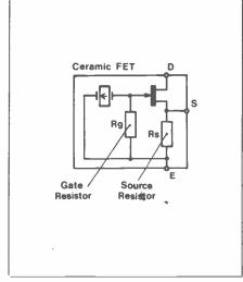
Figure 4. Proximity detector Circuit.
