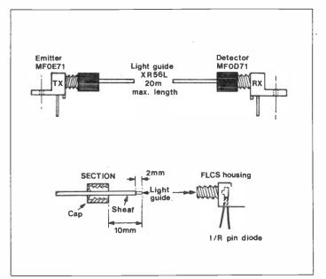
Figure 1. Connecting Light Guide.
