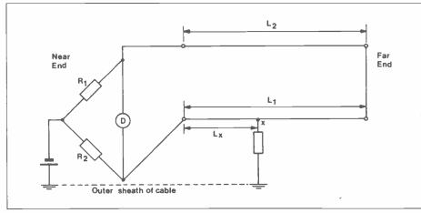
Figure 5. Murrary Loop Test.
