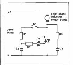
Figure 12. Practical Triac switch for a motor-driven appliance (for component values see Appendix 3).
