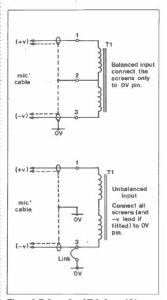
Figure 1. Balanced and Unbalanced Lines.
