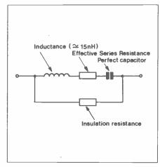
Figure 3. Capacitor equivalent circuit.
