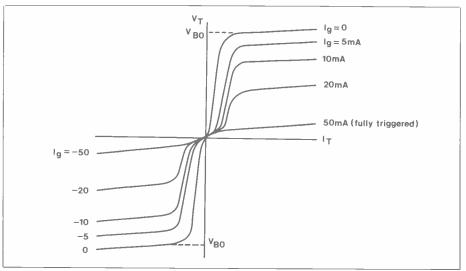
Figure 3. Triac main voltage/main current characteristics with gate current as parameter
