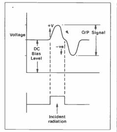
Figure 3. Source Output Voltage Swing.
