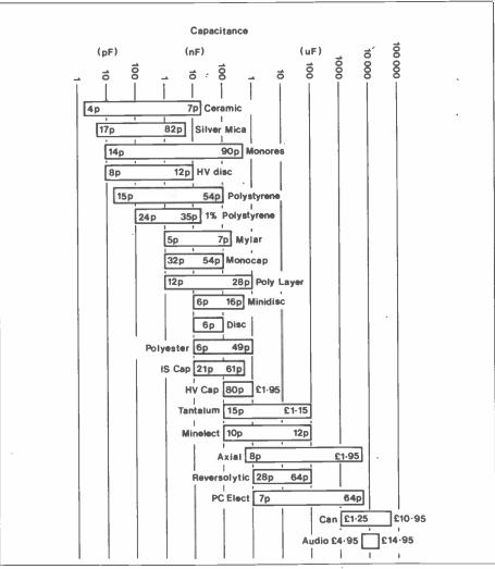
Figure 1. Capacitance range offered by different types.
