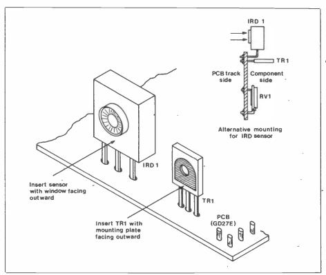
Figure 7. Mounting arrangements.
