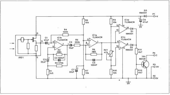
Figure 2. Sensor Circuit.
