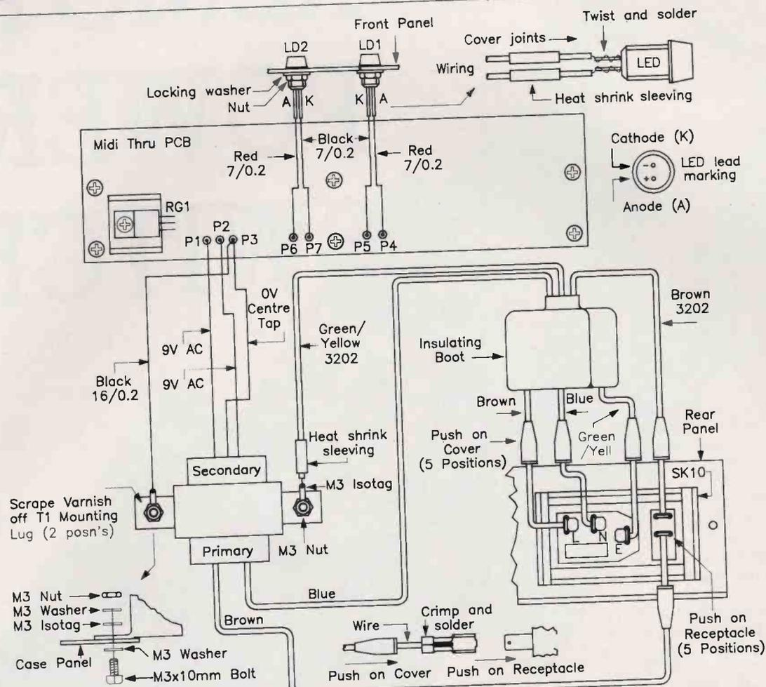
Figure 8. Wiring and assembly diagram.
