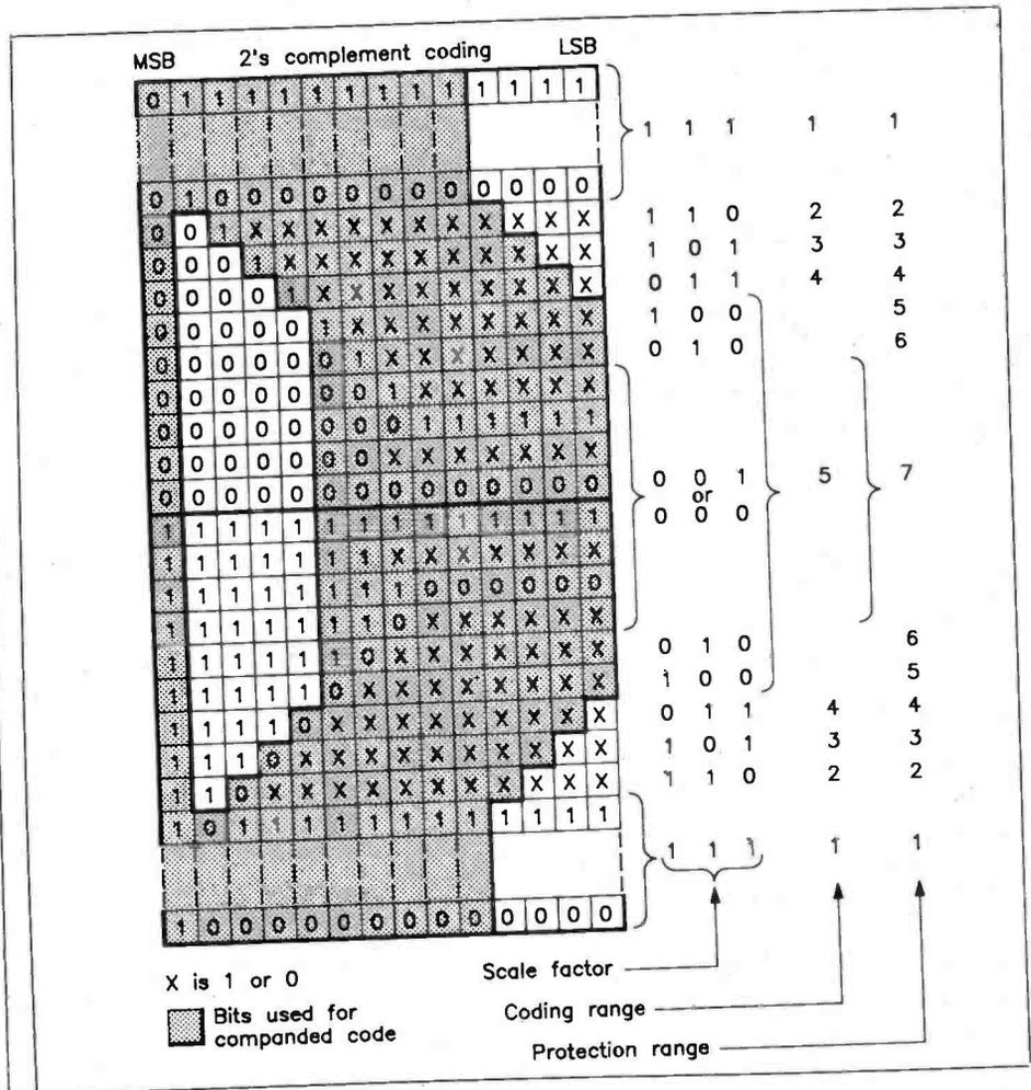
Figure 5. Coding of companded sound signals.
