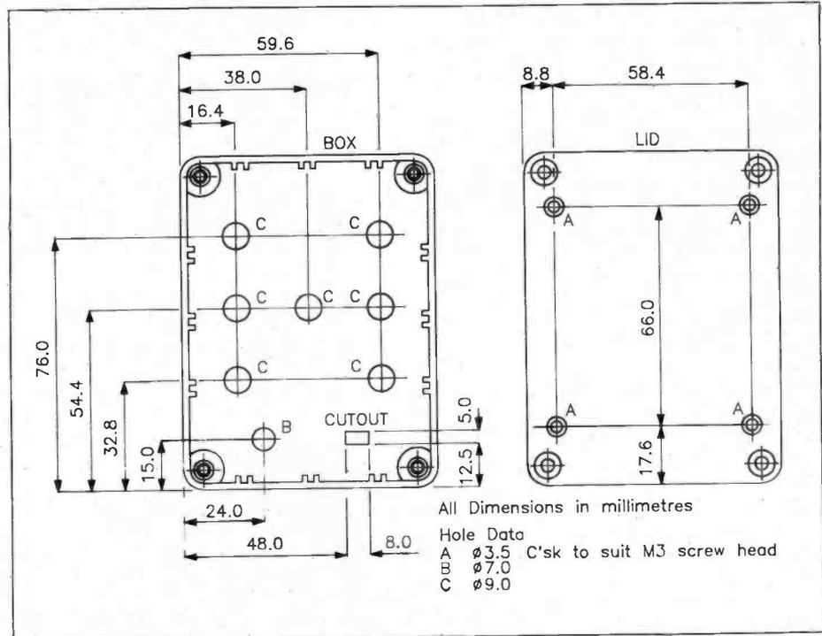
Figure 5. Drilling Details.
