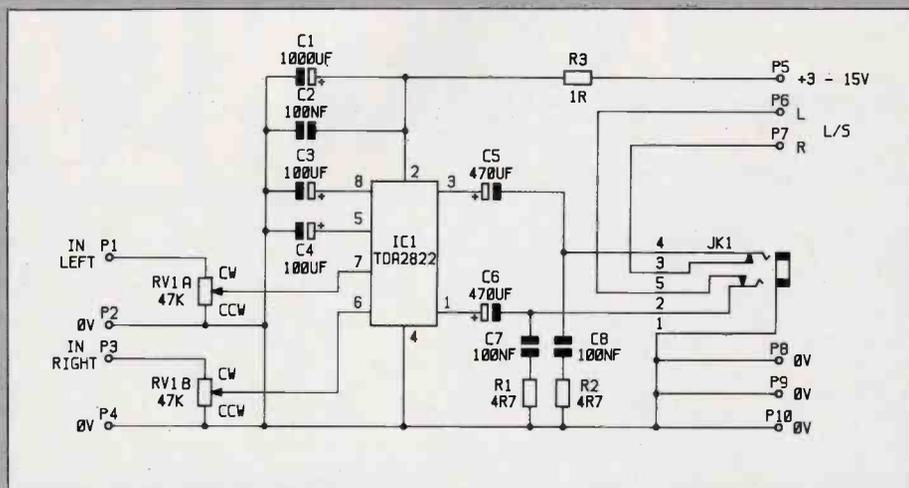
Figure 3. Circuit diagram.
