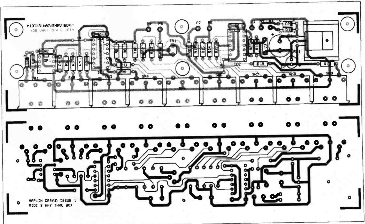
Figure 5. PCB legend and foil pattern.
