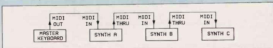
Figure 1. Connecting synthesisers using MIDI chain.
