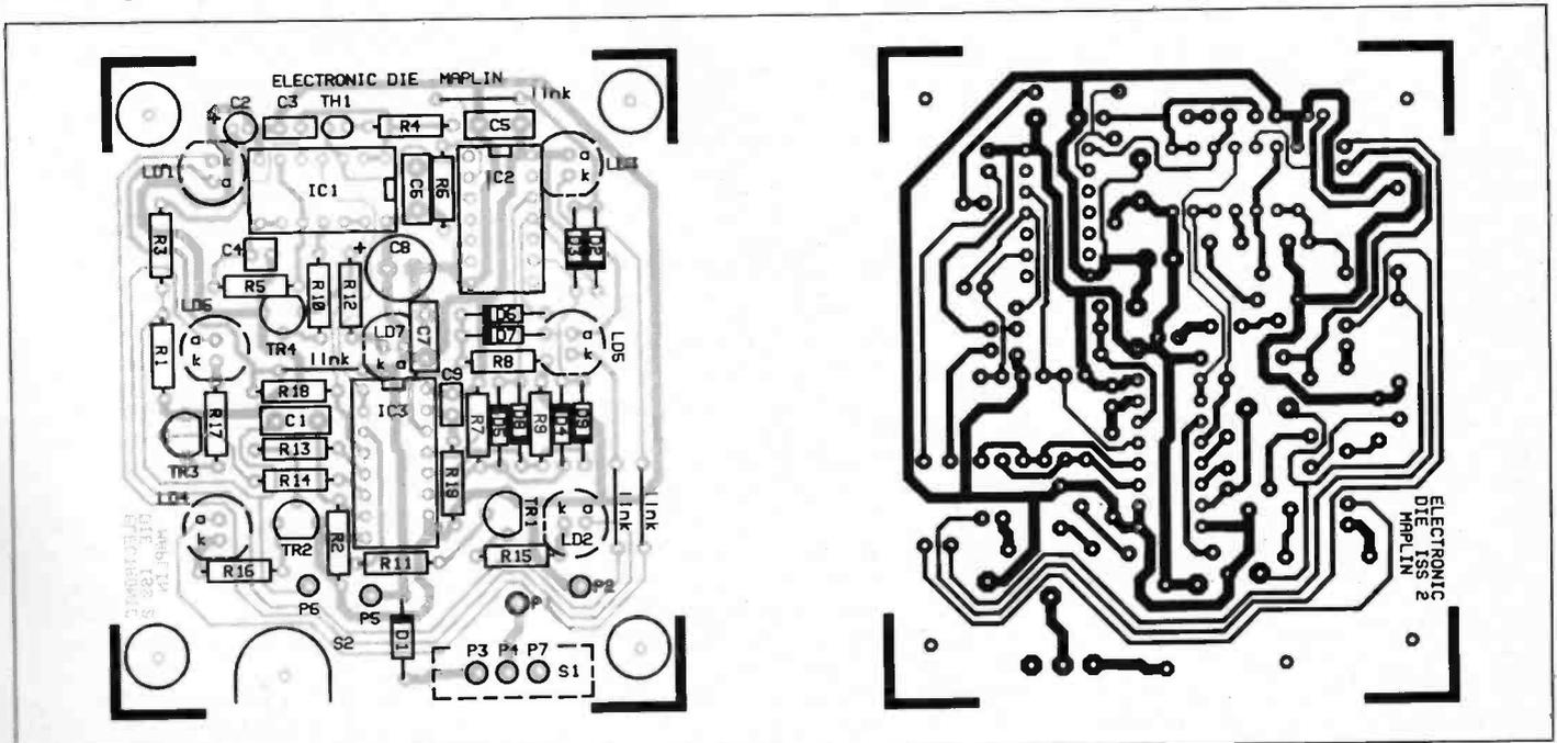
Figure 2. PCB Layout.
