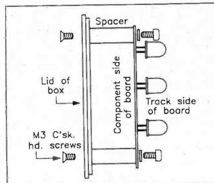
Figure 6. Installing the PCB.
