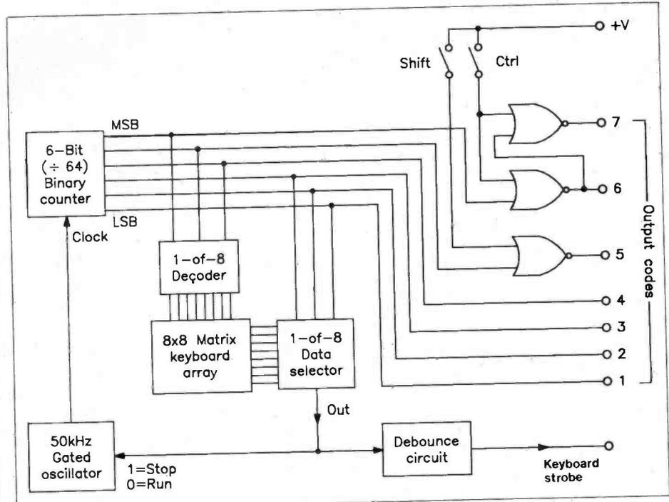
Figure 2. A scanned keyboard.
