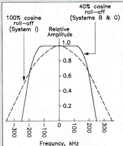
Figure 2. Spectrum shaping (due to combined transmit/receive data-shaping) for System I and Systems B and G.
