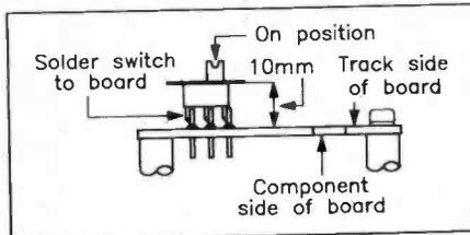
Figure 4. Mounting the Slide Switch.
