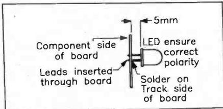
Figure 3. Mounting the LEDs.
