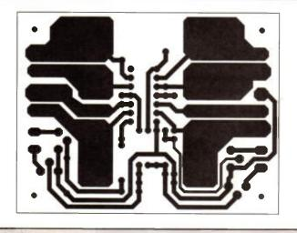
Figure 4. Car Lamp Monitor PCB legend and track.
