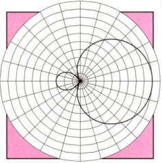
Figure 15a. Hypercardioid directional response of each capsule of the Soundfield microphone.
