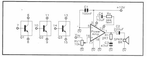
Figure 15. Basic circuit connections of the LM389 IC.
