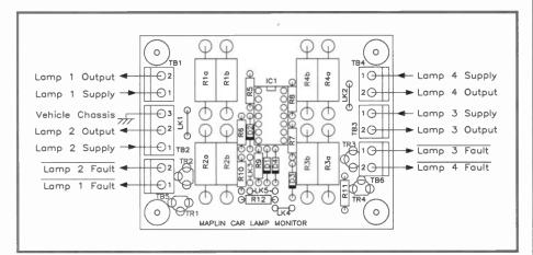
Figure 6. Car Lamp Monitor terminal functions.
