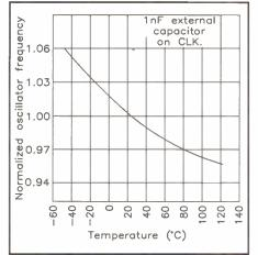
Figure 2(c). Internal oscillator frequency vs. temperature.
