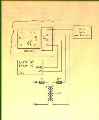
Figure 6a. Suitable interconnections to PSU and to door lock mechanism.
