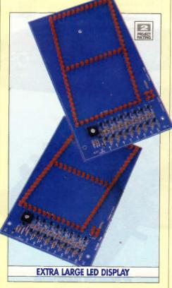
A choice of two 20cm (7 1/2in.) 7-segment LED displays, catering for open-collector and open-anode circuits. Ideal for educational equipment, public displays, exhibitions, demonstrations, clocks etc. Connects to existing 7-segment display drivers. Operating voltage: 22 to 26V DC, maximum supply current: 400mA. Order as: VF01B, Common Cathode Version, **Price £32.95**, or: VE63T, Common Anode Version, Price £32.95. Details in Electronics No. 74 (XA74R).
