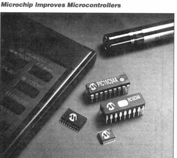
Microchip's PIC16C54 8-bit microcontroller is now available with reduced power consumption, improved electrical characteristics and denser packaging. Using an advanced 0.9-micron double-layer metal wafer fabrication process, the new one-time programmable PIC16C54A can be powered from a single lithium-ion battery making it an ideal solution for portable applications such as pagers and remote controls.
