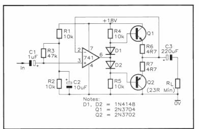
Figure 5. Op amp power amplifier using a single-ended supply.
