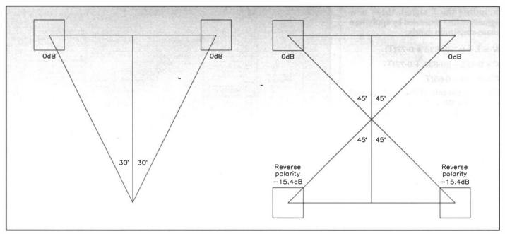
Figure 16. Optimum loudspeaker layouts for stereo and 2-channel Ambisonics.
