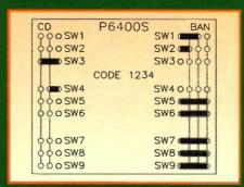
Figure 3. The wire links set up for code '1234'.
