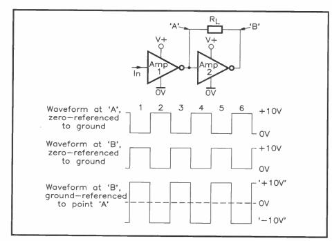
Figure 7. A pair of amplifiers connected in the 'bridge' mode give a peak output of  $2V^2 \div R$  watts, i.e. four times the power of a single-ended circuit.
