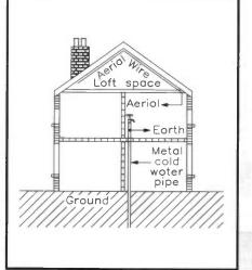
Figure 8c. Typical indoor loft aerial system.
