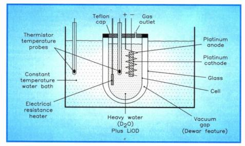
Figure 2. Schematic design of Fleischmann-Pons electrochemical cell used to demonstrate cold fusion.
