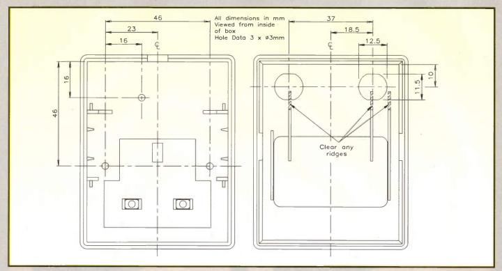
Figure 6b. PSU box drilling details.
