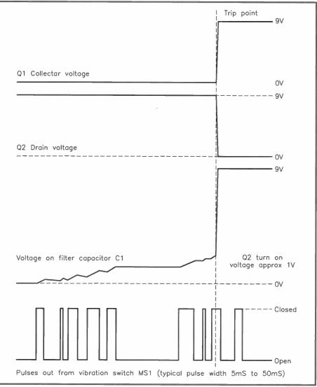
Figure 3. Movement detector, typical waveforms.
