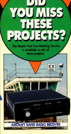
Listen in on pilot and control tower communications with this super AM airband receiver. The kit is simple to build and requires little alignment. Frequency range is 118 to 135MHz and the receiver operating voltage is 9V. (Optional case not included.) Order as: CP17T, **£29.95**. Details in *Electronics* No. 75 (XA75S).
