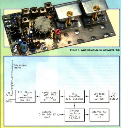
Figure 1. Block diagram of the Aerial Activator.
