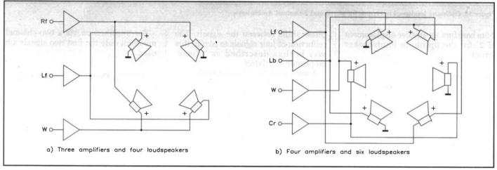
Figure 18. Arrangements of amplifiers and loudspeakers for Ambisonics.
