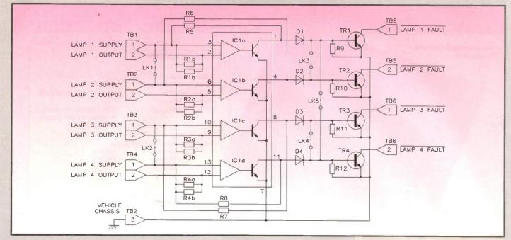
Figure 3. Circuit diagram of the Car Lamp Monitor.
