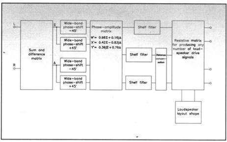
Figure 17b. Example of an Ambisonics decoder with 2-channel input.
