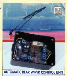
At last! Comprehensive control for rear window wipers, tied into the operation of the front windscreen wipers and gearbox. Facilities include: Single shot (when front wipers turned on), Intermittent operation (when front wipers on), and Auto wipe (Reverse gear selected and front wipers on).
