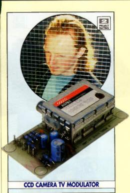
A low-cost unit which allows the Maplin colour and black & white CCD Camera Modules to be linked to any normal domestic TV with UHF aerial input. Applications include closed-circuit security systems, and interfacing equipment that only has video outputs to a normal TV receiver
