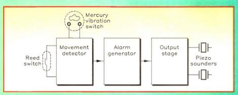
Figure 1. The ATD block diagram.
