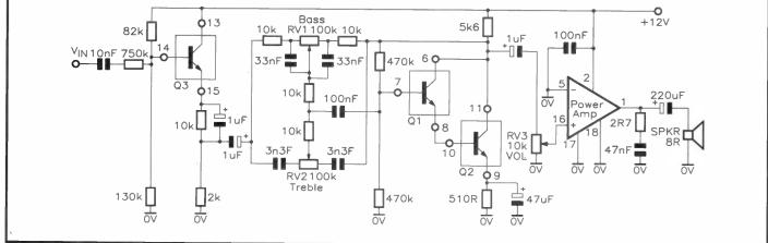
Figure 16. Ceramic phono amplifier, with tone controls, using an LM389.
