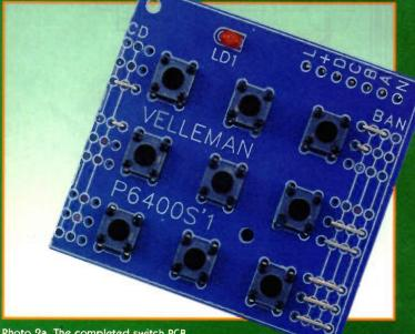
Photo 2a. The completed switch PCB.
