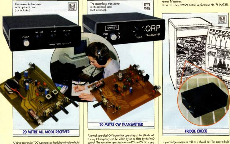
A 'direct conversion' 'DC' type receiver that is both simple-to-build and easy-to-use as there is no 'intermediate frequency' (IF). Frequency range is 13.85 to 14.50MHz and the receiver operates from a standard 9V PP3 battery (not supplied). Order as: CP13P, £31.95. Details in Electronics No. 76 (XA76H).
