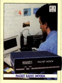
Combine your amateur radio and computing hobbies with this radio MODEM! The project is supplied with software compatible with the IBM PC/AT but could also be used with other computers provided suitable software can be obtained. The unit communicates via the host computer's RS232 port and operates at 1200 baud. Power consumption is very small and the unit can, in foct, be powered direct from the serial data port of most compatible computers!
