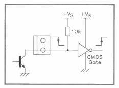
Figure 8. Interfacing the Car Lamp Monitor to CMOS logic.
