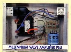
A Power Supply kit for the Millennium 20W Valve Power Amplifier. The supply is capable of powering up to two amplifier modules for a stereo system, or alternatively you could use two PSU kits and two amplifier modules to produce a pair of 'monobloc' amplifiers. Order as: LT44X, Price £49.95 C6. Details in Electronics No. 73 (XA73Q)
