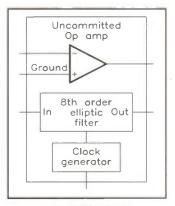
Figure 1(b). MAX293/297 internal diagram. An internal block diagram of the MAX293 or 297 IC is given in Figure 1b. The absolute maximum ratings and electrical characteristics of the IC are detailed in Tables 1a and 1b. Note: Do not exceed these absolute maximum ratings.
