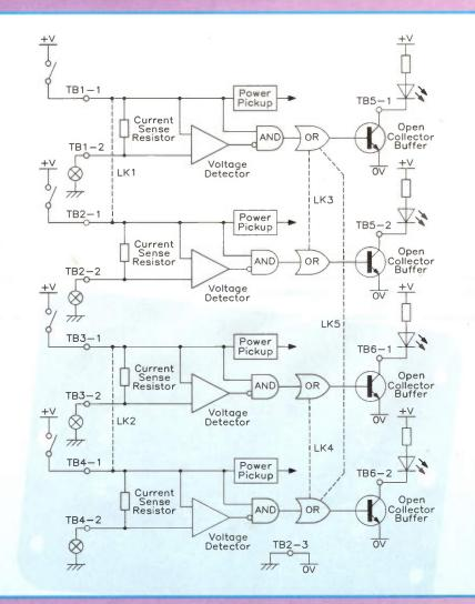
Figure Z. Block diagram of the Car Lamp Monitor.
