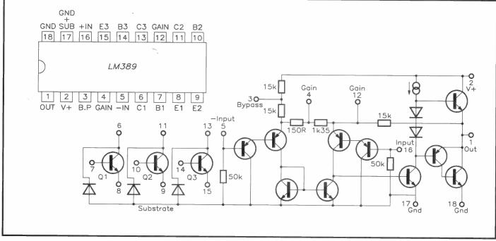
Figure 14. Circuit and outline of the LM389 low-voltage audio power amplifier with npn transistor array.
