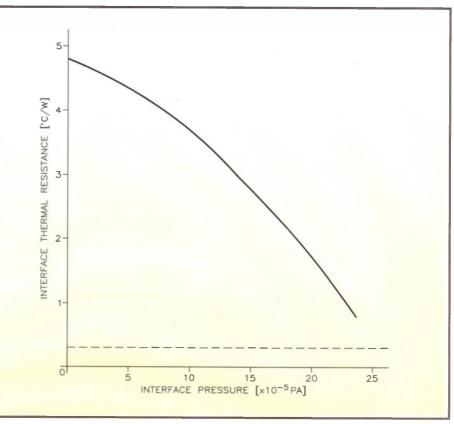
Figure 5. The effects of pressure and heat transfer grease on thermal resistance, when applied to the Interface between a power device and heatsink.
