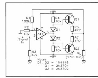
Figure 4. Op amp power amplifier using dual supplies
