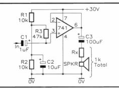
Figure 2. Low-power amplifier using a single-ended power supply.
