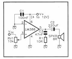
Figure 9. Minimum-parts LM386 amplifier with AV = 20.
