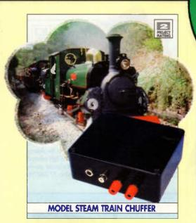
Add the extra dimension of sound to your layout with this realistic steam engine sound simulator. The rate of chuffing varies with the track voltage, i.e. train speed, and when the engine is stationary the sound of escaping steam can be heard. The unit requires a supply of +15.5 to 36V DC and the audio output connects to your existing amplifier. (Optional case not included.) Order as: LT39N, £9.99. Details in *Electronics* No. 79 (XA79L).
