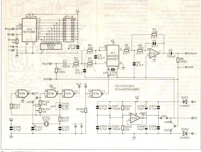
Figure 8. MAX293/297 circuit diagram.
