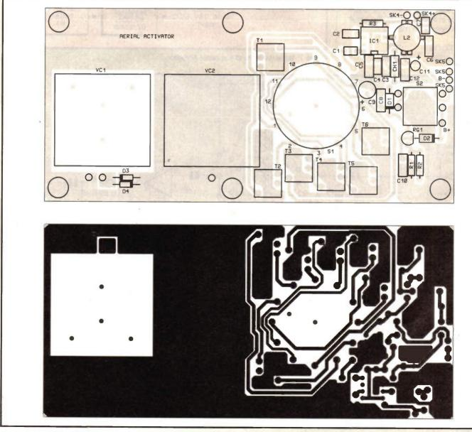
Figure 3. PCB legend and track (please note that this design employs a double-sided PCB with component side ground plane,
