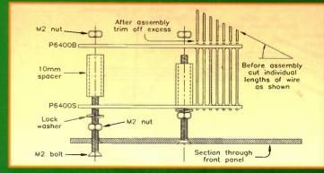
Figure 4. The exploded assembly including the fitting and cutting of the seven interconnecting wires.
