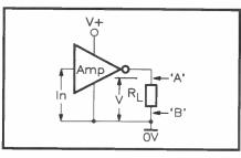
Figure 6. An amplifier connected in the 'single ended output' mode gives a peak output of  $V^{*}$  + R watts.
