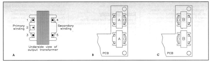
Figure 9. (a) Underside view of output transformer. (b) Type A orientation. (c) Type B orientation.
