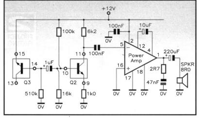
Figure 17. LM389 white-noise sound generator.
