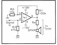
Figure 1. Low-power amplifier using dual power supplies
