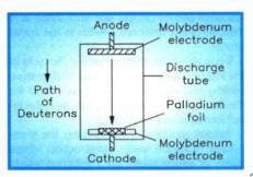
Figure 3. Glow discharge system of cold fusion. Excess powers of at least 300% have reported using this technique.
