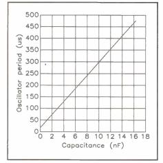
Figure 2(a). Internal oscillator period vs. capacitance value.
