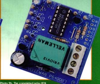
Photo 2b. The completed relay PCB.
