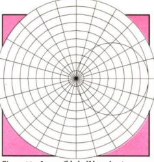
Figure 12a. Impossible half-lemniscate directional response required for correct capture of '4-channel stereo'.
