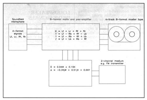
Figure 17a. Example of Ambisonics encoding.
