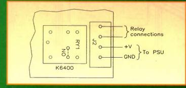
Figure 5. External connections to the terminal block on the PCB. August 1994 Maplin Magazine
