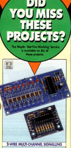
How da you get up to 16 channels and a power supply down two wires? This clever project scans the transmitter inputs and converts them to serial data pulses superimposed on the DC power supply. The data is then decoded by the receiver and operates the rel evant channel. Each transmitter and receiver pair can handle 8 channels, expandable to 16 by adding further modules. Order as: VE70M, Transmitter, £9.95. Order as: VE71N, Receiver, £17.95. Details in Electronics No. 77 (XA77H).
