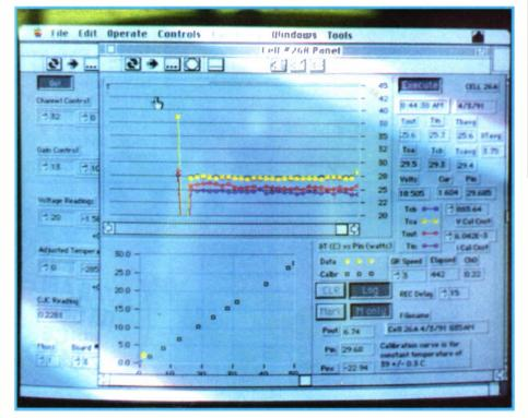
A close up of computer monitor showing the virtual instrument stored in computer memory and used for cell data acquisition and cell monitoring.
