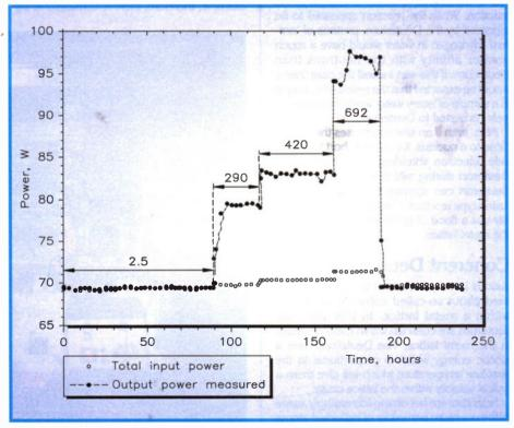
Figure 5. Variation with time of output/input power of a molten salt electrochemical cell. Numbers in the figure are the current densities in mA/cm<sup>2</sup> at which Deuterium was charged into the Palladium electrode.
