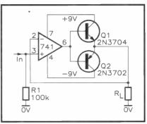
Figure 3. Basic 'boosted output current' unity-voltage-gain op amp circuit.
