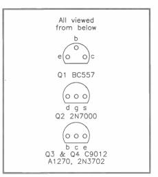
Figure 5. Transistor bases.
