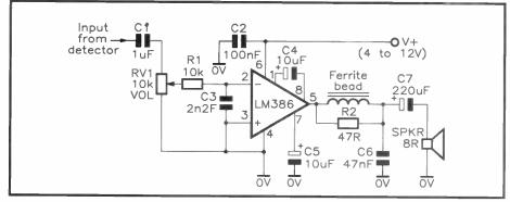
Figure 13. AM-radio power amplifier.
