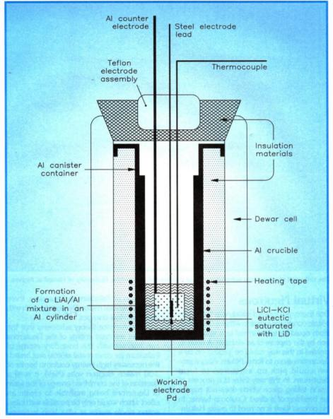
Figure 4. Molten salt 'cold fusion' cell developed by the University of Hawaii. The unit operates at temperatures between 350°C and 500°C.
