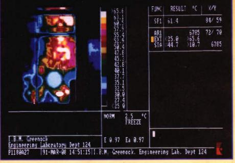
Photo 1. The thermal image of a PCB taken using a Thermovision 800 infra-red camera.
