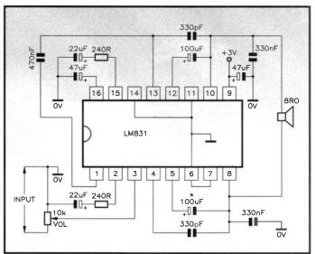
Figure 20. Bridge-connected LM831 amplifier.
