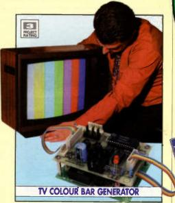
Essential for accurately setting up TV and video equipment. The generator consists of two modules, a colour bar generator and a colour encoder. Although the modules are available separately, both are required for this project. The generator has both PAL compasite video and PAL UHF RF outputs and can produce EBU, 100% and 75% colour bars.
