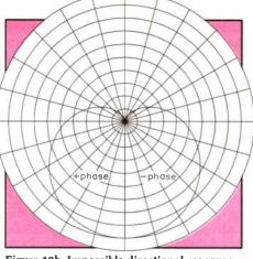
Figure 12b. Impossible directional response required for correct capture of rearward sound in a two-channel system.
