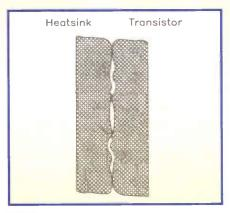
Figure 4. Typical microscopic appearance of the contact interface between a power device and a heatsink.
