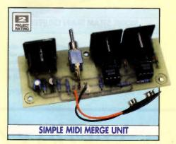
This easy-to-build project allows you to control a single MIDI sound module from two different sources. Apart from simultaneous operation from two MIDI sources, this simple unit can perform all the tasks normally undertaken by complex microprocessor controlled units costing many times more
