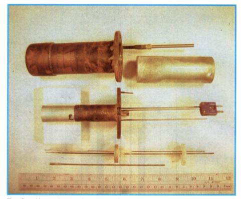
The cell used in a previous experiment using molten salt electrolyte. University of Hawaii at Manoa.
