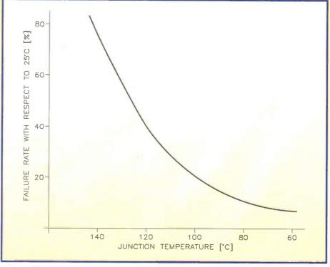
Figure 1. Failure rate of a semiconductor junction. versus temperature.
