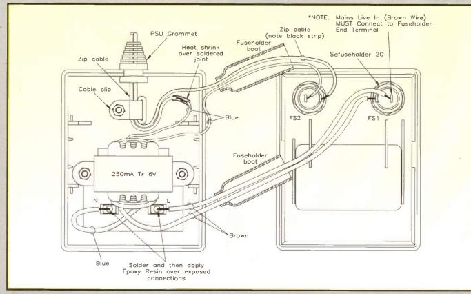
Figure 6c. PSU assembly details.
