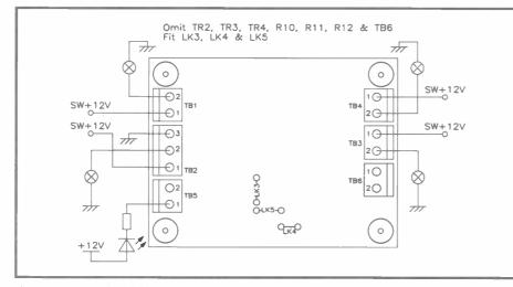
Figure 7c. Shared fault indicator LED for all lamps.
