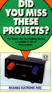
Help eliminate the hazards of accidental short-circuits during your experimental and development work with this simple-to-build project. The unit is connected in series with the unit being tested, and if the current drawn exceeds 200mA the electronic fuse will emit a short bleep and the LED will flash continuously. The current then falls to a very low holding level until the fault has been corrected. (Optional case not included.) Order as: LT70M, £12.99. Details in Electronics No. 79 (XA79L).
