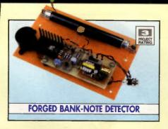
Sort out fake bank-notes with this notable Maplin project! Unlike counterfeit notes, the genuine article absorbs ultra-violet light from the built-in UV tube. A light dependent resistor in the detector changes its resistance depending on the amount of light reflected. If the note is genuine, an LED indicator lights and a buzzer sounds. Order as: LT54J, £14.99. Details in Electronics No. 77 (XA77H).
