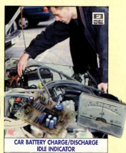
Is your car's battery being charged as you drive, or is it wait ing for the next cold, rainy morning for you to find out that it isn't? Keep an accurate eye on where the current is going with this inexpensive project. A 3-colour LED, mounted on the dashboard, indicates whether the battery is being charged, discharged or if a balanced condition is achieved. Order as: LT56L, £7.99. Details in *Electronics* No. 78 (XA78K).
