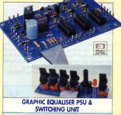
Part of the Modular Graphic Equaliser System. This project provides a regulated power supply for various of the other units in the system, a front panel mounted line input sensitivity control and also provides all of the necessary switching functions. Order as: VE45Y, Price £32.95. Details in Electronics No. 73 (XA73Q).
