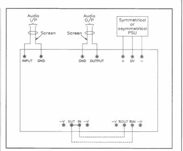
Figure 10. PCB connection diagram.
