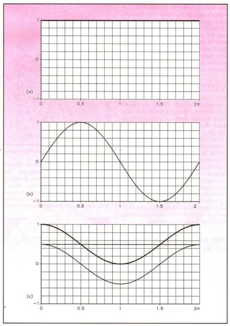
Figure 13. Directional responses plotted on Cartesian co-ordinates. (a) Omnidirectional: zero order harmonic. (b) Lemniscate: first order harmonic. (c) Cardioid and its two harmonic components.
