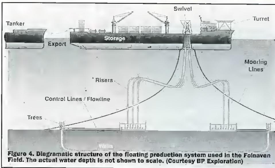
Figure 4. Diagrammatic structure of the floating production system used in the Foinaven Field. The actual water depth is not shown to scale. (Courtesy BP Exploration)
