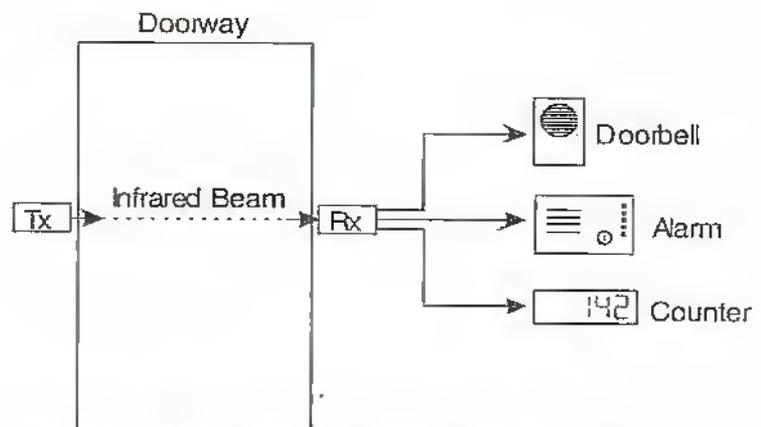
**Figure 4. Typical arrangement and possible applications for beam break detector.**
