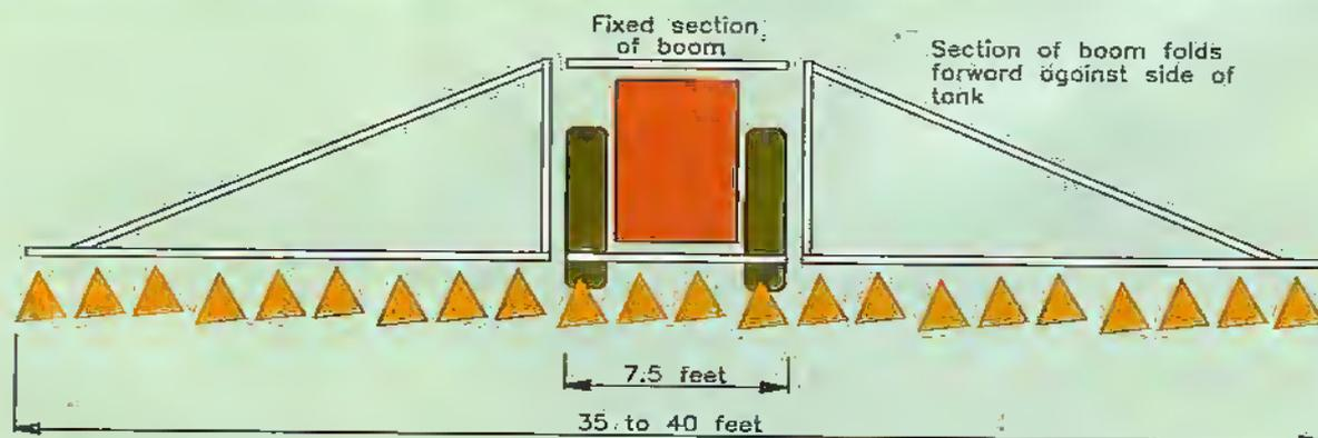
**Figure 3.** Simplified sketch of a 'bean' sprayer with orchard spray gear replaced by a crop sprayer boom. When turning on headlands, spray was stopped by driver disengaging the tractor PTO shaft. High pressure was required to cause nozzles to produce fine spray droplets and this caused problems with spray drift.
