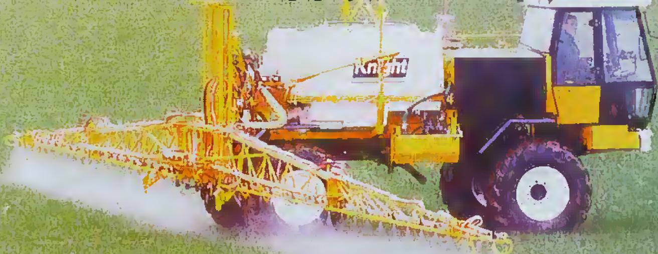
Photo 1A. A modern self-propelled, computer-managed, crop sprayer. Note that cab is supplied with filtered air. (Courtesy of Knight Farm Machinery Ltd.)
