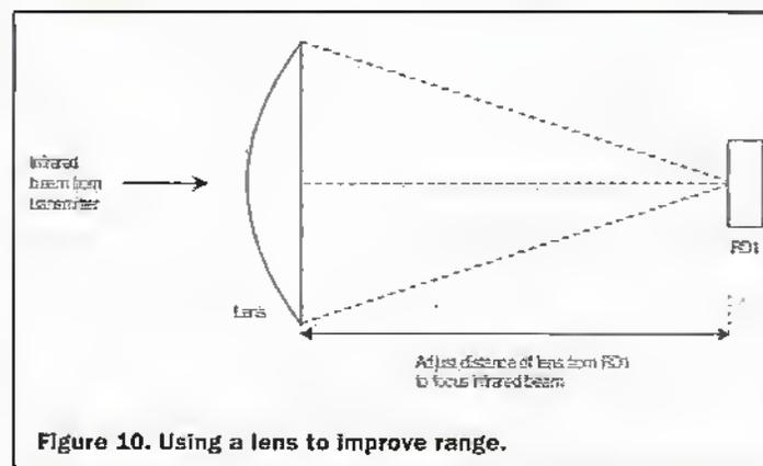
Figure 10. Using a lens to improve range.
