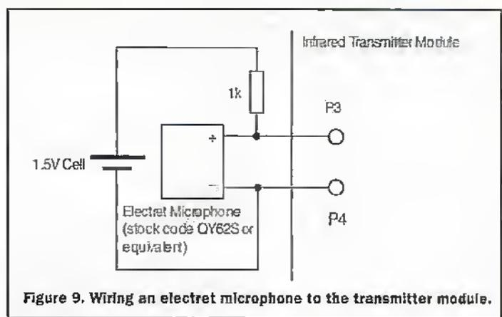
Figure 9. Wiring an electret microphone to the transmitter module.
