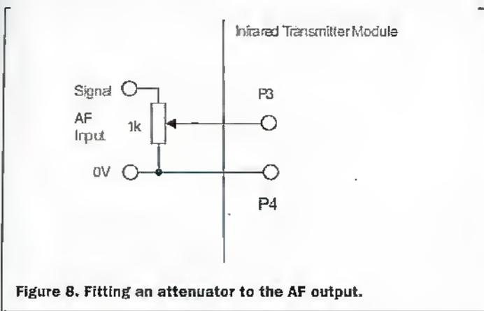
Figure 8. Fitting an attenuator to the AF output.
