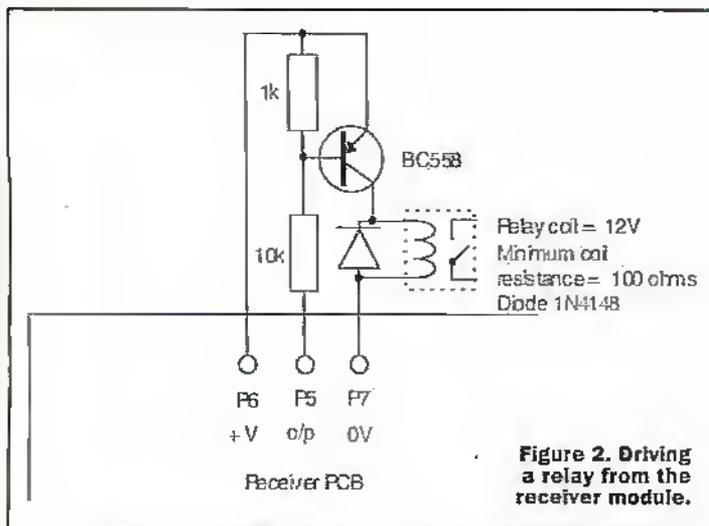
**Figure 2. Driving a relay from the receiver module.**
