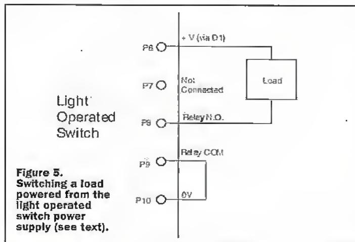
Figure 5. Switching a load powered from the light operated switch power supply (see text).
