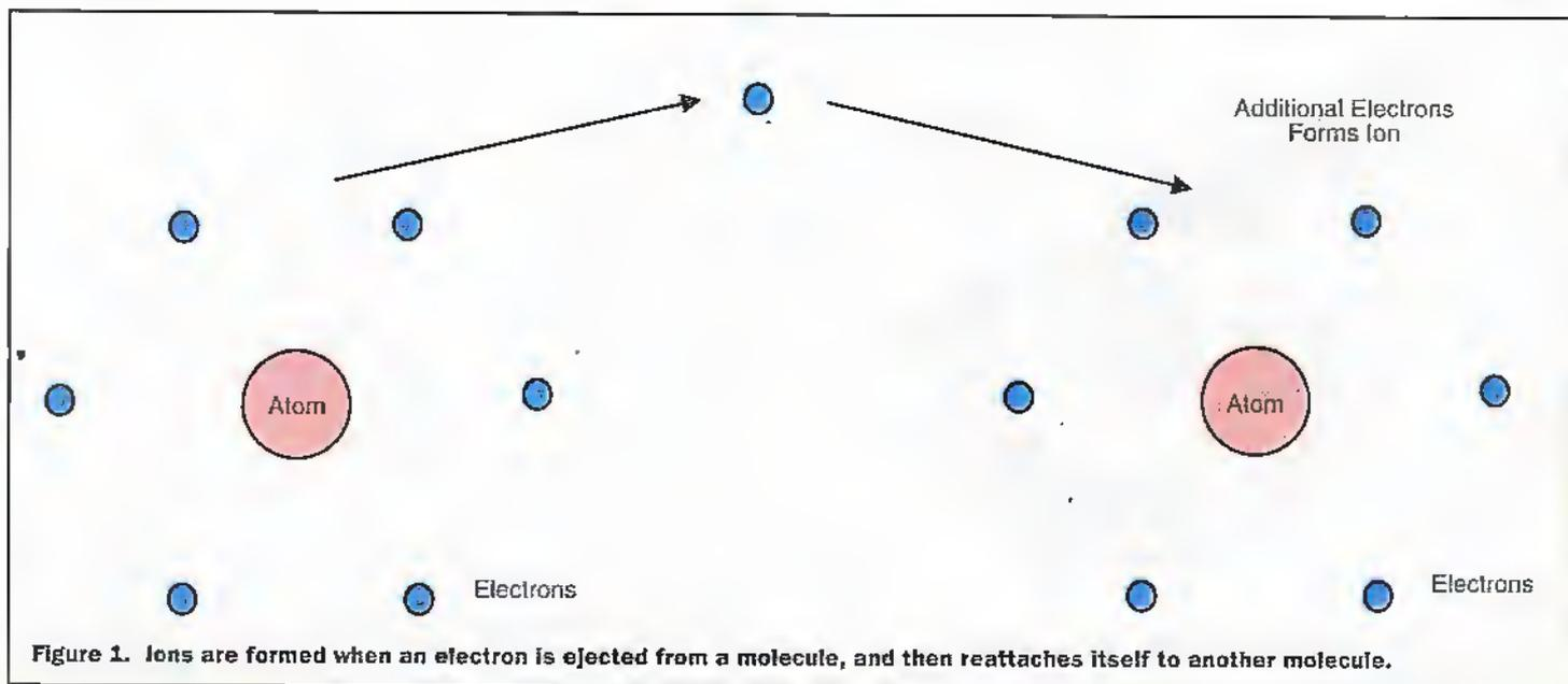
Figure 1. Ions are formed when an electron is ejected from a molecule, and then reattaches itself to another molecule.
