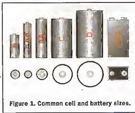
Figure 1. Common cell and battery sizes.
