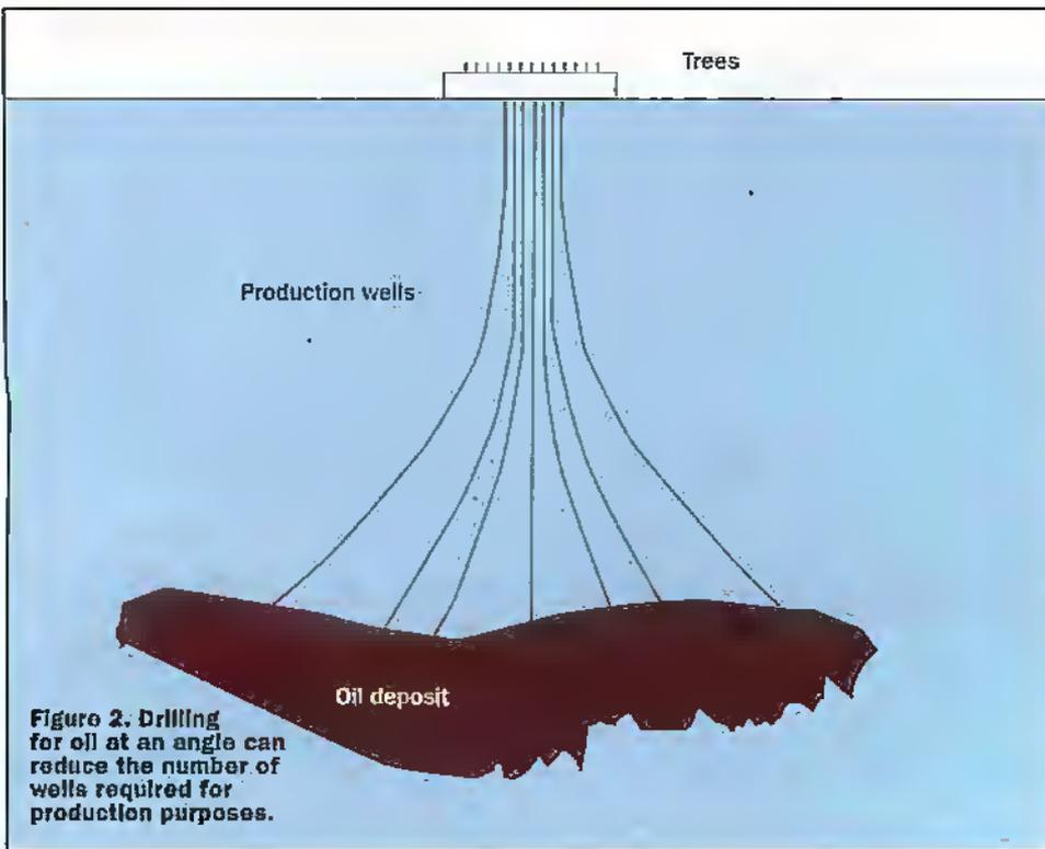
**Figure 2.** Drilling for oil at an angle can reduce the number of wells required for production purposes.
