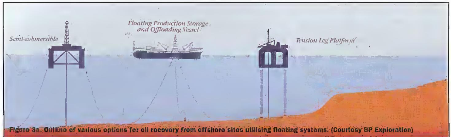
**Figure 3a.** Outline of various options for oil recovery from offshore sites utilising floating systems. (Courtesy BP Exploration)
