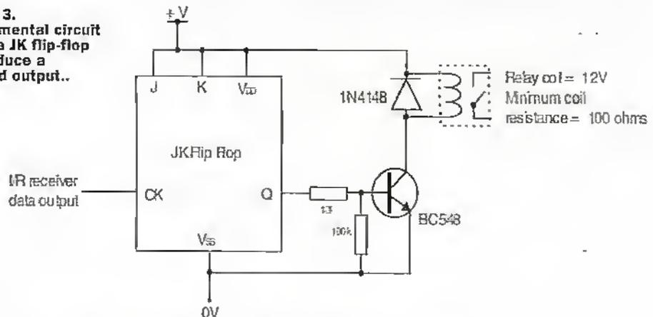
JK Flipflop must be capable of operating from 12V supply (CMOS 4027 or similar). Set and reset pins should be tied low where applicable.
