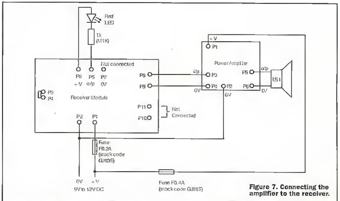
Figure 7. Connecting the amplifier to the receiver.
