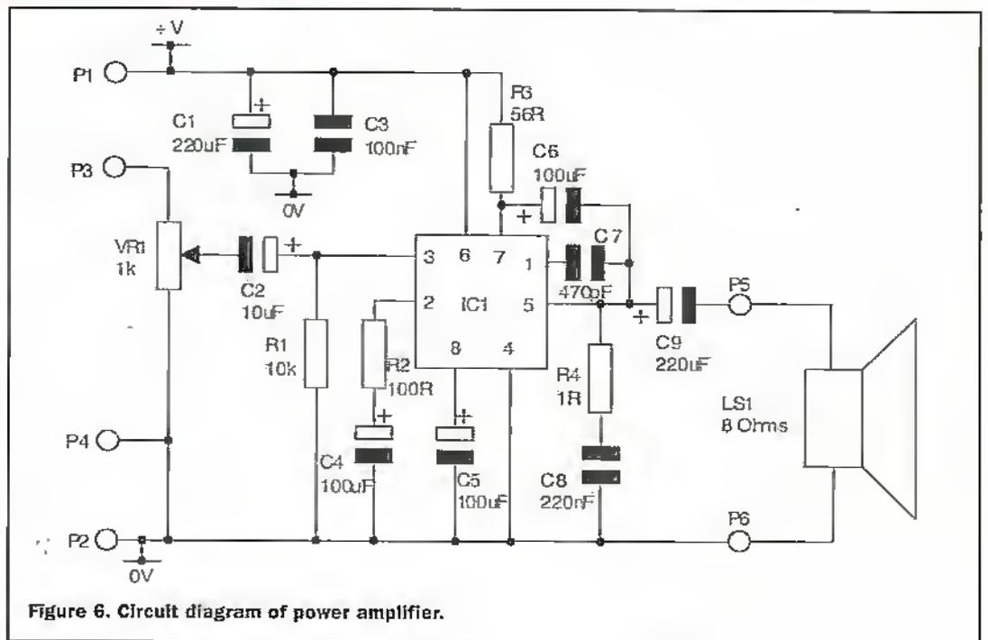
Figure 6. Circuit diagram of power amplifier.
