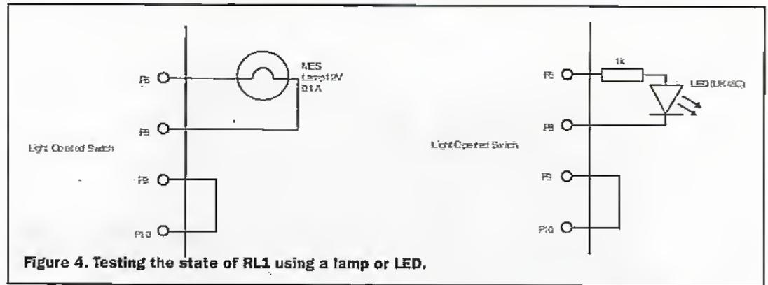
Figure 4. Testing the state of RL1 using a lamp or LED.
