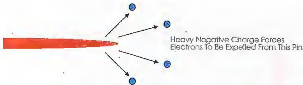
Figure 3. Electrostatics theory dictates that a pin is the best vehicle to expel negative ions into the atmosphere.
