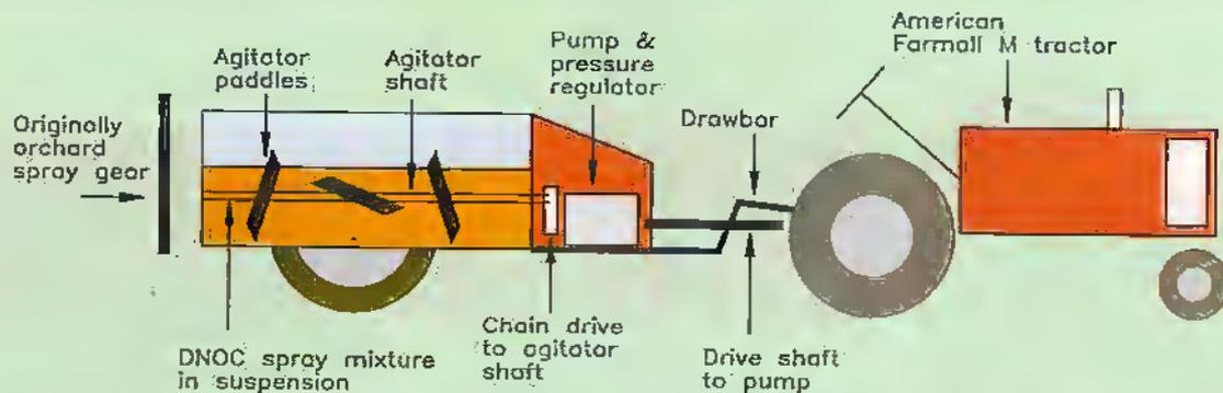
**Figure 2.** Simplified sketch of a 'bean' spraying machine. 1944. Only imported Farmall tractors had sufficient power to tow the sprayer and drive the pump.
