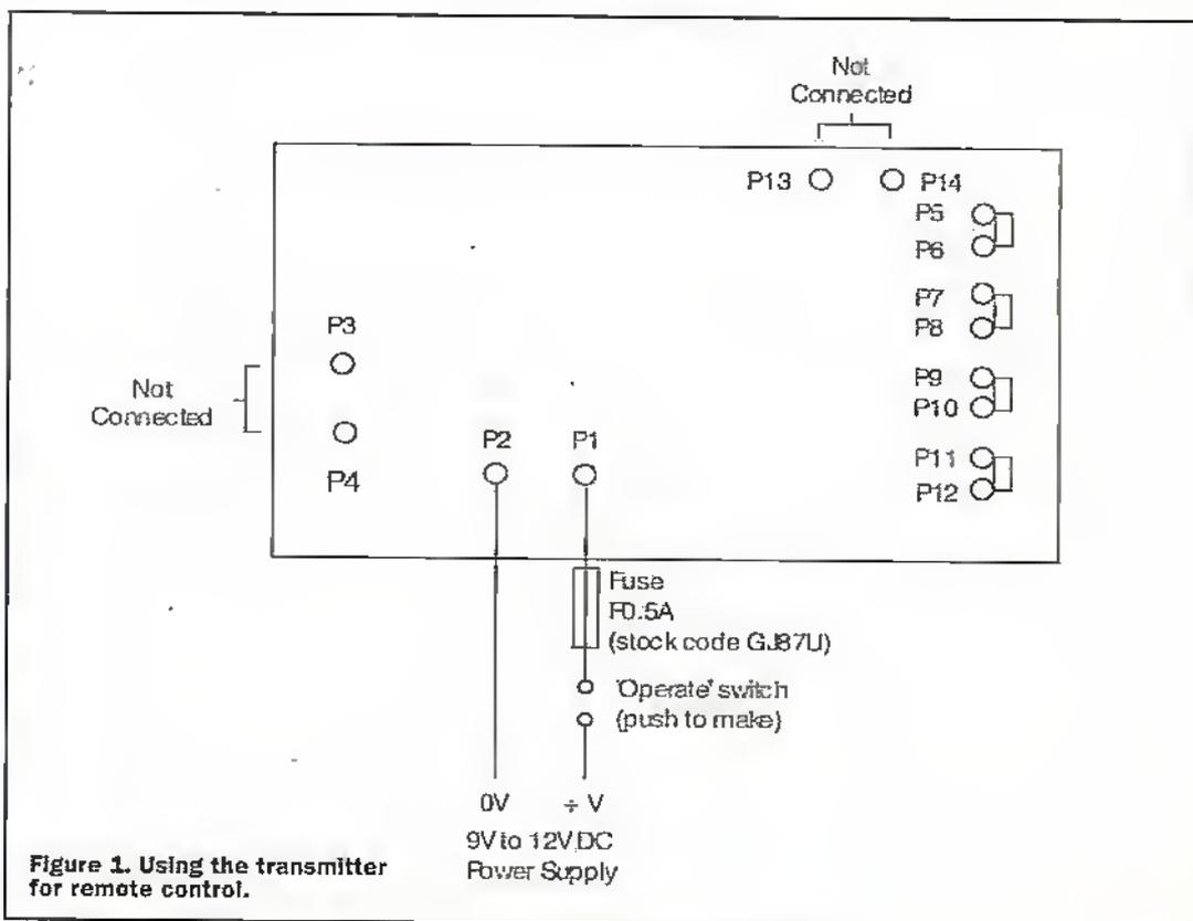
Figure 1. Using the transmitter for remote control.
