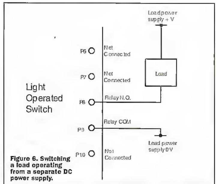
Figure 6. Switching a load operating from a separate DC power supply.
