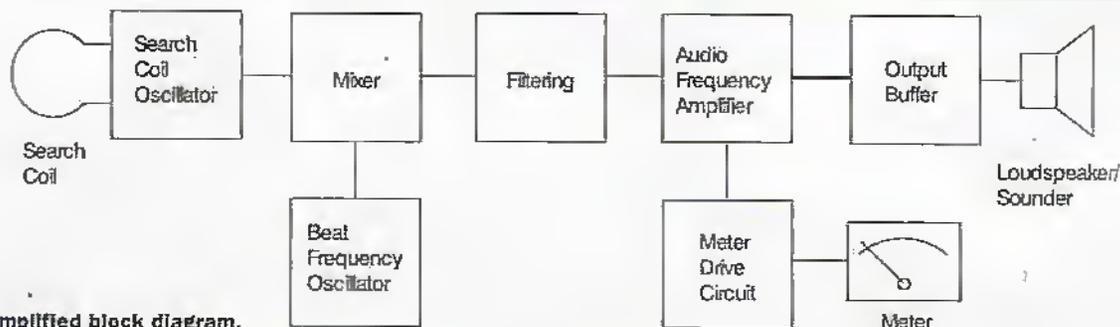
Figure 1. Simplified block diagram.
