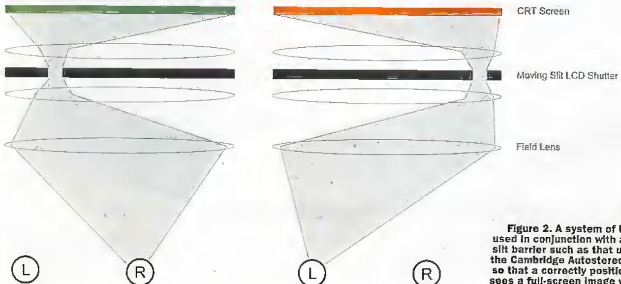
Figure 2. A system of lenses is used in conjunction with a moving slit barrier such as that used with the Cambridge Autostereo Display so that a correctly positioned eye sees a full-screen image when the appropriate slit is open.
