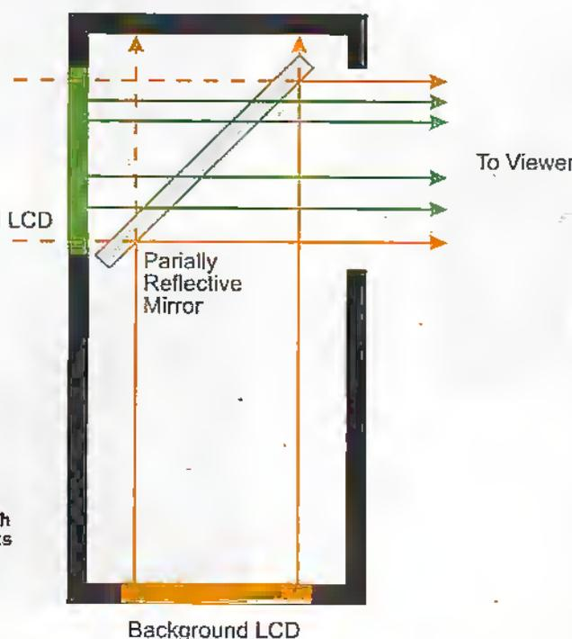
**Figure 5.** In the Real-Depth display, foreground objects and the background are displayed on different LCDs. Optics makes the background image seem further away.
