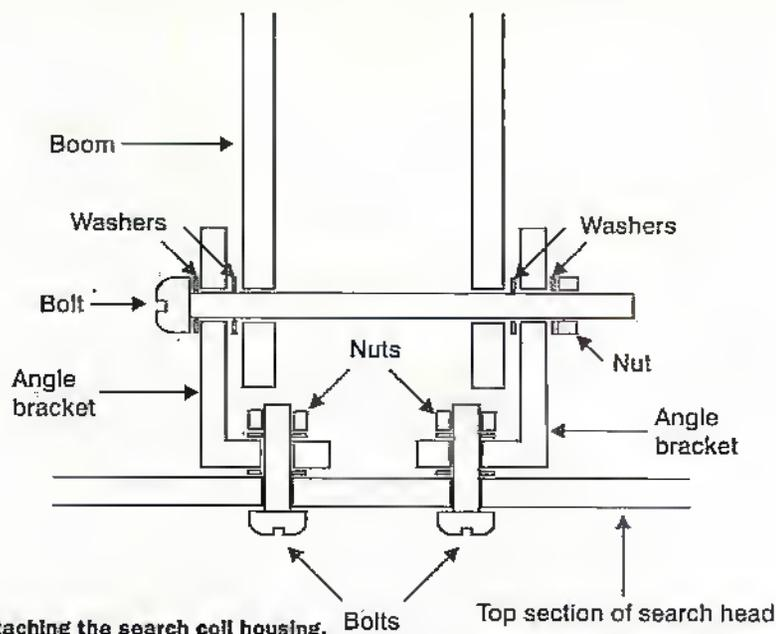
Figure 12. Attaching the search coil housing.
