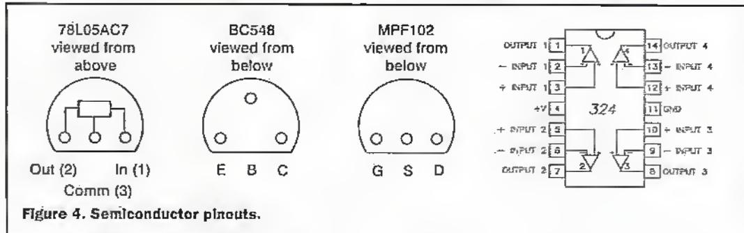
Figure 4. Semiconductor pinouts.
