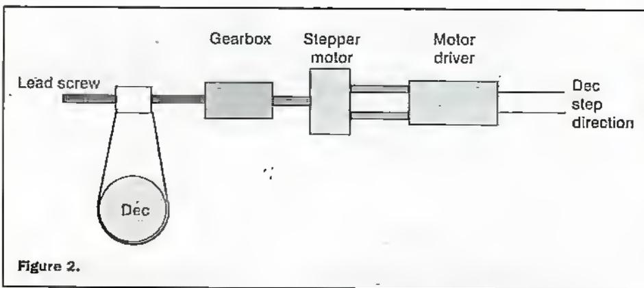
For the RA drive the mechanics consist of a stepper motor driving, via a gearbox and worm the main shaft. Bottom right in the main photograph and in detail in the Photo 3.
