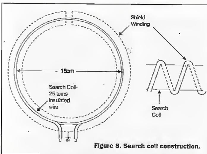
Figure 8. Search coil construction.
