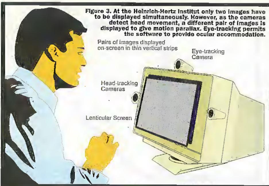
800Hz or one picture every 1.25ms. In fact, a CRT with this sort of refresh rate is one of the more demanding elements of this display method. Not only is ultra-fast electronics required - almost an order of magnitude faster than run-of-the-mill displays - but the phosphor must be ultra bright and have a very fast decay time.
