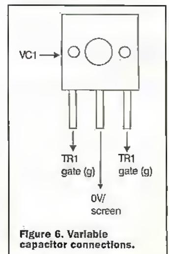
Figure 6. Variable capacitor connections.
