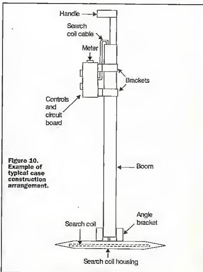
Figure 10. Example of typical case construction arrangement.
