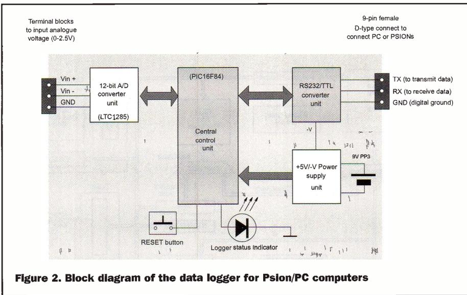
**Figure 2. Block diagram of the data logger for Psion/PC computers**
