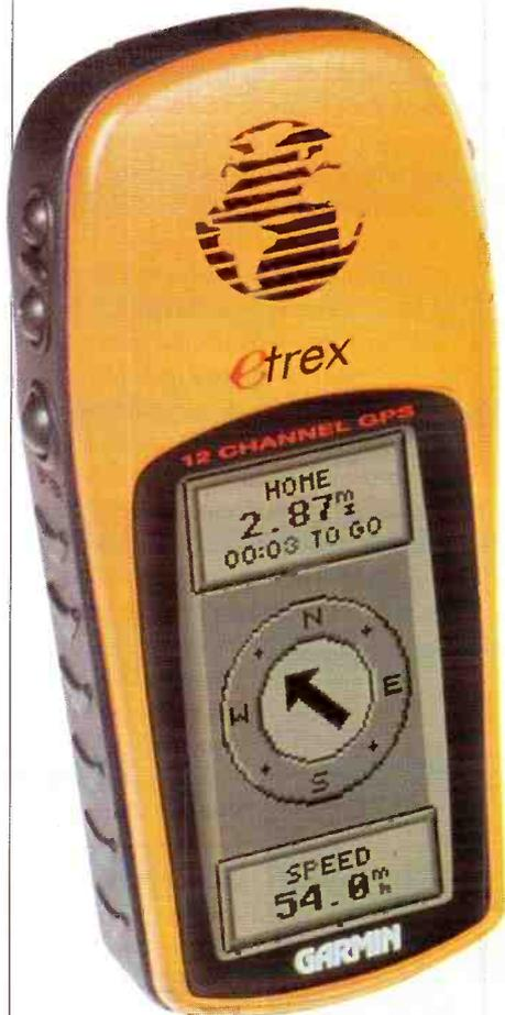
**The Garmin eTrex GPS receiver. This is waterproof to IP67 and it floats.**
