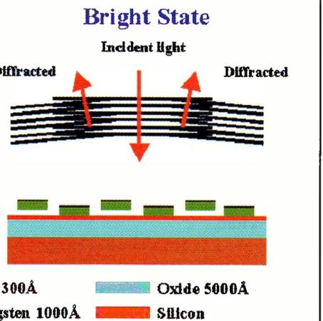
the ability to modulate, over a wide range, the time ratio of up-to-down states, which produces the effect of shades of grey or colour variations. GLV switching speeds make it easy to implement an 8-bit or greater grey scale, and are fast enough to support colours and greys over a 1000:1 dynamic range.
