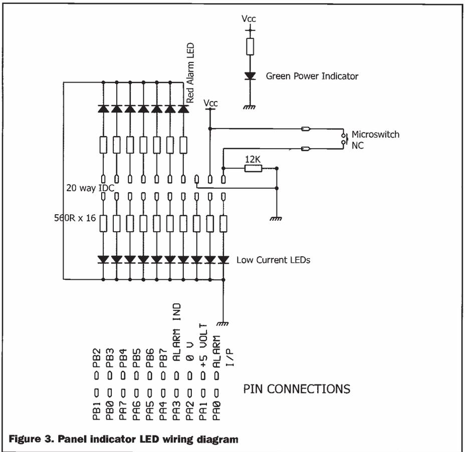
**Figure 3. Panel indicator LED wiring diagram**
