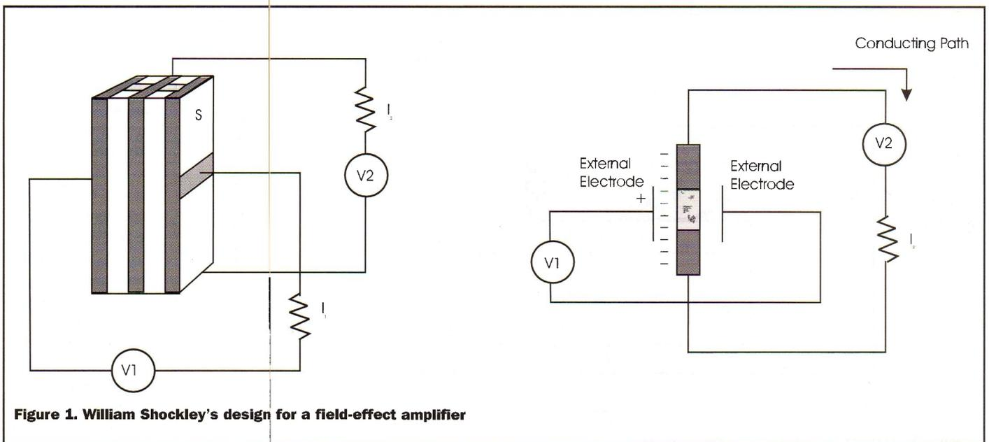
Figure 1. William Shockley's design for a field-effect amplifier
