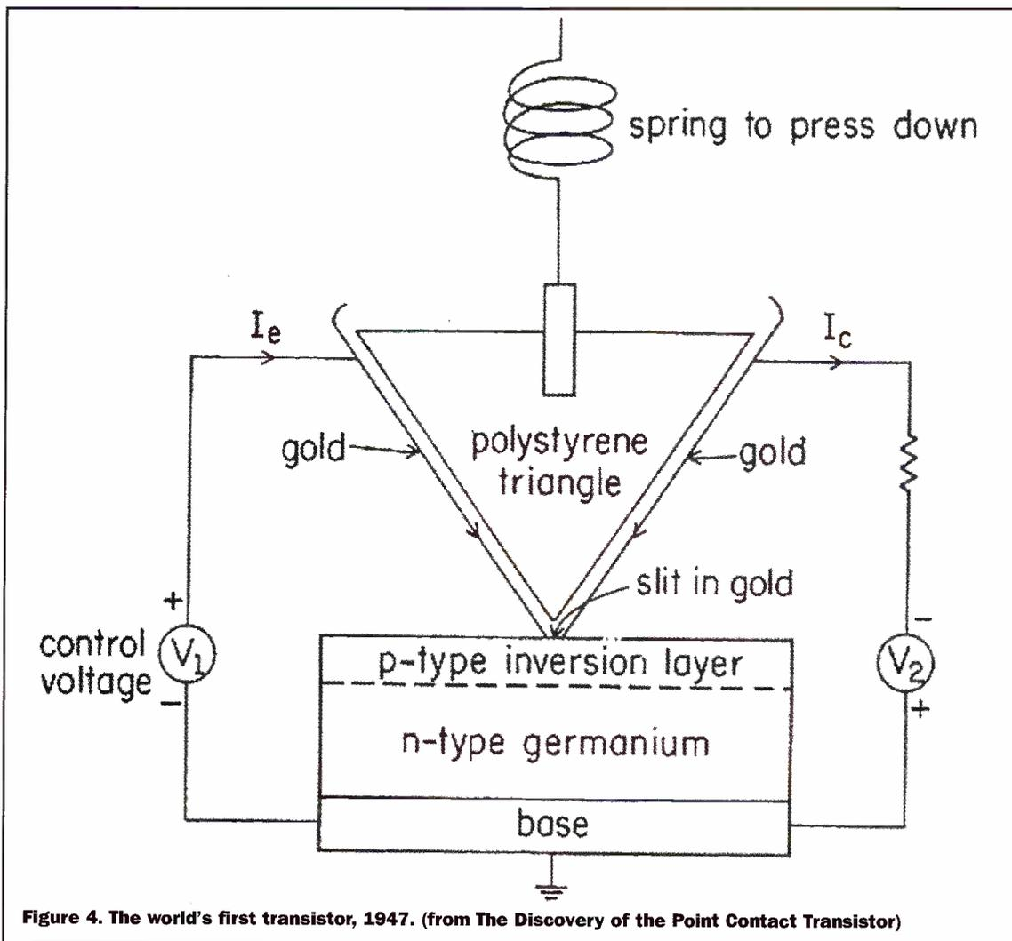
Figure 4. The world's first transistor, 1947. (from The Discovery of the Point Contact Transistor)
