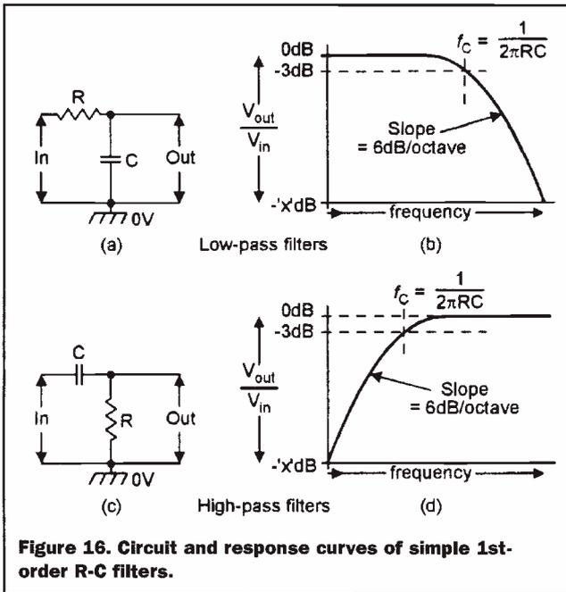
**Figure 16. Circuit and response curves of simple 1st-order R-C filters.**
