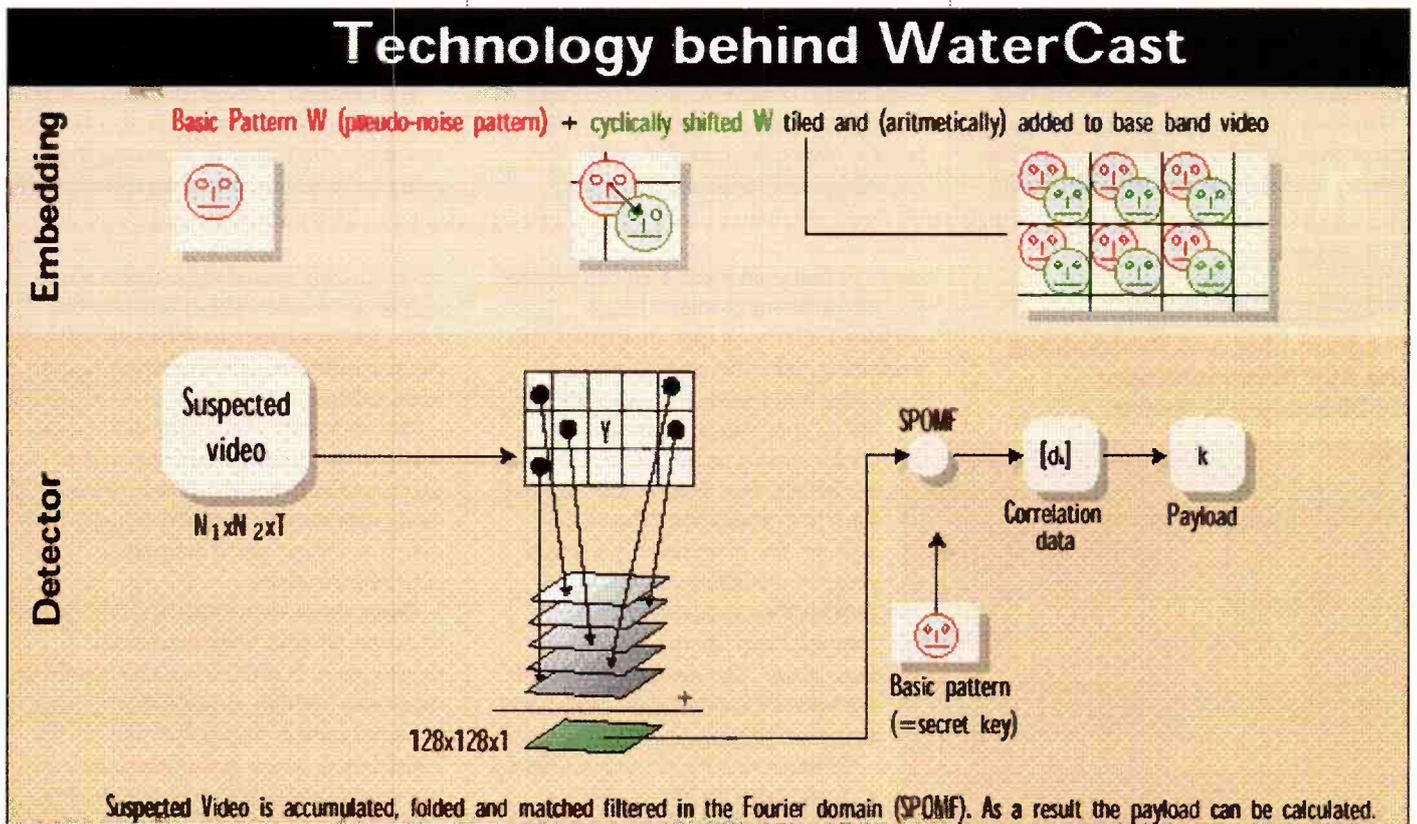
**Figure 3. Philips Watercast embedding and detecting.** Picture Philips Broadcast
