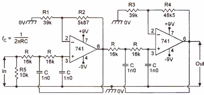
Figure 19. 4th-order 10kHz low-pass filter.
