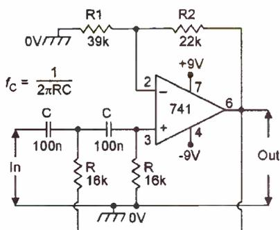
Figure 21. 'Equal components' version of 2nd-order 100Hz high-pass filter.
