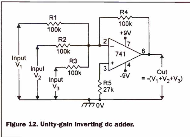
**Figure 12. Unity-gain inverting dc adder.**
