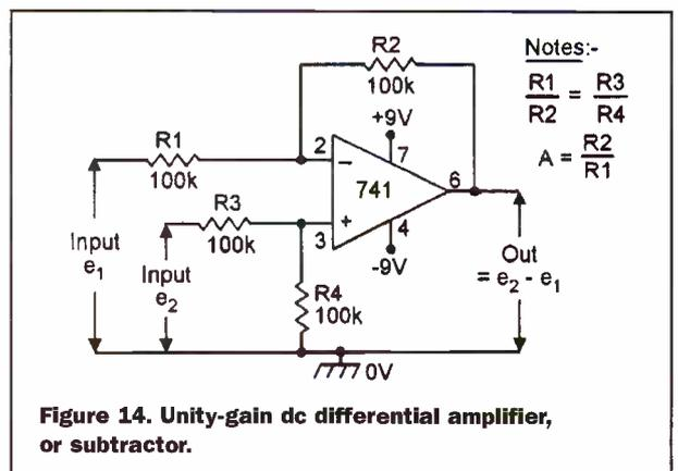
**Figure 14. Unity-gain dc differential amplifier, or subtractor.**
