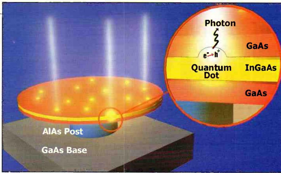
**Figure 2. A quantum dot single-photon turnstile device prepares the way for quantum cryptography**
