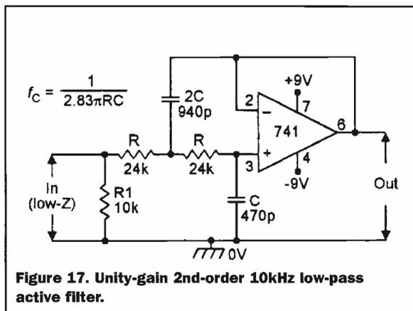
**Figure 17. Unity-gain 2nd-order 10kHz low-pass active filter.**
