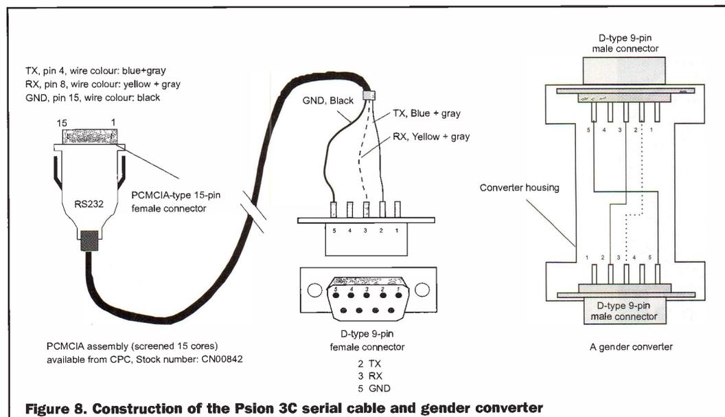
**Figure 8. Construction of the Psion 3C serial cable and gender converter**
