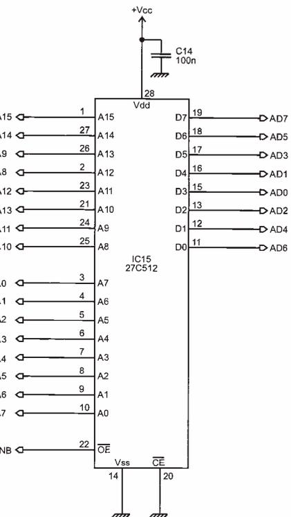
**Figure 6. EPROM connections. Note the mismatch between device pin functions and the connections to the microcontroller. See text for explanation.**
