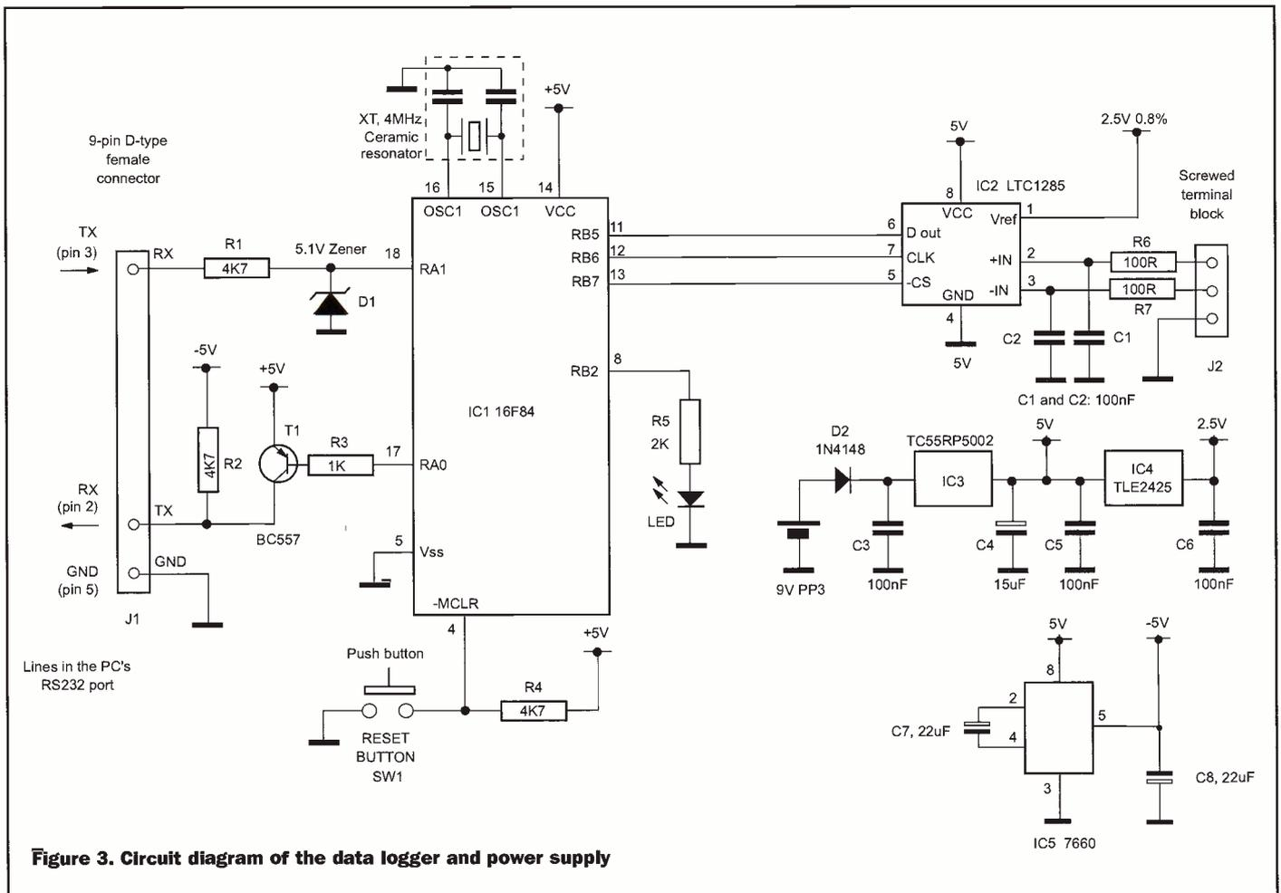
**Figure 3. Circuit diagram of the data logger and power supply**
