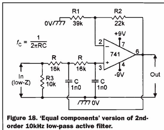
**Figure 18. 'Equal components' version of 2nd-order 10kHz low-pass active filter.**
