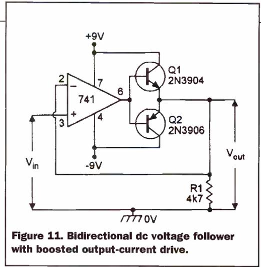
**Figure 11. Bidirectional dc voltage follower with boosted output-current drive.**
