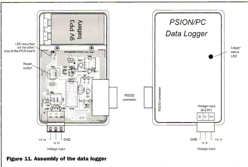
Figure 11. Assembly of the data logger
