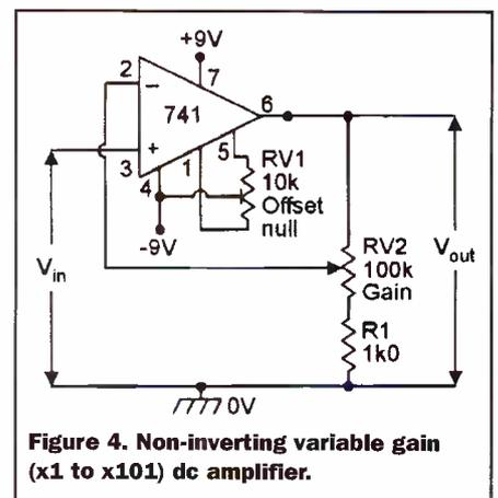
Figure 4. Non-inverting variable gain (x1 to x101) dc amplifier.
