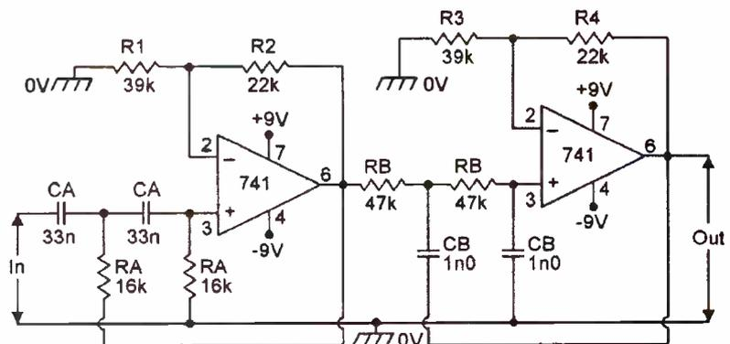
Figure 23. 300Hz to 3.4kHz speech filter with 2nd-order response.
