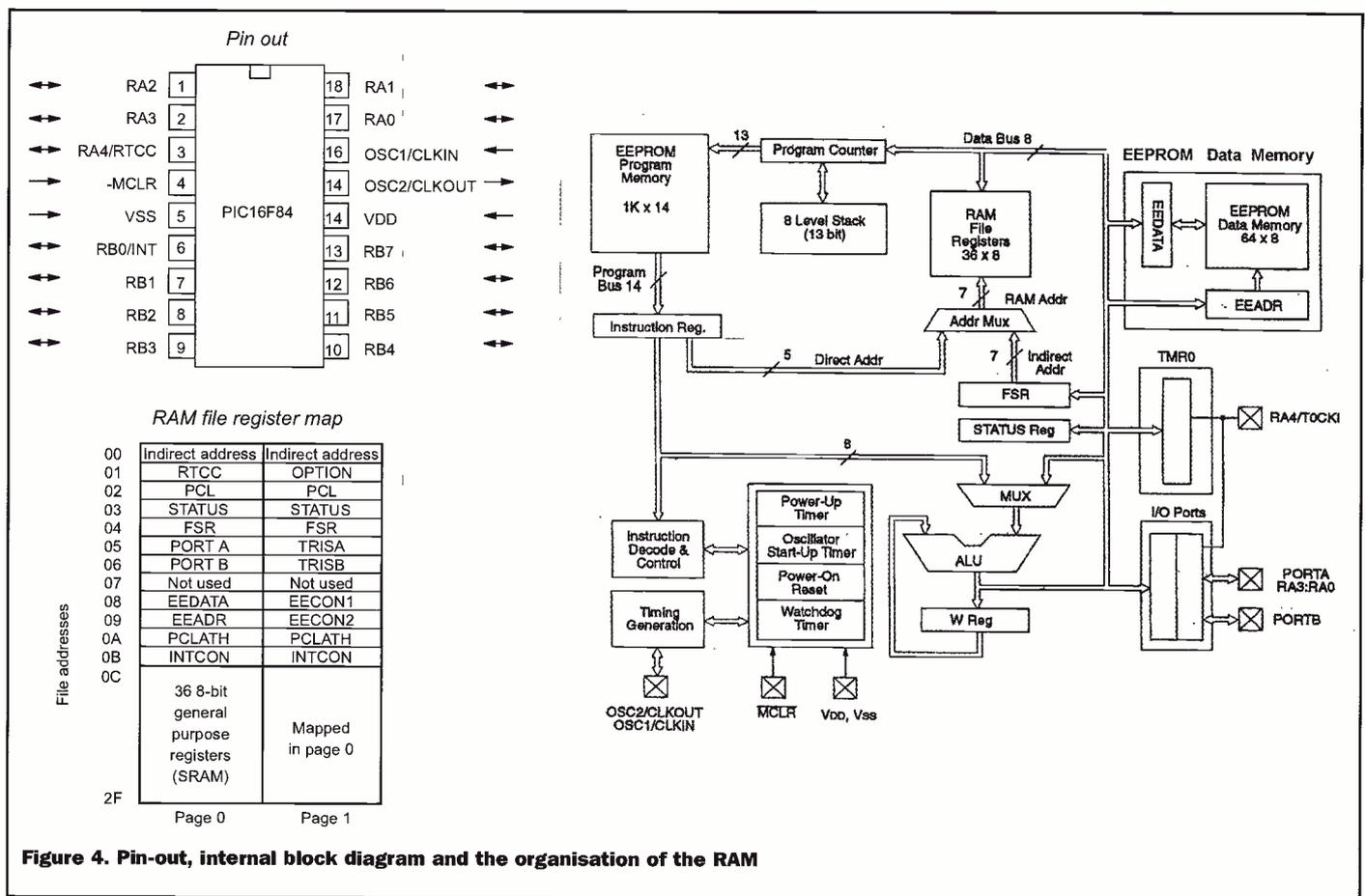
Figure 4. Pin-out, internal block diagram and the organisation of the RAM
