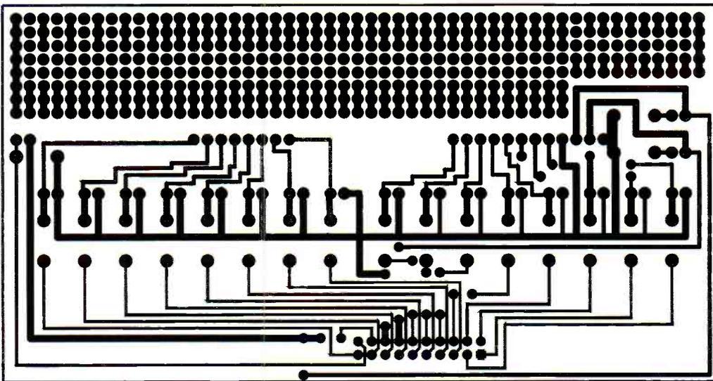
Figure 5. LED PCB bottom side
