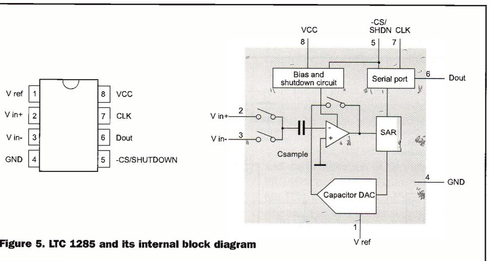
Figure 5. LTC 1285 and its internal block diagram
