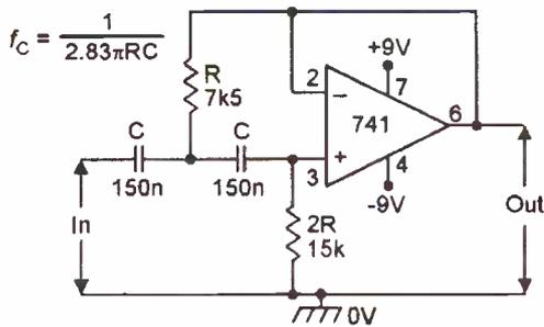
Figure 20. Unity-gain 2nd-order 100Hz high-pass filter.
