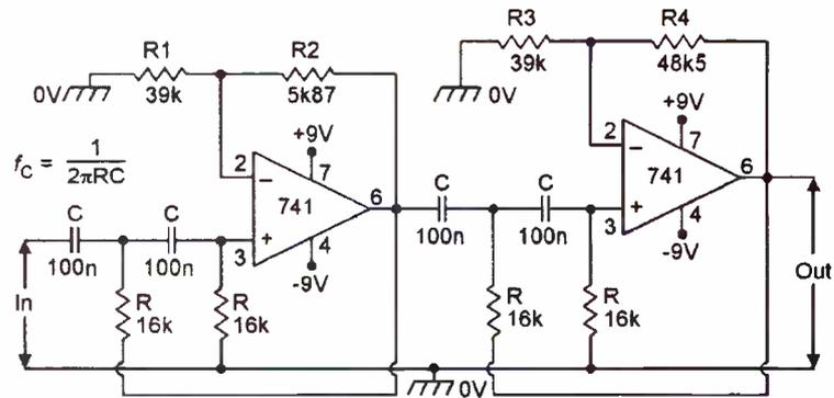
Figure 22. 4th-order 100Hz high-pass filter.
