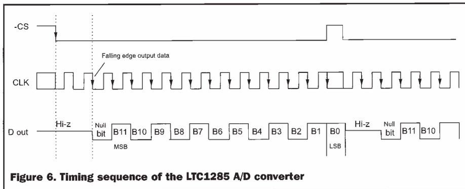
**Figure 6. Timing sequence of the LTC1285 A/D converter**
