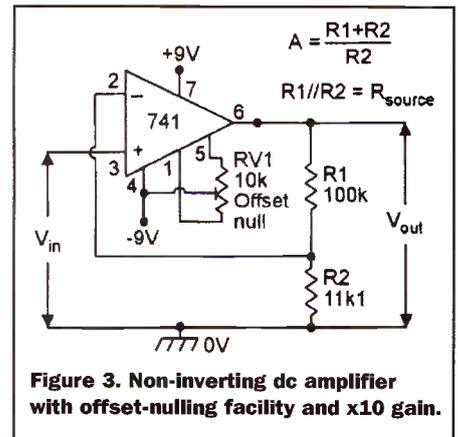
Figure 3. Non-inverting dc amplifier with offset-nulling facility and x10 gain.
