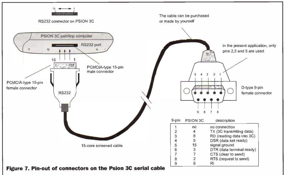
**Figure 7. Pin-out of connectors on the Psion 3C serial cable**
