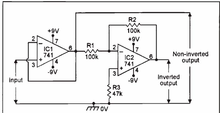
**Figure 15. Unity-gain balanced dc phase-splitter.**
