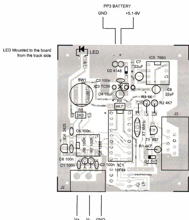
LED Mounted to the board from the track side
