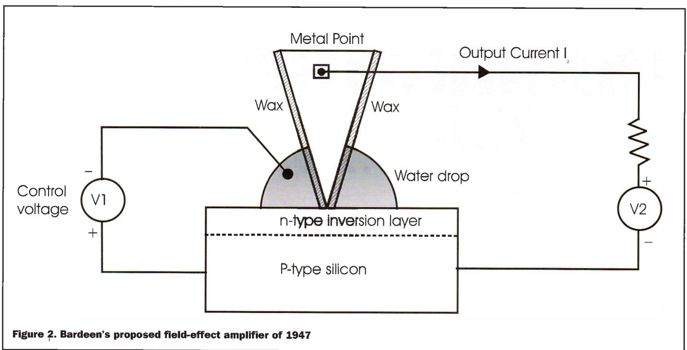
**Figure 2. Bardeen's proposed field-effect amplifier of 1947**
