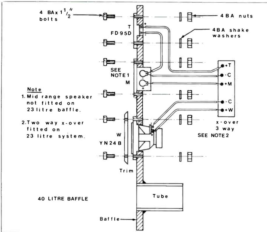
**Figure 12. Baffle mounting.**
