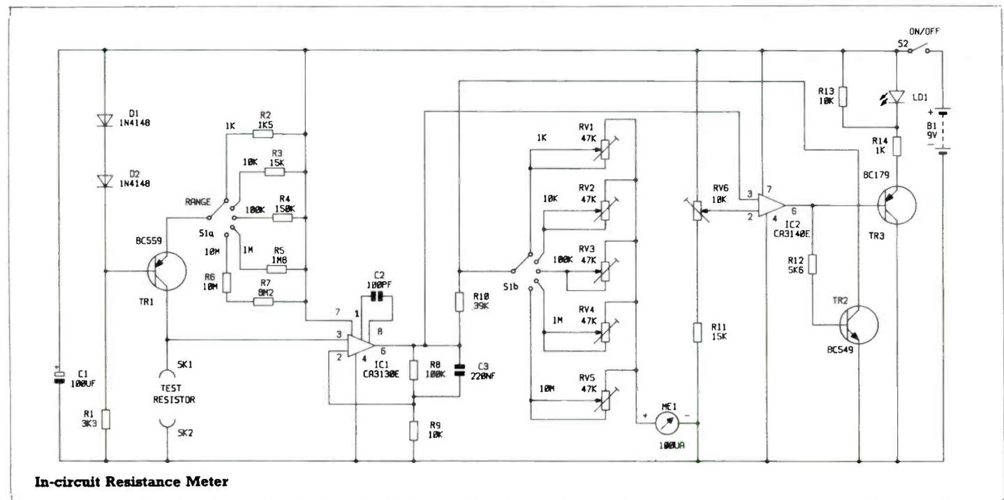
Semiconductor junctions (which can be in diodes, transistors, integrated circuits, or practically any semiconductor component) are often forward biased by the voltage source in the multimeter, and this results in a very low reading. Sometimes simply reversing the test leads will cure the problem, but although this might eliminate the original junction by reverse biasing it, it may well forward bias a second junction and re-introduce the problem.
