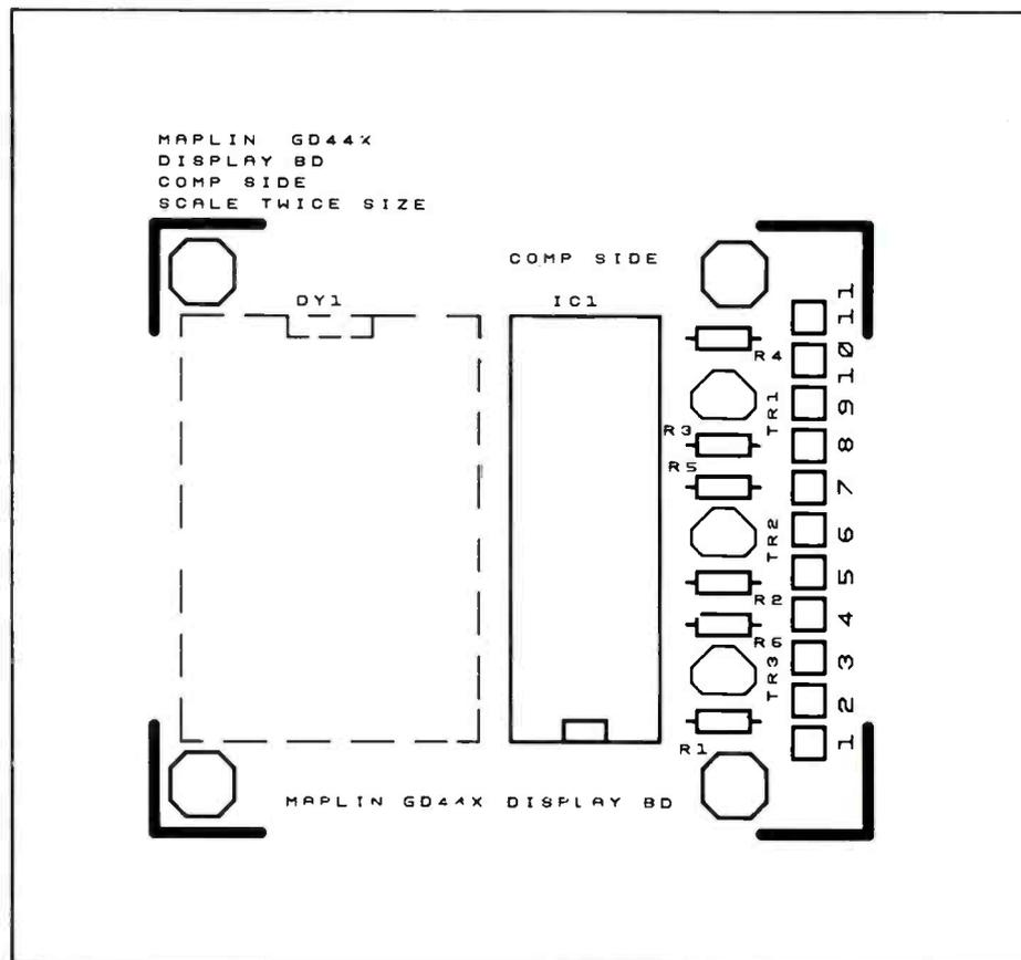
Figure 2. PCB layout.
