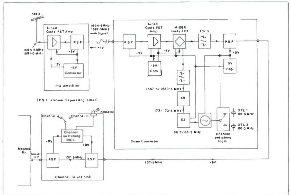
Figure 3. Block schematic of the system.
