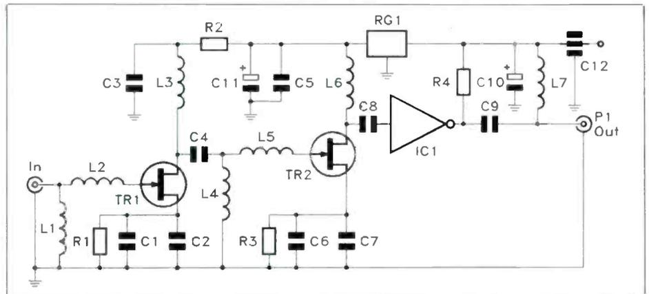
Figure 4. Pre-amplifier circuit.
