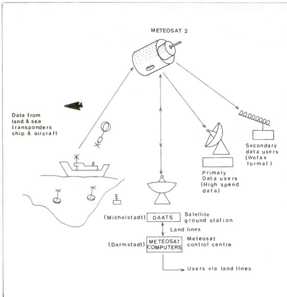
Figure 2. Meteosat 2 receiving station.
