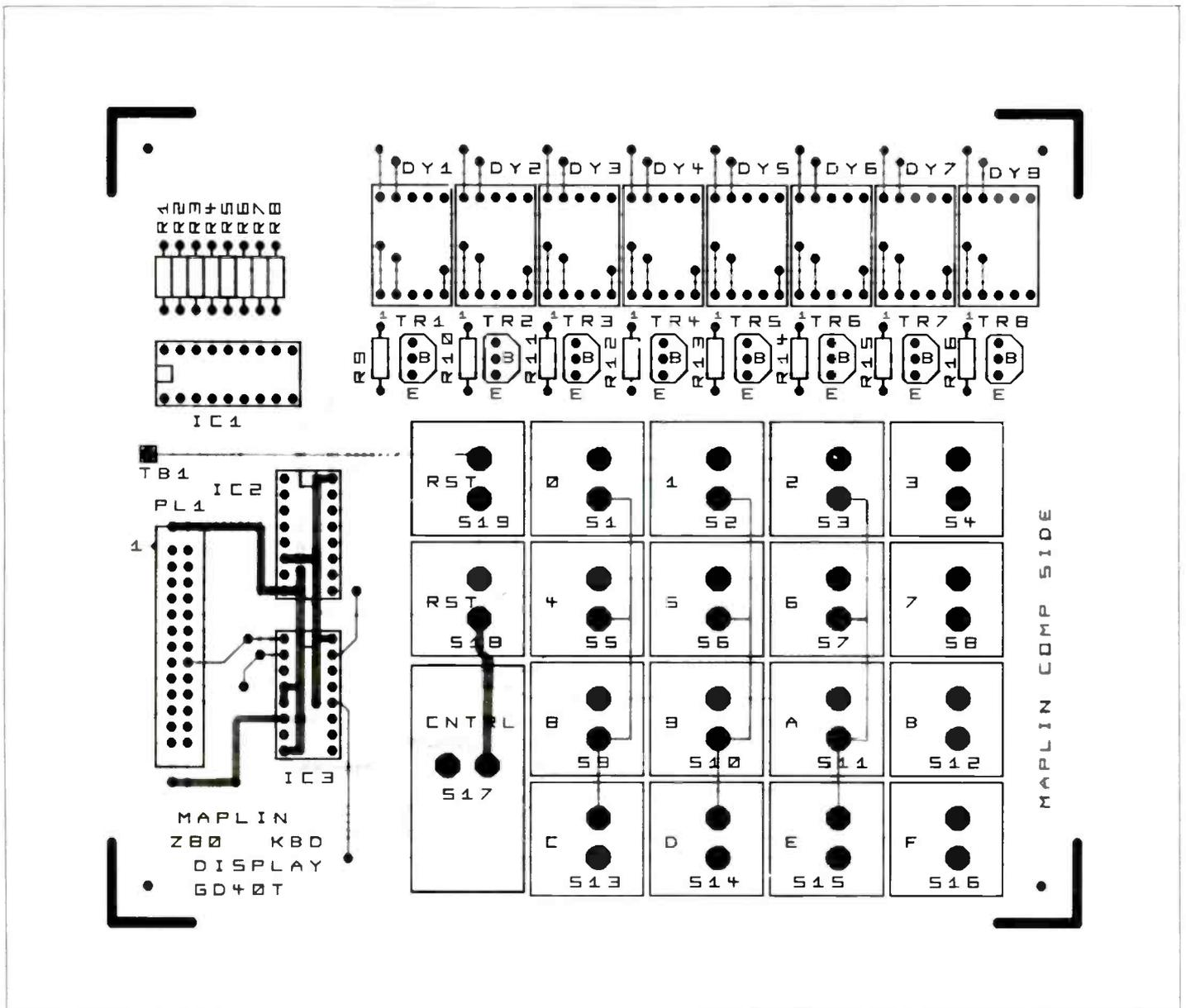
Figure 2. PCB Layout.
