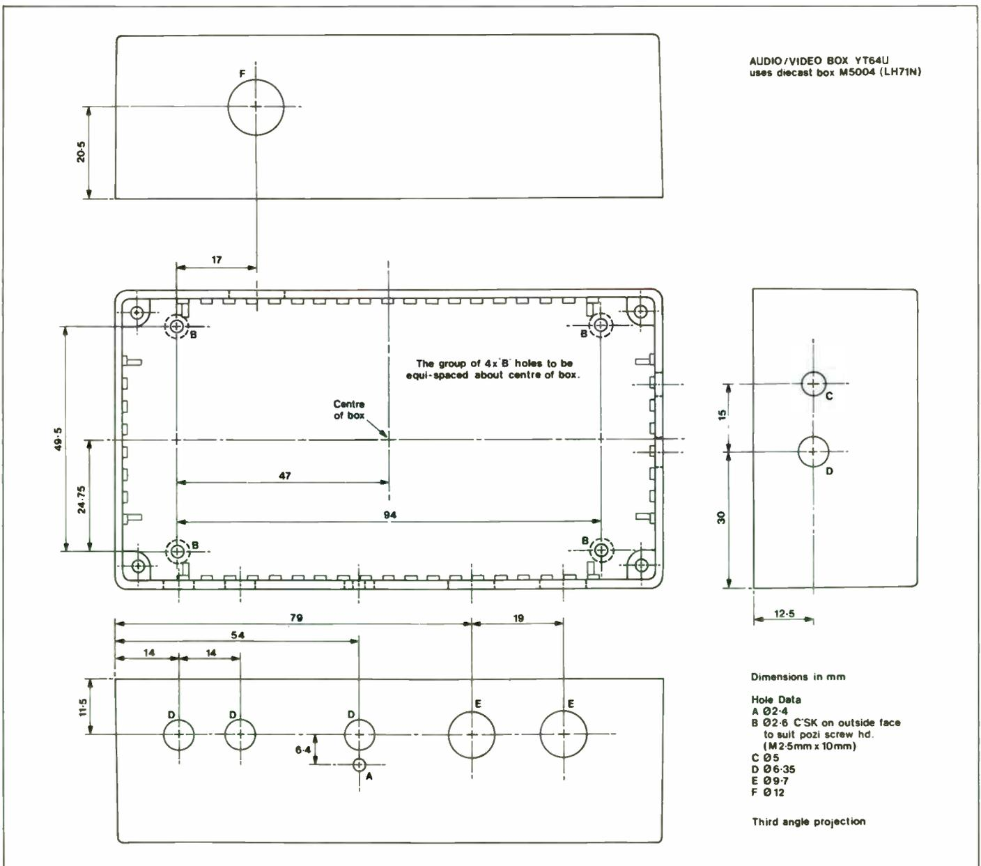
Figure 6. Box drilling.
