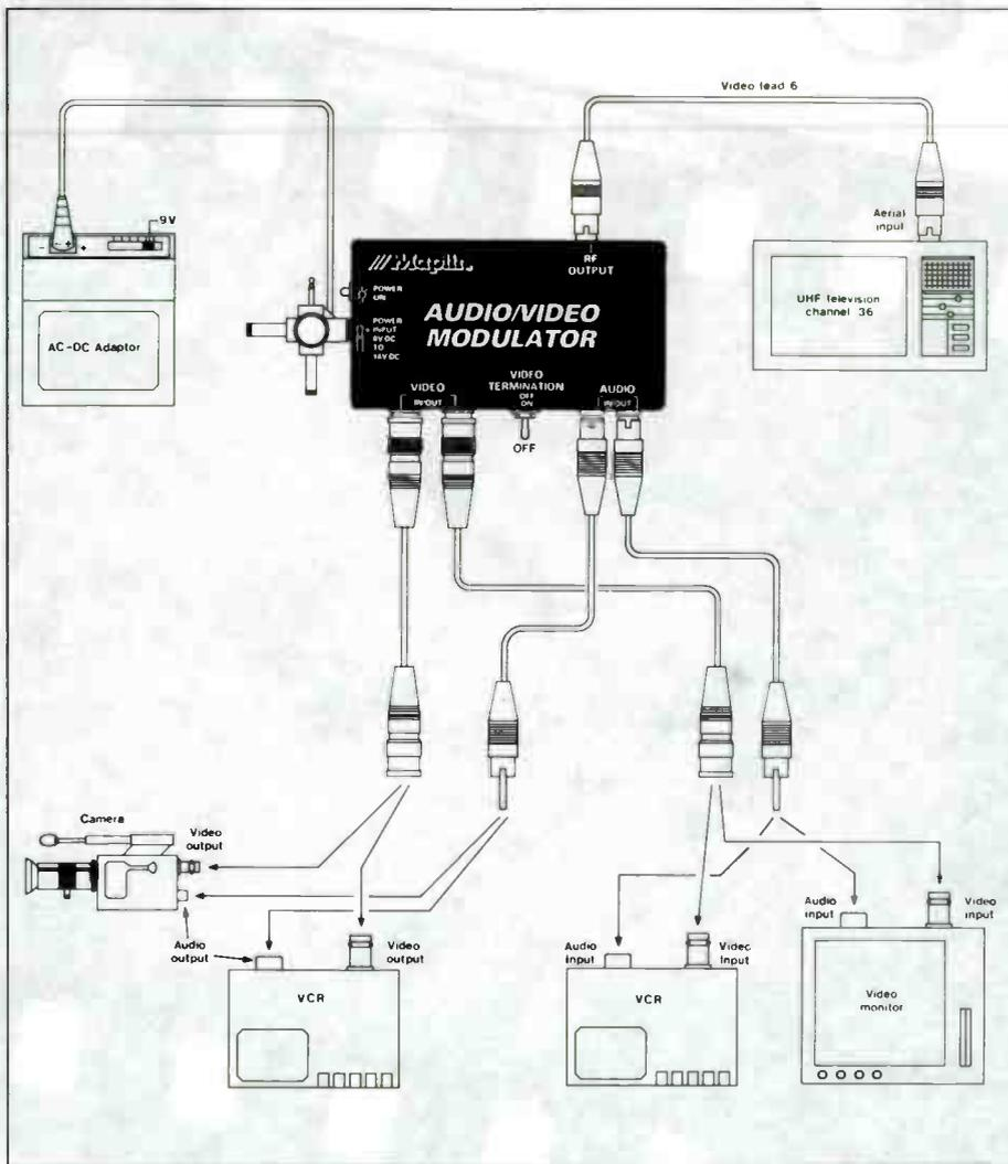
Figure 1a. Audio and video connections.
