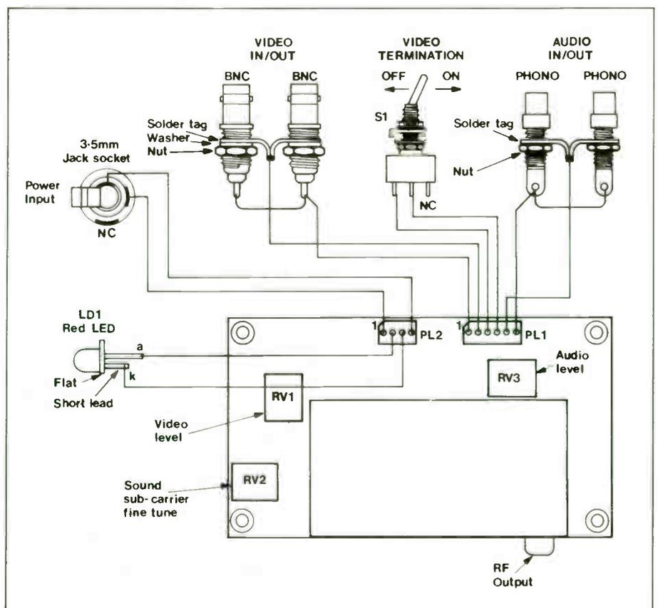
Figure 5. Wiring.
