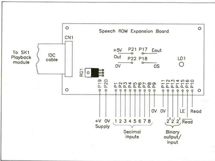
Figure 7. Connections to Speech ROM Expansion Module.
