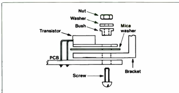
Figure 7. Mounting IC1.
