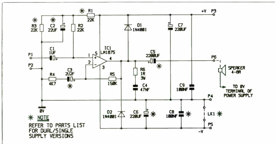
Figure 5. Combined circuit to which PCB is designed.
