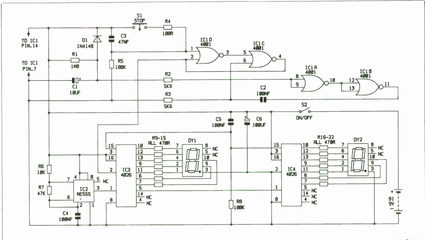
**Reaction Tester Circuit.**
