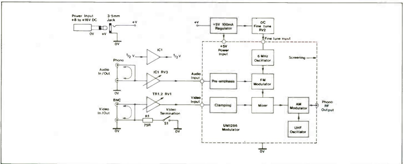
Figure 2. Block diagram.
