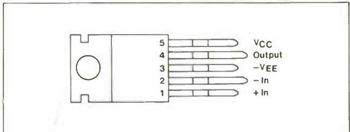
Figure 1. Pin-out of the LM1875.
