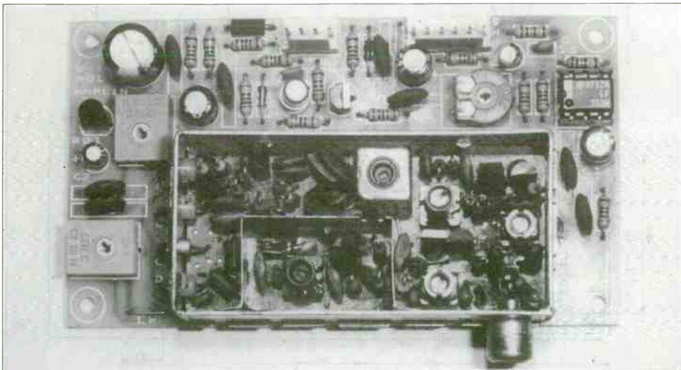
Photo 3. Completed PCB assembly (with modulator lid removed).
