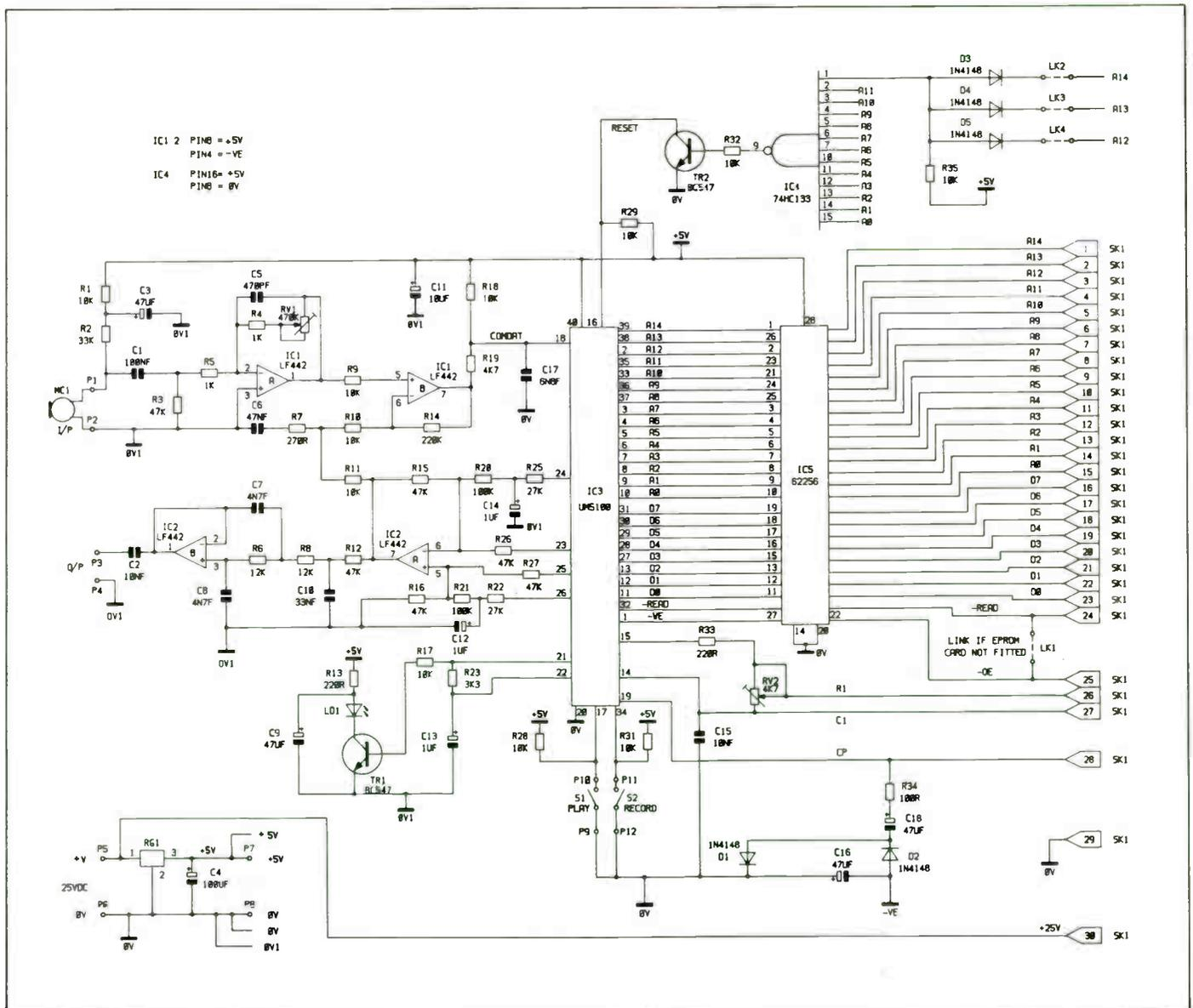
Figure 2. Circuit of the record/playback module.
