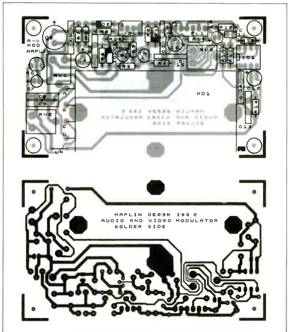
Figure 4. Track and layout of the PCB.
