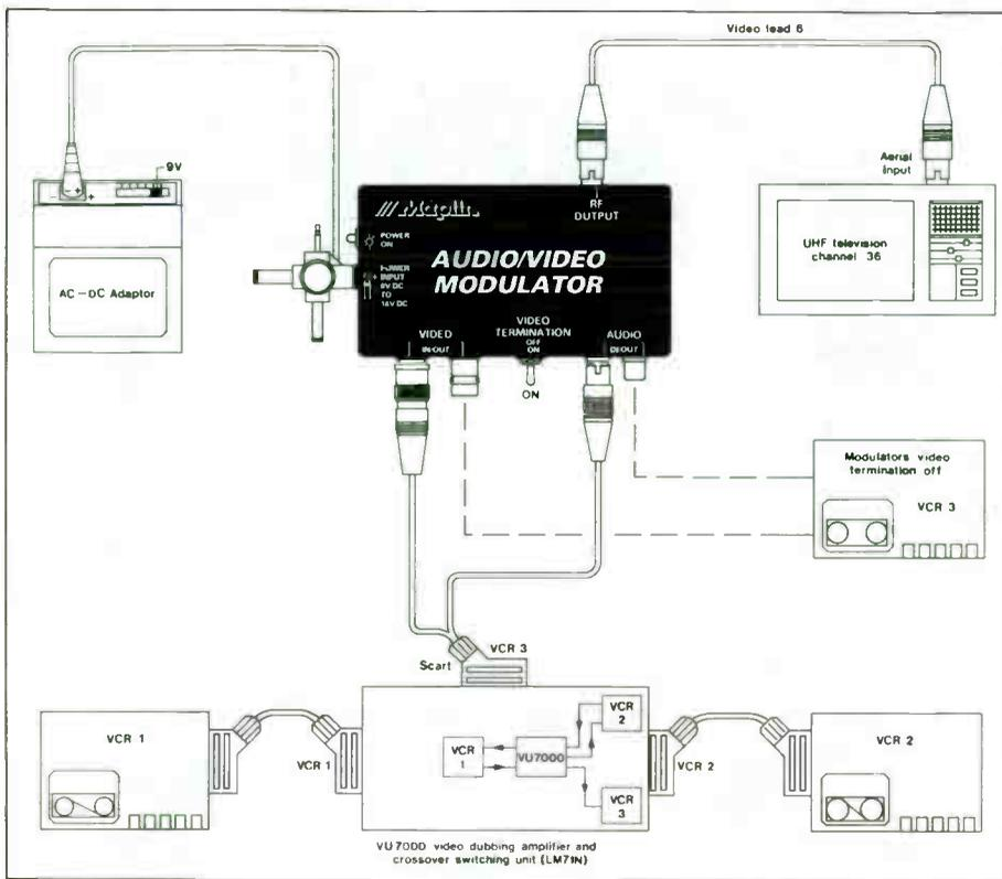
Figure 1c. VU7000 connections.
