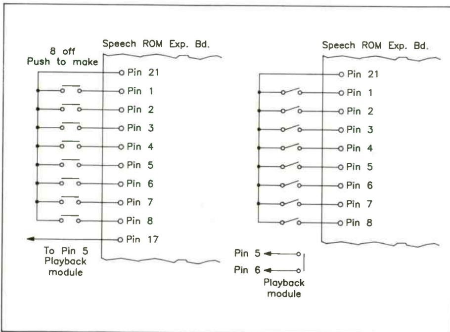
Figure 8a & 8b. Connecting switches to Speech ROM Expansion Module.
