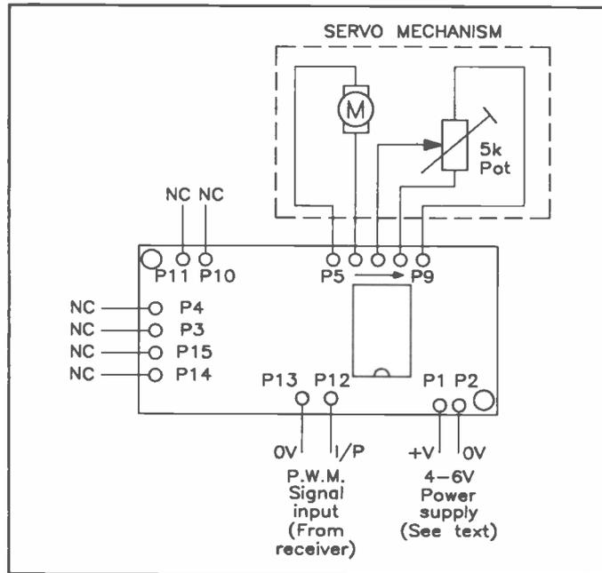
Figure 5. Servo driver wiring diagram.
