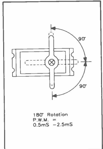
Figure 7. Servo operation.
