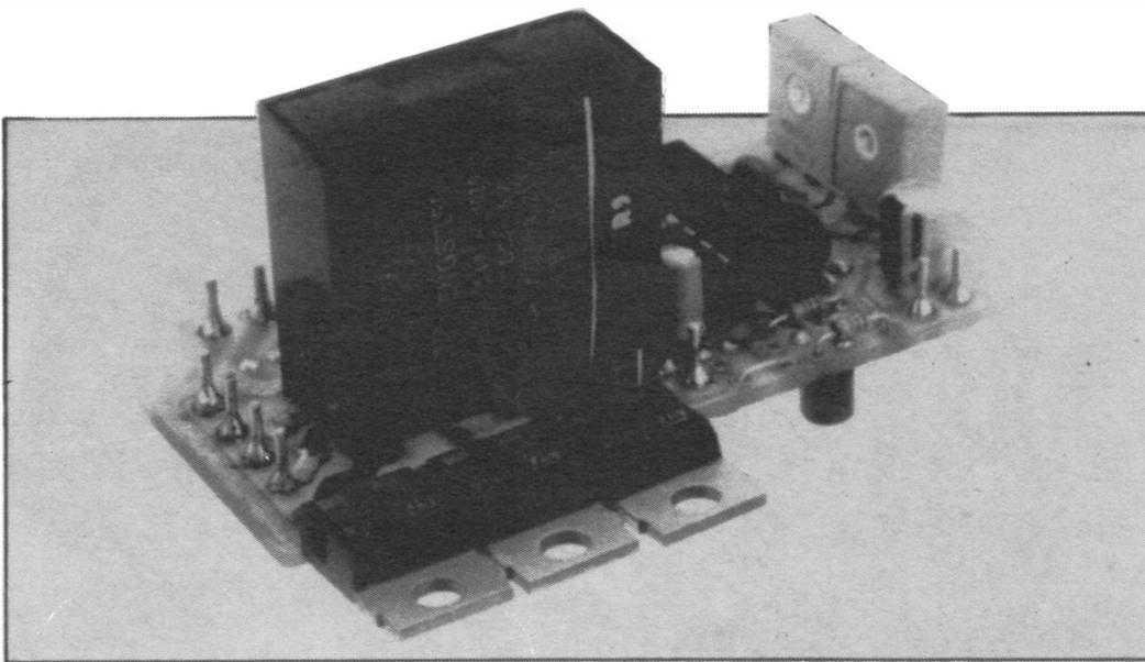
Photo 2. Note how the power transistors are mounted on the motor driver option.
