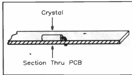
Figure 6. Mounting the crystal Q1.
