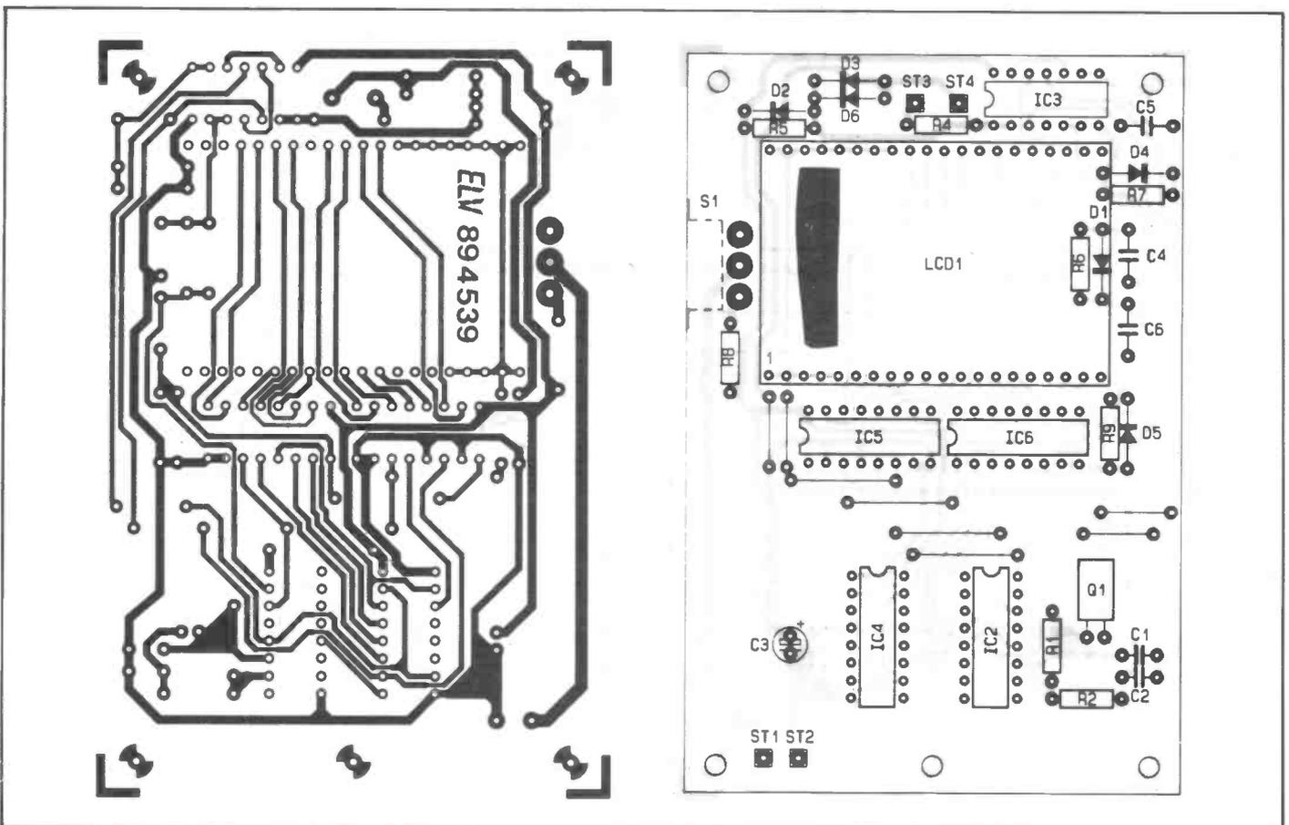
Figure 5. Printed circuit board for the receiver.
