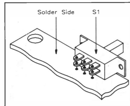
Figure 9. Mounting the receiver's on/off switch.
