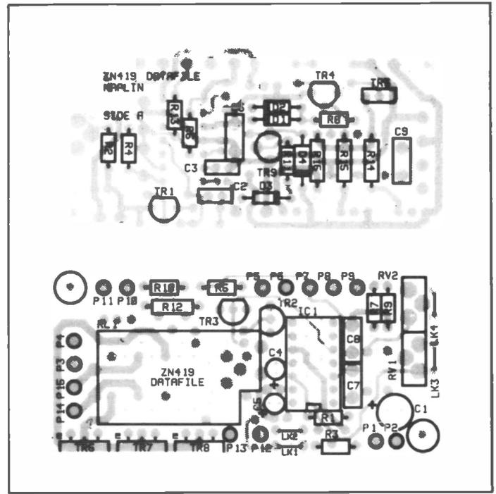
Figure 3. Legend on both sides of PCB.
