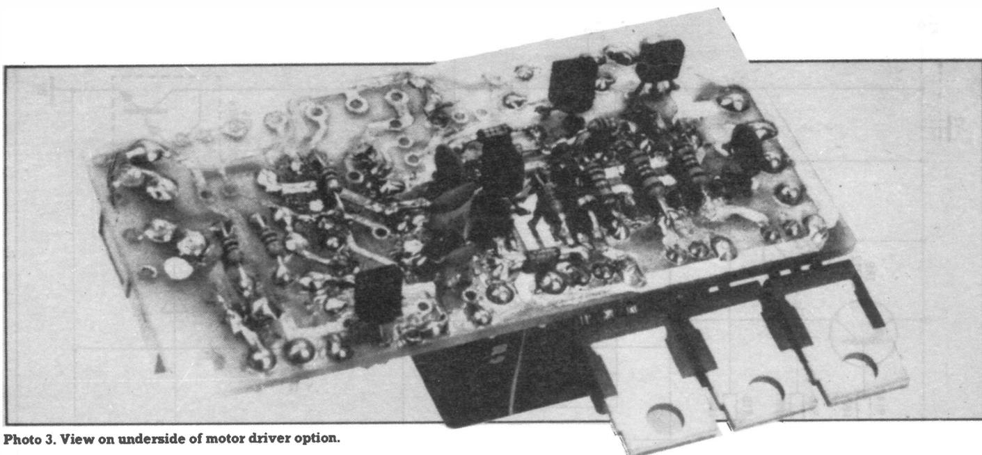
Photo 3. View on underside of motor driver option.
