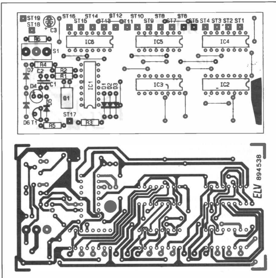
Figure 4. Printed circuit board for the transmitter.
