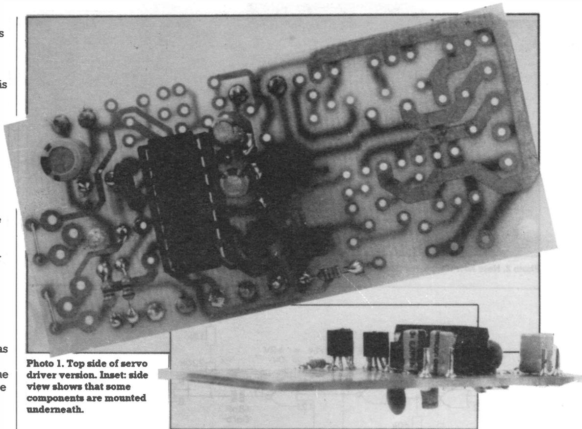
Photo 1. Top side of servo driver version. Inset: side view shows that some components are mounted underneath.
