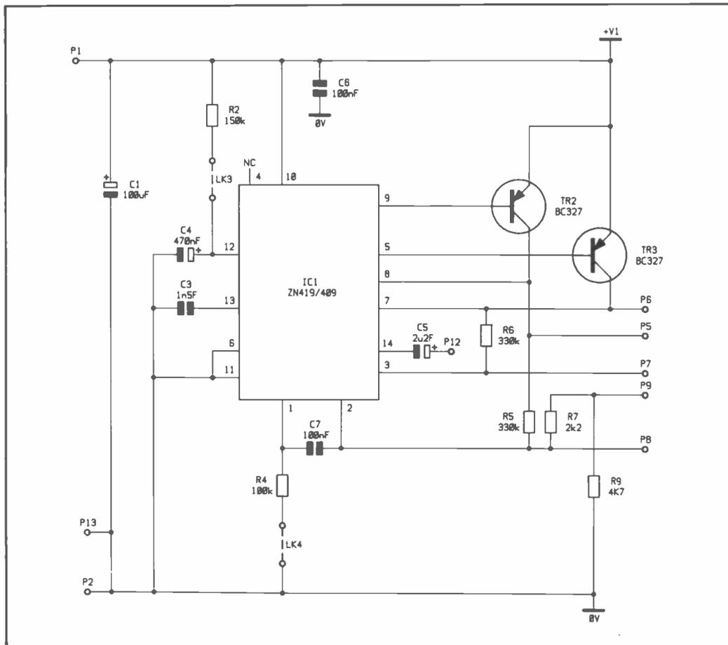
Figure 4. Circuit diagram of servo application.
