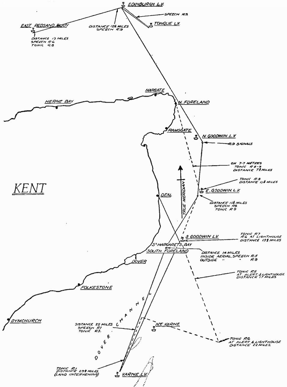
FIG. 2, Chart of Trinity Steamer "Alert" during S.A.I Range Trials.
