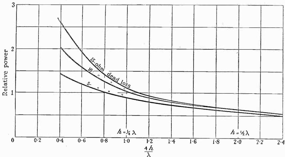
FIG. 2.—Relative power required to produce a given value of metre-amperes.
