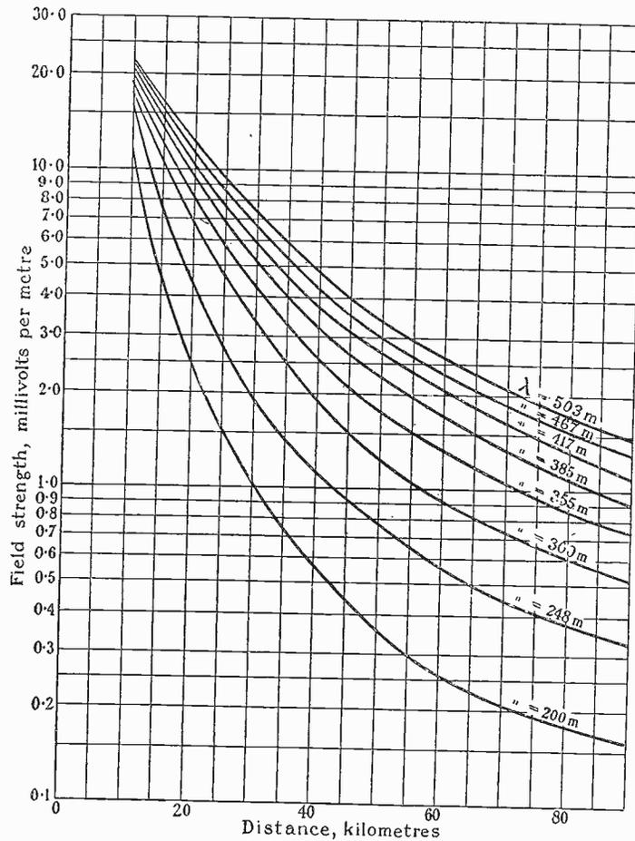
FIG. 6.—Mean attenuation curve for  $\frac{1}{4}\lambda$  transmitting aerial with 10-ohm dead loss and 1 kw. input to aerial.
