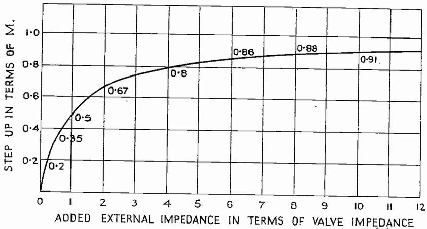
FIG. 2.—Curve showing the step-up obtained in terms of  $M$  for added impedance of different values.
