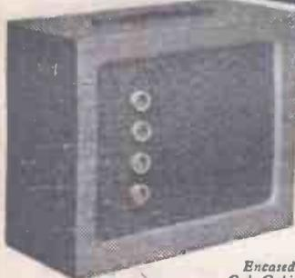
Specification: 2 inputs for Guitar, Record Player, and Mike. Four independently matched controls, giving variable treble cut and bass boost. Printed Circuit, using double triode and EL 84 output with contact-cooled rectifier. Frequency response +0.5 to -1db, 40 c/s to 20 kc/s, giving 5/6 watt output, with fine quality 8" Internal Speaker.
