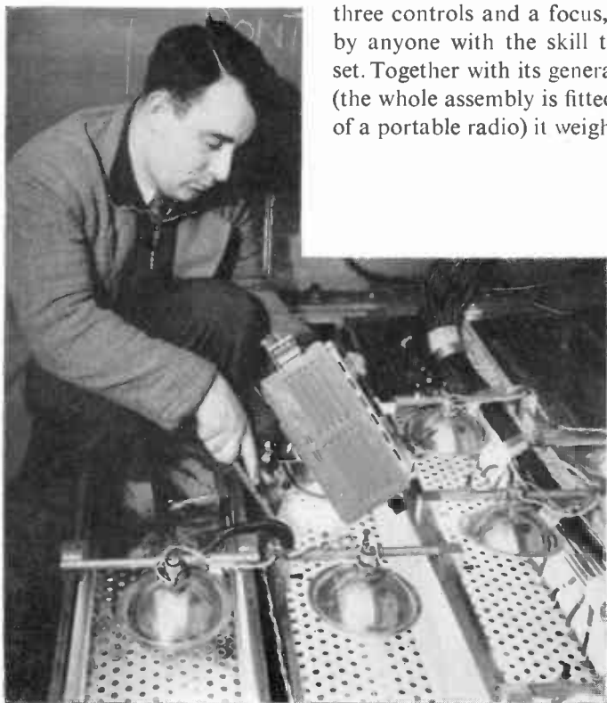
TV helps aircraft research. The Aircraft Research Association's new trans-sonic wind tunnel has an inner porous wall which does not admit the usual glass observation window. A miniature TV camera, surrounded by special lighting, fits over one of the perforations in the inner wall and gives a clear picture of the model under test.
