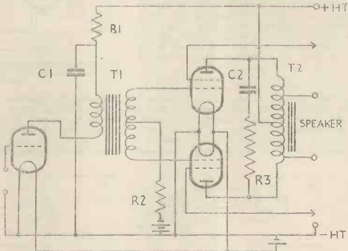
transformer—usually one with a ratio of about 10-1. This is of the centre-tapped or push-pull variety.
