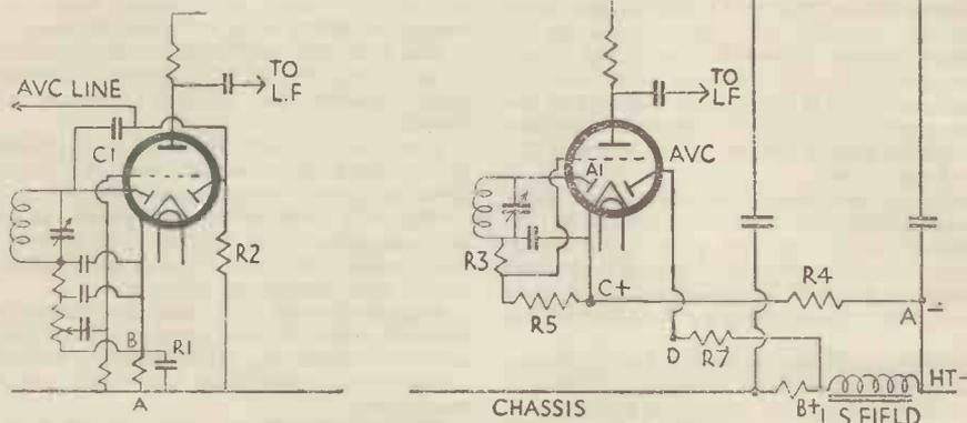
FIG. 4 (on the left) shows the simplest delayed A.V.C. circuit, and FIG. 5 (right) gives the most popular arrangement for amplified A.V.C. The A.V.C. line to the H.F. valves is taken from D in FIG. 5.
