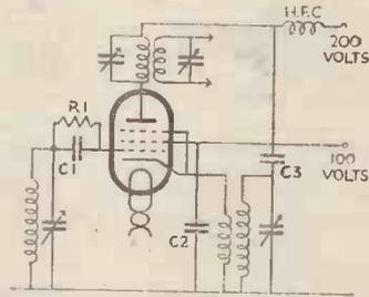
ohms.; R.3, 500 ohms; R.4, 60-70,000 ohms; R.5, 7,000 ohms; C.1, .1 mfd.; C.2, .1 mfd.; C.3, .0005 mfd.; C.4, .0003 mfd.; C.5, .001 mfd.
