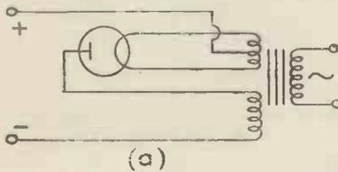
FIG. 20.—Half and full wave valve rectifier circuits.
