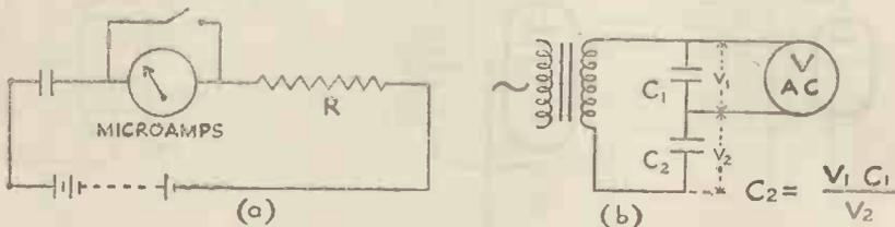
FIG. 7A.—When measuring the insulation of a condenser, a safety resistance  $R$  must be included in the circuit, the microammeter being shorted by a switch, while the condenser charges. How the capacity of a condenser can be checked is shown in (B).
