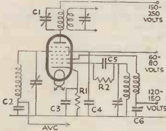
FIG. 15.—On the left is a circuit (simplified as regards coil switching) showing how a heptode is used as a combined detector-oscillator or frequency-changer. In Fig. 16 (right) the connections for using an H.F. pentode for the same purpose are indicated.
