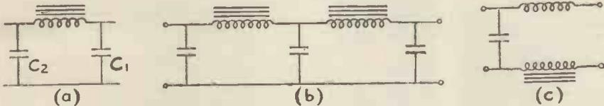
FIG. 10.—Three examples of fundamental smoothing circuits comprising iron cored chokes and large condensers.
