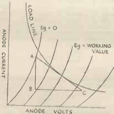
as shown in the diagram. AB equals change in anode milliamps and BC change in anode volts.
