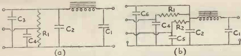
FIG. 11.—Shows two voltage distribution systems. (a) Potentiometer method. (b) Series resistance method.
