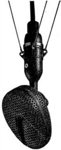
The 4105 microphone is a moving coil pressure-gradient microphone with a cardioid response obtained by using an acoustic phase shifting network. It is small, unobtrusive and robust.
