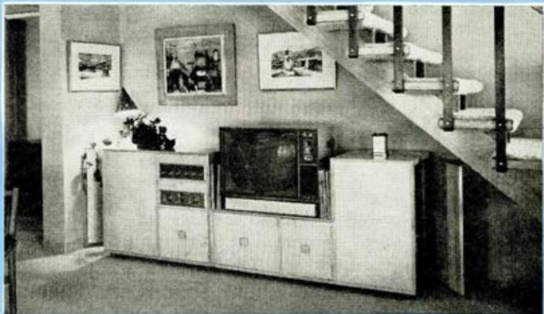
**SOUND UNDER THE STAIRS** — *In this installation the speakers are mounted at each end and the adjustable doors reflect the sound into the room. The television chassis is rotatable, stereo radio, tape and record reproduction is provided (H. H. SCOTT).*
