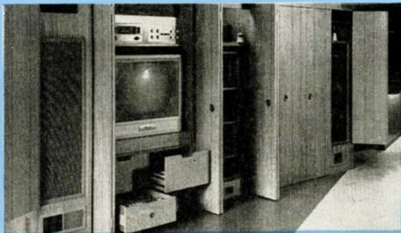
**THE WHOLE WORKS** — Built-in installation comprising remote-controlled television, stereo control unit with separate amplifiers, A.M./F.M. tuners, stereo tape deck and pre-amplifiers, multi-channel loudspeaker system and two changers — one for father's favourite records and the other for the children! (AUDIO EXCHANGE).
