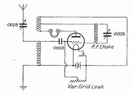
FIG. 1.-THE UNIDYNE CIRCUIT FOR H.T.-LESS RECEPTION
