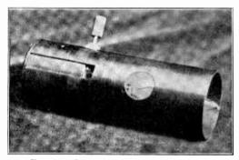
FIG. 11.—CELL FOR TRANSFORMING LIGHT FLUCTUATIONS INTO ELECTRIC CURRENTS
