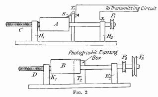
One of these may be of wood (for the receiver), but the transmitter drum should be of metal, a 5 in. length of 2 in. brass tubing fitted with metal ends accurately bored to take a  $\frac{3}{8}$  in. or  $\frac{1}{2}$  in. shaft.
