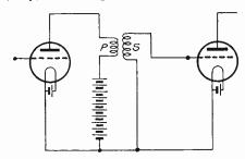
FIG. 2.-TRANSFORMER COUPLING
