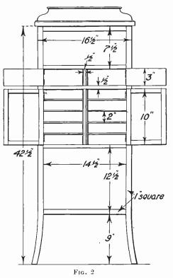
The spaces above and below the doors are filled in by three-ply wood, sizes  $6\frac{1}{2}$  in. by  $14\frac{1}{2}$  in. and  $11\frac{1}{2}$  in. by  $14\frac{1}{2}$  in. respectively.
