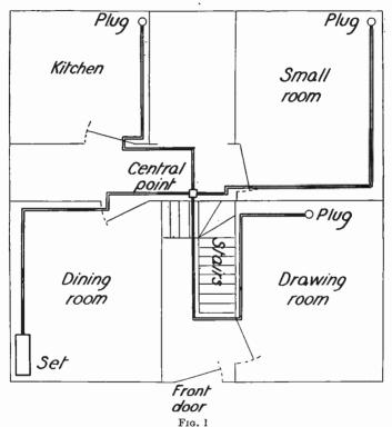
which upstairs rooms will be supplied. In this way, one central joint on each floor is used, and, if this joint is soldered and well covered with insulating tape, efficient results can be assured for years of wear. Then leads should be run to the various rooms on
