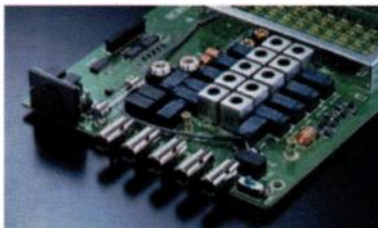
The VRF circuitry uses high-Q components to protect the receiver front end.
