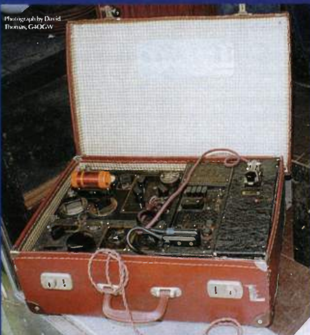
The B2 'suitcase radio', as used by Violette Szabo during WWII. An example of this set is on permanent display at the RSGB National Amateur Radio Museum at Potters Bar.
