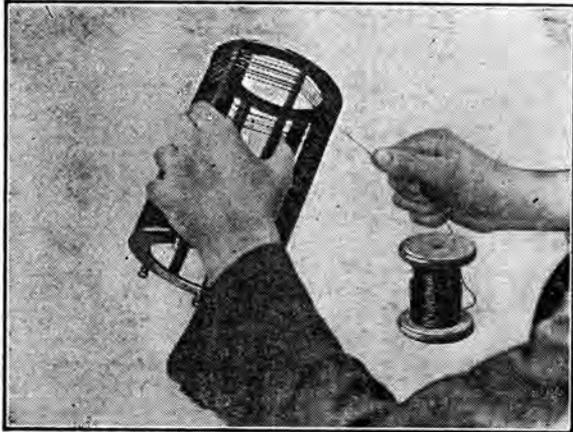
The "Three-step" coil is one for which enamelled wire is suitable.
