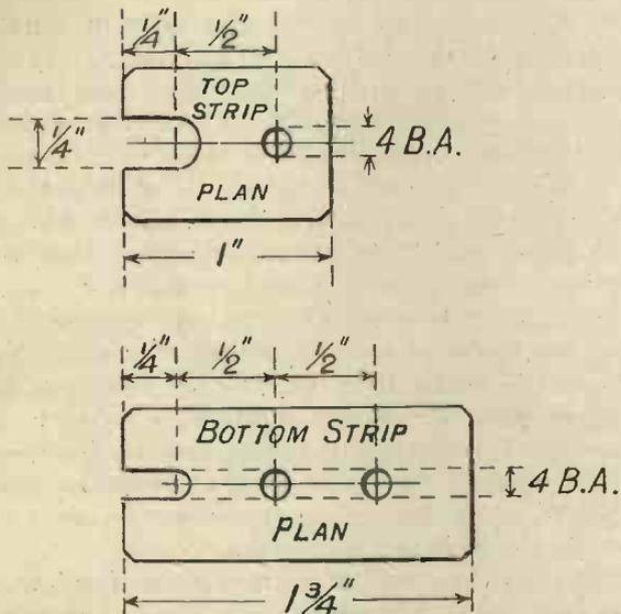
Fig. 2. Details of brass strips.
