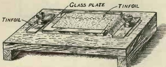
Fig. 8. Illustrating a home-made grid condenser.
