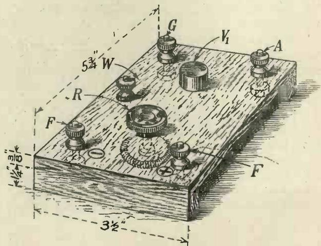
Fig. 11. Illustrating a suitable valve panel.
