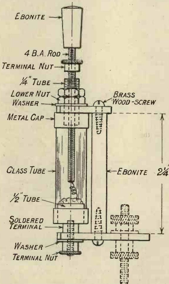
Fig. 1. General arrangement of detector.
