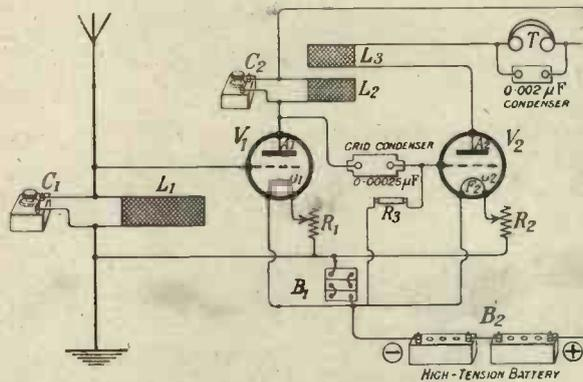
Fig. 2. Showing the wiring of the set.
