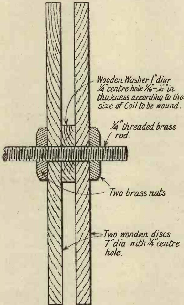
Fig. 1. Section of slab coil winder.
