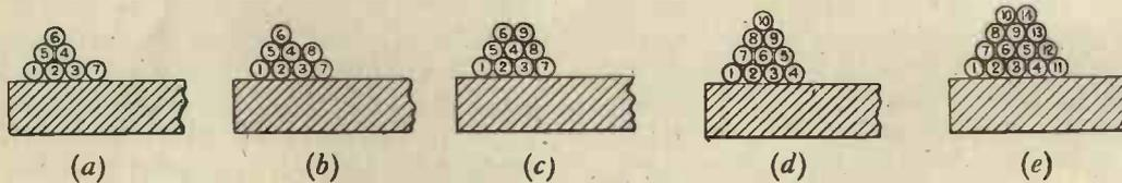
Fig. 6. Commencement of a four-pile winding.
