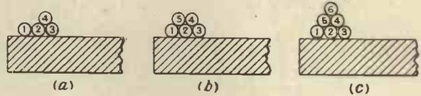
Fig. 5. Commencement of a three-pile winding.
