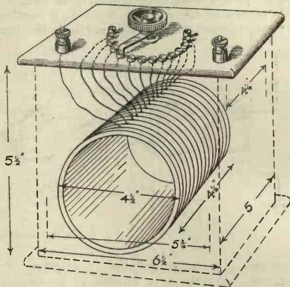
Fig. 6. The coil in position.
