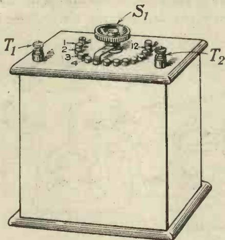
Fig. 4. Showing the appearance of the finished inductance unit.
