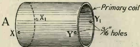
Fig. 4. Details of primary tube.
