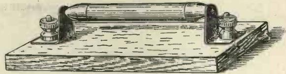
Fig. 10. The holder for the grid leak.
