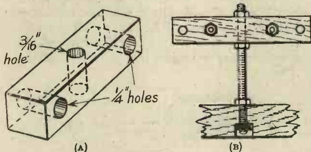
Fig. 7. Supports for the secondary.
