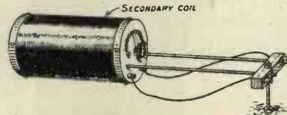
Fig. 5. Assembly of secondary coil.
