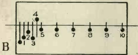
Fig. 3. Tapping points on secondary.
