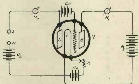
Fig. 2. A circuit for obtaining the characteristic curve of the negatron.
