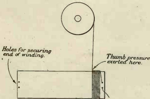
Fig. 1. Illustrating method of winding.
