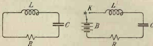
Figs. 2 and 3. Illustrating the application of a direct-current potential to a circuit containing inductance and capacity, but little resistance.
