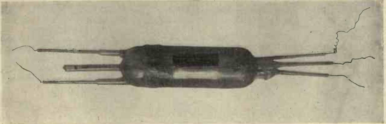
Fig. 5. A silica negatron used as a generator for transmission purposes.
