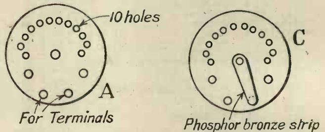
Fig. 2. Arrangement of secondary switch.
