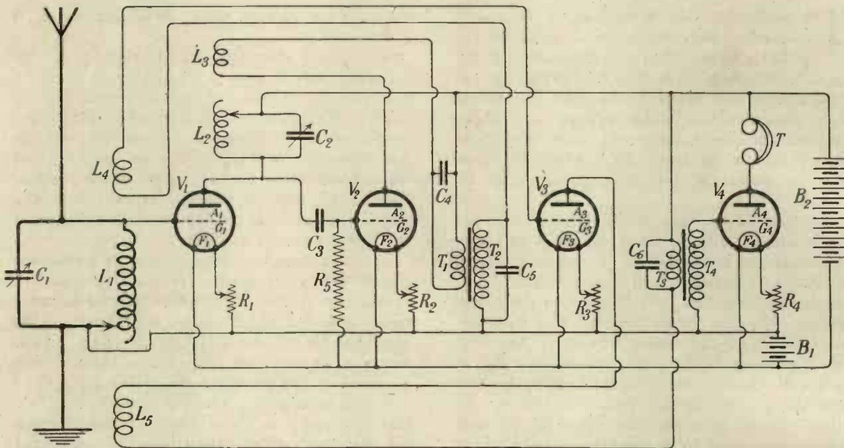
Fig. 1. The new circuit, which enables reaction effects to be produced in both aerial and anode circuits independently.
