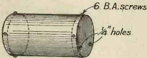
Fig. 1. Tube for secondary winding.
