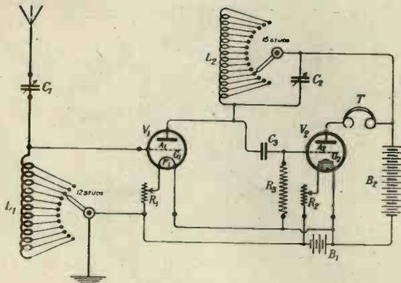
Fig. 3. Circuit of the two-valve receiver.
