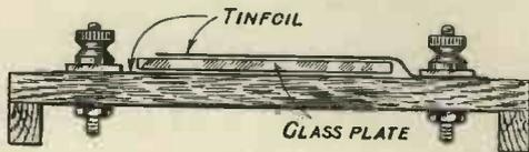
Fig. 9. Side view of the grid condenser.
