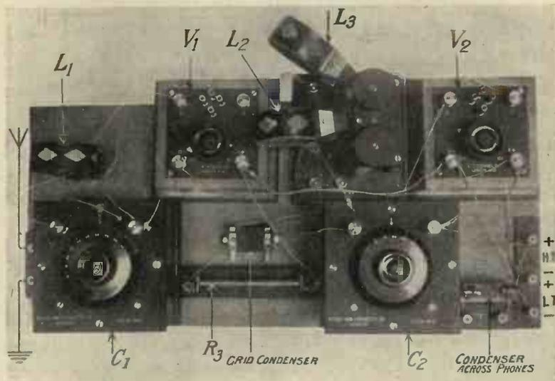
Fig. 1. Illustrating the arrangement of the two-valve receiver.
