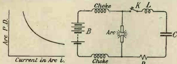
Figs. 5 and 6. The characteristic curve and fundamental circuit used with the arc.
