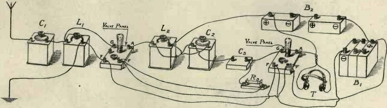
Fig. 2. Connections of the two-valve set.
