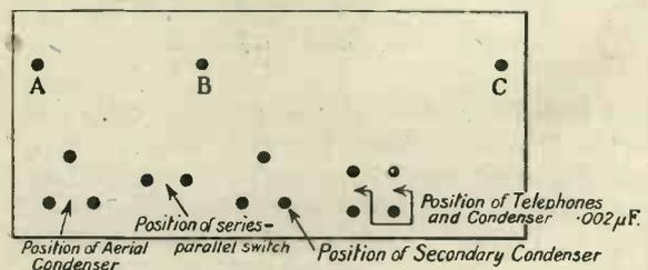
Fig. 6. Plan of the base-board.
