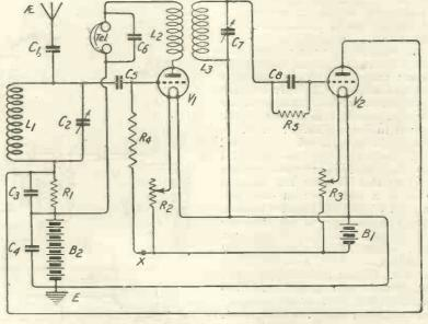
Fig. 1. An H.F. transformer coupled resistofiex.
