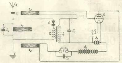
Fig. 1.-A method of Improving a crystal and I.L.F. Circuit.
