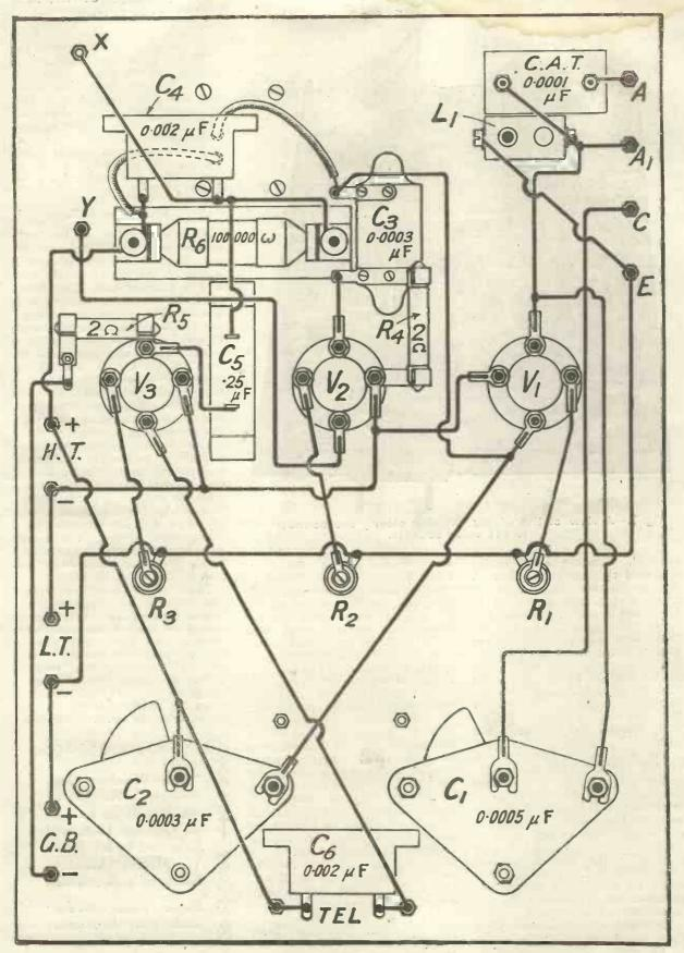
Fig. 6.-Back-of-panel wiring diagram. Blue Print No. 66B.
