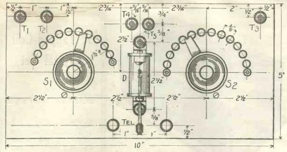
Fig. 3.-Dimensioned plan of the panel from which drilling may easily be carried out.
