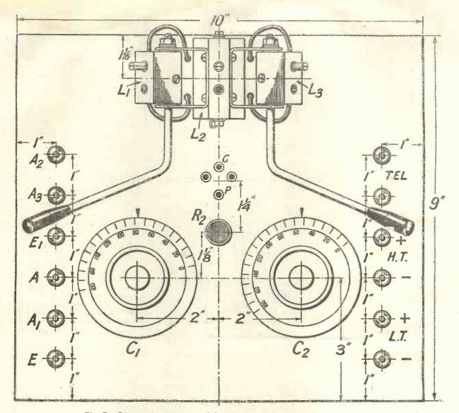
Fig. 7.-Dimensioned plan of front of panel. Blue Print No. 67A.
