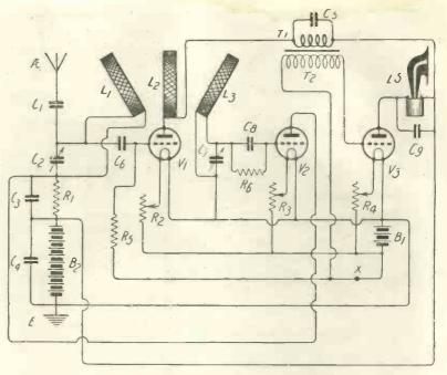
Fig. 8.—A three-valve resistoflex.
