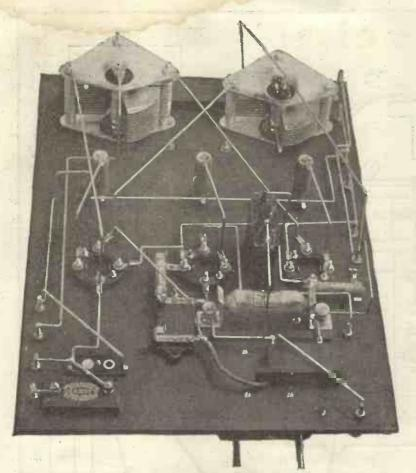
Fig. 7.—A view of the wiring showing clearly the connection to the valve sockets.
