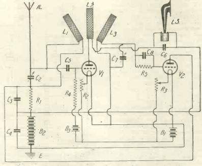
Fig. 5.-A recommended form of resistoflex circuit.
