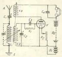
Fig. 2.- The theoretical circuit, using the loose-coupled arrangement.
