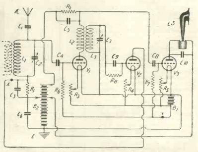
Fig. 7.—The reaction coil shown in dotted lines might occupy the position indicated by x.
