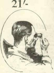
Illustration showing laboratory worker taking a temperature reading by means of the Pyrometer—an instrument for measuring temperatures which cannot be obtained by means of the ordinary thermometer system.
