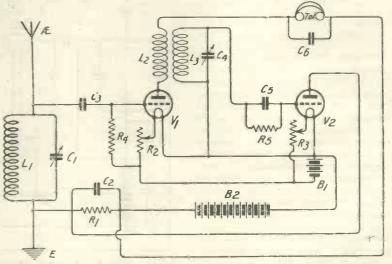
Fig. 3.—This arrangement has certain disadvantages but keeps the aerial circuit clear.
