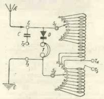
Fig. 2.—The theoretical circuit of the receiver.
