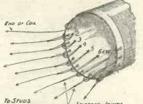
Fig. 5.—The inside of the coil. Notice how the tappings are brought out.
