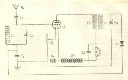
Fig. 4. A modified type of reflex circuit introduced by P. G. A. H. Voight.
