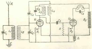
Fig. 43.—The Cowper arrangement of stabilising a tuned anode circuit.
