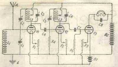
Fig. 39.—Individual stabilisation of two high-frequency valves in which delicate adjustment is required.
