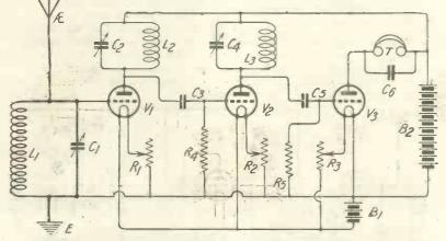
Fig. 34:—A two tuned anode circuit which has a pronounced tendency to fall into self-oscillation.
