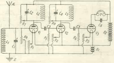
Fig. 35.—The introduction of parallel resistance to obtain stability.
