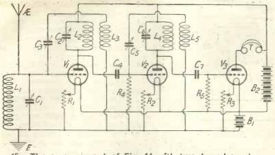
45.-The arrangement of Fig. 44 with two tuned anodes.
