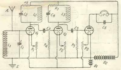
Fig. 36.—Circuit showing series stabilising resistances favoured by the author.
