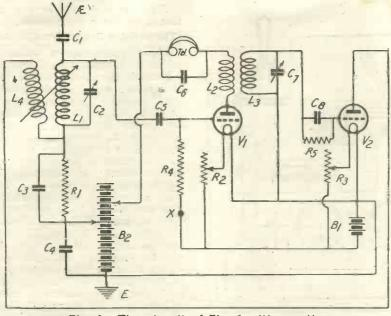
Fig. 4.- The circuit of Fig. 1 with reaction.
