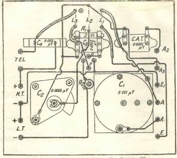
Fig. 8.-Back - of - panel wiring diagram. Blue Print No. 67B.
