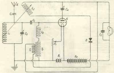
Fig. 3.—A choke coil method of feed-back which has certain advantages.
