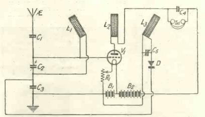
Fig. 5. The introduction of reaction by the "Tri-coil" system.
