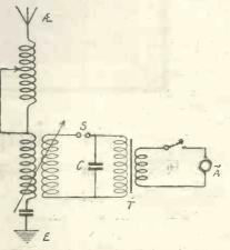
Fig. 2.—A circuit diagram of a simple spark transmitter.
