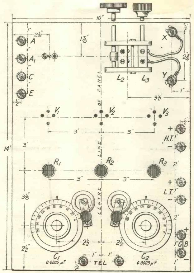
Fig. 4.—Drilling diagram showing front of panel. Blue Print 66A.
