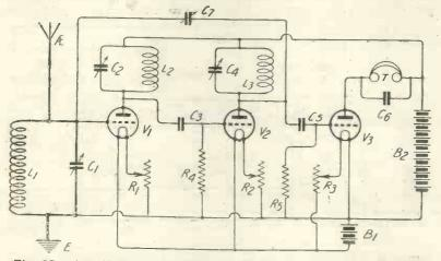
Fig. 38.—A collective method of stabilisation which is difficult to handle.
