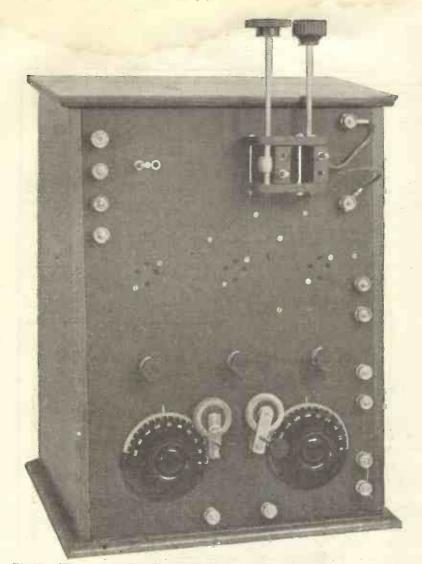
Fig. 5.—The set with coils and valves removed to show how the components are disposed.
