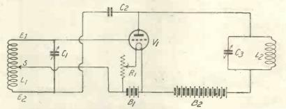
Fig. 31.—A circuit in which valve capacity is neutralised by a tap on the grid circuit.
