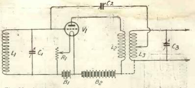
Fig. 33.—A circuit in which the tapping is taken from the grid circuit of the next valve.
