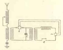
Fig. 4.—The Marconi synchronous spark transmitter circuit.
