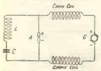
Fig. 5.—The circuit of an arc transmitter.
