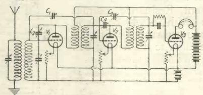
Fig. 40.—A circuit suggested by the author in which stabilising adjustments are less critical than in Fig. 39 circuit.
