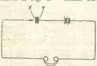
Fig. 4.—A test which makes a short circuit evident.
