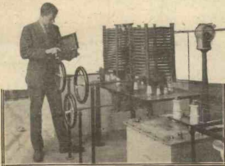
Wavelength measurements at Daventry. The wave-meter is being used to check the tuned circuits in the 5XX transmitter.
