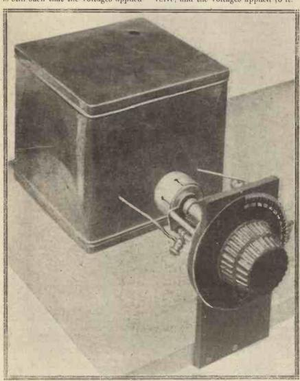
A standard "Modern Wireless" screening box experimentally wired up. A complete tuned H.F stage is represented by this and the variable condenser. When the lid is properly in position the control handle of the neutralising condenser passes through the hole that can be seen.
