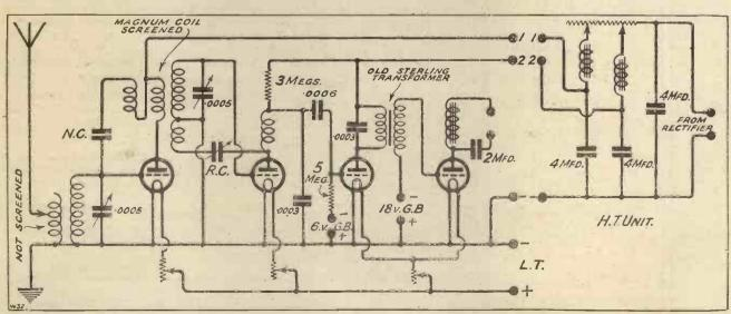
The four-valve circuit employed by Mr. W. H. Lowe. About 60 stations have been received at loud-speaker strength.
