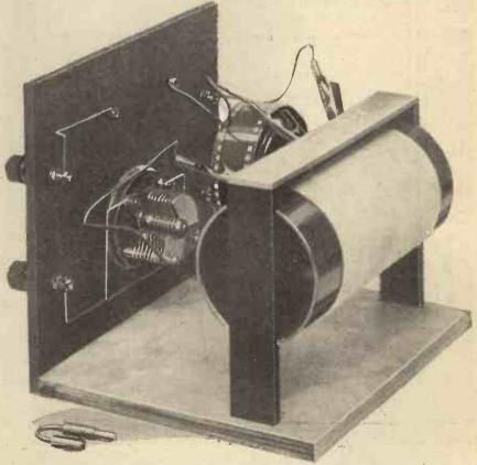
This view was specially taken to show the method of mounting the coil.
