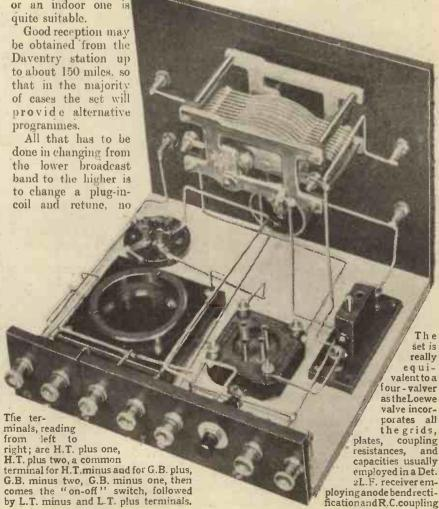
H.F. amplification, and may be any low impedance H.F. or small power valve. The aerial circuit is directly coupled, consisting of a plug-in coil tuned by the variable condenser. In the
