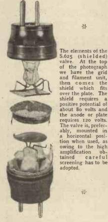
fore, the valve is, as far as its own internal capacities are concerned, self-neutralising. External wiring has to be carefully arranged, however, in order not to defeat the object of the valve by introducing outside unneutralised capacities.
