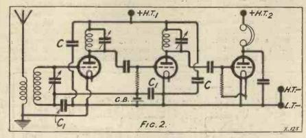
resistances, but when two or three stages of high-frequency amplification are being used with considerable magnification it may be necessary to take all of these precautions. Chokes connected in the anode-battery feed-wires in conjunction with by-
