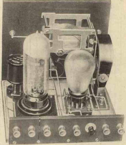
with some fixed condensers of 2 to 4 This back-of-panel photograph shows the set ready for use with H.F. transformer, coil, mfds. total capacity. This is, as a and valves in position.
