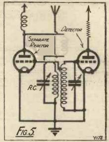
In view of the points considered above there can be little doubt that the addition of a separate reactor valve is well worth while. The utmost efficiency with the least distortion can only be obtained from modern types of valve rectifiers by employing this separate reactor. Therefore, apart from receivers with H.F. stages requiring no direct reaction, this system undoubtedly deserves more attention from progressive experimenters.
