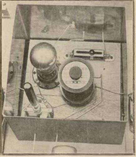
A typical example of the scientific application of screening to a complete H.F. stage; one of the new standard "Modern Wireless" screening boxes wired in a receiver, but with its lid removed to show the components,
