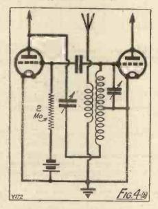
simplicity of the tuning arrangements makes it possible to construct without difficulty plug-in inductances combining the various coils for different wavelengths. With a little modification such a receiver could be used as an "All-wave" set. Results on the ordinary wave-length are almost as good as those obtainable with a powerful three-valve set.
