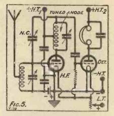
circuits L<sub>1</sub>C<sub>1</sub> and L<sub>2</sub>C<sub>2</sub>, and no common impedance, the circuit when tuned will produce most violent oscillations. We are therefore left with the stray coupling provided by the capacity of the valve.
