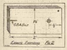
the ends of the wooden skewer as a tight fit, the wood afterwards being cut off flush with the ebonite. A small hole is also drilled near one top corner of each piece of ebonite for a bolt and nut to hold a soldering tag.
