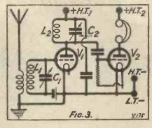
Similar chokes or resistances may also have to be joined in the grid circuits, but fortunately it is seldom necessary to do this. In some instances, though, it has been found advisable to connect 1-mfd. condensers across the filaments of the amplifying valves.
