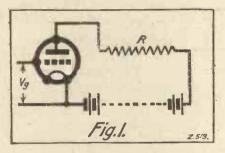
it varied with frequency. I do not quite know how valve impedance as a term came about, except that impedance is now commonly used for any mixture of resistance, capacity, and inductance effect, and if capacity and inductance are missing the term is still used, although resistance would be the only remaining factor and, of course, there is no frequency effect with a resistance.
