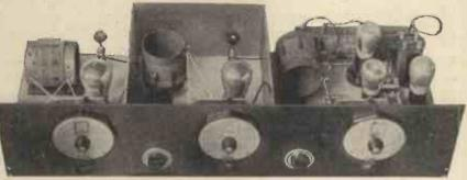
Note that the high-frequency circuits are well spaced and screened.
