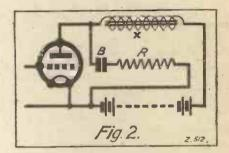
at every voltage a different value of R because the valve does not behave like a copper wire.
