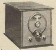
This wave-meter was constructionally described in the August issue of "M.W."
