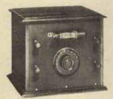
An ordinary condenser dial has been fitted to the midget condenser for convenience in tuning.
