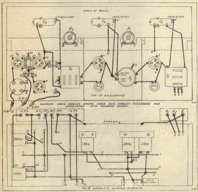
The back of panel is shown in the upper portion; the centre shows the upper side of the baseboard, while the lower section shows the under side of the baseboard. (Wires which pass through holes are numbered.)
