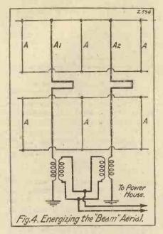
definite direction has been applied by C. S. Franklin, of the Marconi Company, to improve the working efficiency of the beam aerial.
