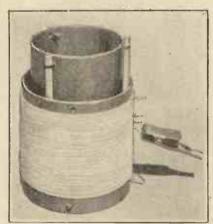
An H.F. transformer with a tapped primary winding and an adjustable coupled secondary.
