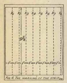
1 in. in width, and one division, at the end,  $\frac{3}{4}$  in. in width. Next, two pencil lines are drawn horizontally, parallel to the top edge of the paper, at distances  $9\frac{3}{4}$  in. and  $19\frac{1}{2}$  in. respectively from the top.
