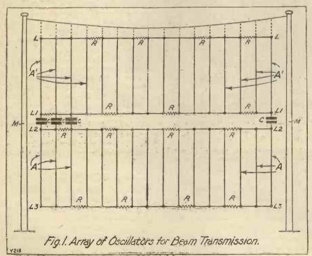
portion is practically annulled, the current distribution again becomes predominant in a direction at right angles to the aerial, giving a much sharper directional or polar diagram than before, as shown in dotted lines.
