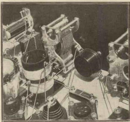
This is the "oscillator" end of a super-heterodyne receiver, and the valve which can be seen is, as in most super-hets, operating purely as a "reactor." Combining the duties of the "oscillator" and first detector is not usually attended with real success, and this is another point in favour of "separate reactor valves."
