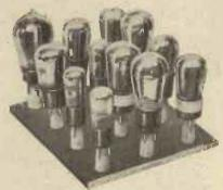
One advantage of the valve rack is that all the valves are readily accessible.
