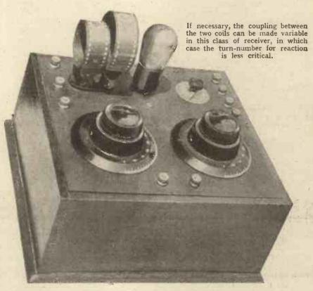
the addition of an L.F. stage is quite A standard one-valve receiver embodying the so-called Reinartz form of reaction, a simple matter. Notice that the Mr. English advocates the use of an additional valve for "reaction," leaving the detector crystal is tapped off a part of the grid free to carry out the task of rectification.
