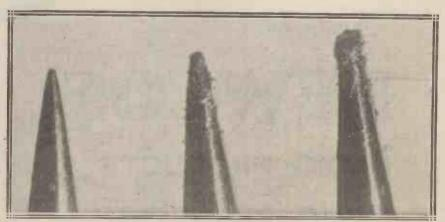
Fig. 7. Showing (left) a new needle; (centre) after one run on a new record; (right) a new needle after one run on an old record.
