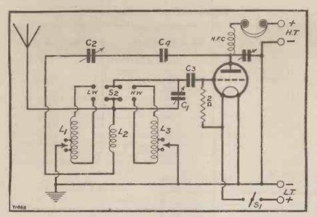
one of the general-purpose type. Connect up a pair of 'phones and your H.T. and L.T. batteries to the terminals marked. You will need about a 60- or 72-volt H.T. battery. and it is best to buy a tapped battery so that you can vary the H.T. until you get maximum results.
