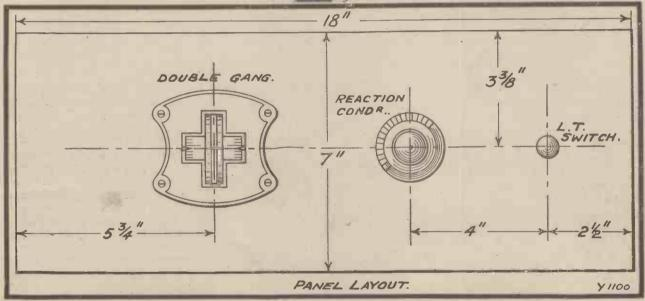
The panel view above this drilling diagram indicates the method of searching when once the drums have been got into step; both are run together with the thumb.
