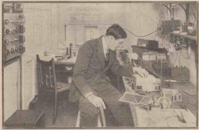
In the "M.W." Research Laboratory : Capt. Eckersley examining one of the experimental receivers under construction. On the left is seen part of the A.C. power board, and to the right the D.C. battery-charging gear.
