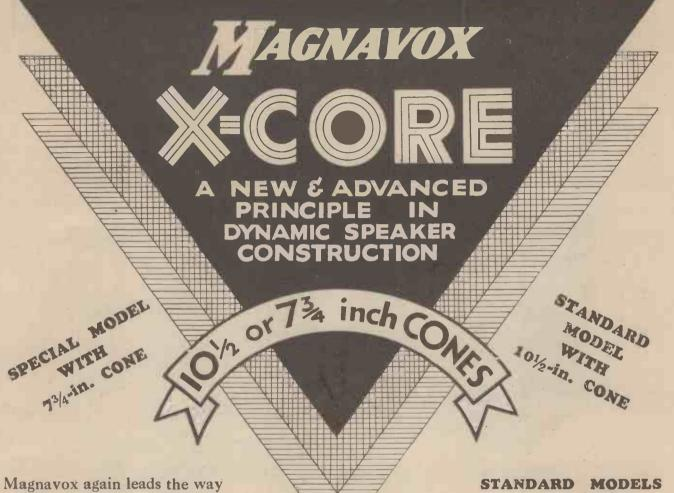
with the new X-Core Dynamics. The X-Core ensures perfect alignment of the inner and outer poles and a true concentric gap in which the moving coil may vibrate. The X-Core is secured in engagement with the main core by means of a bolt running directly through its centre.
