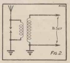
A water-pipe earth is used indoors for stability purposes. If a mains unit of any kind is employed, or the receiver itself is mains driven, the water-pipe connection is unnecessary, as the set will find its stabilising earth in the mains themselves.
