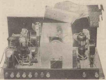
number of circuits arranged in the The "Brookman's" Three incorporated a form of band-pass filter in the intervalve (This set was described in detail in the September issue.) coupling circuits.
