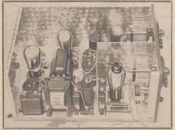
In this general view the set is seen complete except for the fitting of the screening cover and the special screening cap on the S.G. valve. The latter is to be connected, by the by, to the moving plate terminal of the nearest variable condenser.
