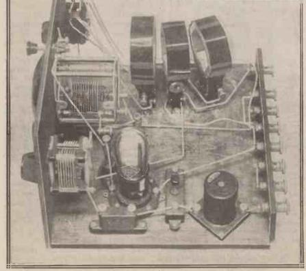
The orientation of the medium-wave coil holder (nearest the terminal strip) is very im-, portant, since it has a great bearing on the smoothness and efficiency of the reaction control.
