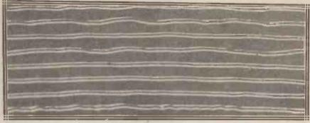
Fig. 4. After 50 times with the Lissen pick-up and a spear-point needle. The grooves show no trace of wear.
