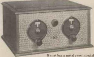
precautions must be taken before a mains unit is used. Remember, it is possible for the whole panel to be "live."
