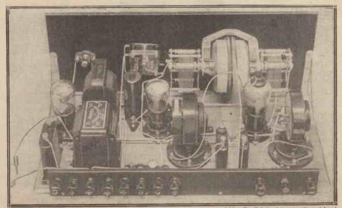
Note how the coils are placed so that the screen intercepts and cuts off their stray fields. The little knob between the aerial and earth terminals controls the series aerial condenser.
