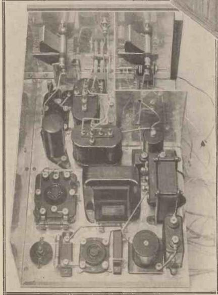
The receiver finished, ready for the fitting of the remaining portions of the screening system. Note how the "ganged " switches are arranged.
