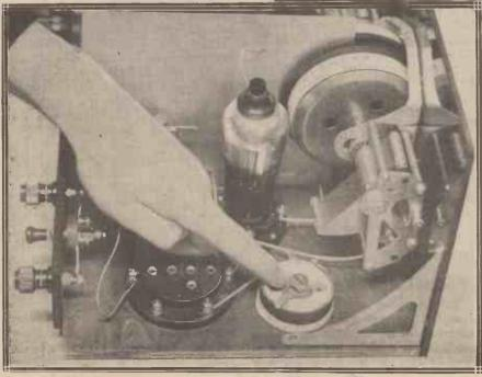
Above, the output filter choke, where low D.C. resistance is to be desired. Below, the "losser" resistance which enables you to flatten out your tuning for the best quality on the local programmes.
