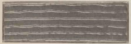
Fig. 3. A section of the same "band" record after the B.T.-H. pick-up has played it 50 times. Little trace of deformation of the grooves is visible. The polish of the record face is worn off, hence the dullness of some of the "crests."
