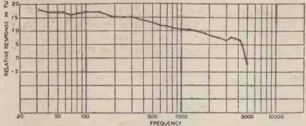
Fig. 2. This pick-up has good bass response though the treble is poorly reproduced.
