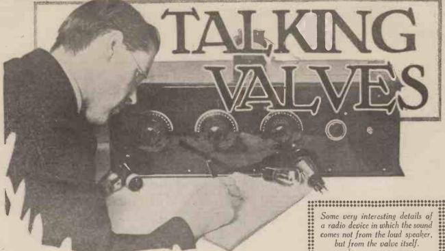
THE three-electrode valve is the focus of so much ingenuity that it is difficult to say where its possibilities will end. As oscillator, amplifier, and rectifier it has for many years been the mainspring of wireless progress in general. Similarly most of the recent advances in picture transmission and in television are due directly or indirectly to its aid.
