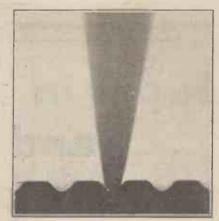
Fig. 6. A fine needle reaches the bottom of the groove and causes less wear, provided it does not "whip" badly.
