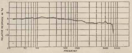
Fig. 3. A curve of a new type of pick-up which has greatly improved high note response.
