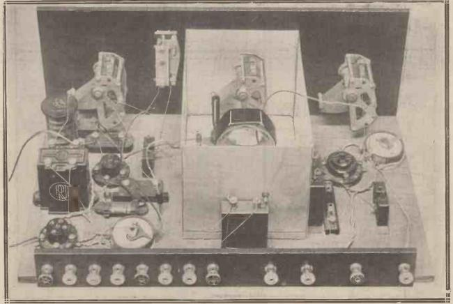
Two potentiometers are required in the A.C. version for the adjustment of the earthing points on the L.T. circuits.
