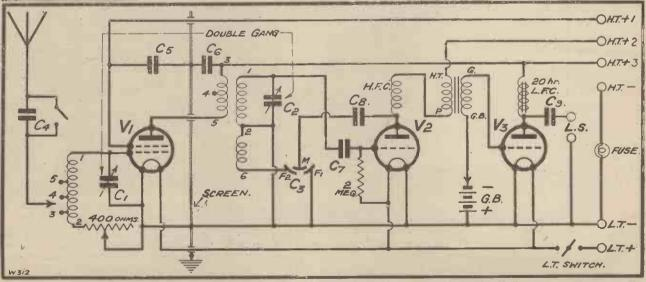
In this circuit diagram you can follow the special arrangements which make the "Eckersley" Three both a high-quality local set and a sensitive long-range outfit. The photo above shows the control for the series condenser  $C_4$ .
