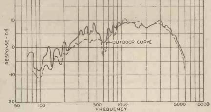
Fig. 7. Response-frequency characteristic of a 32-in. piston-diaphragm loud speaker. Measured in a highly absorbing room and averaged in small region 12 ft. from diaphragm.
