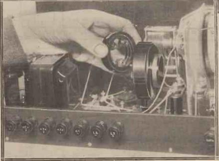
At the top, the control which does NOT upset your tuning (differential reaction condenser). Below and to the left, one of the main controls of selectivity—interchangeable primary windings of different sizes are available for the H.F. transformer.
