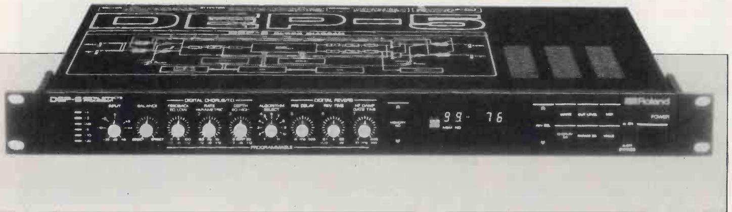
*With the help of 28-bit processing technology, Roland have introduced a signal processor that can generate digital reverb, delay, chorus and flanging effects – and combine them together to produce new treatments. By Paul White.*
