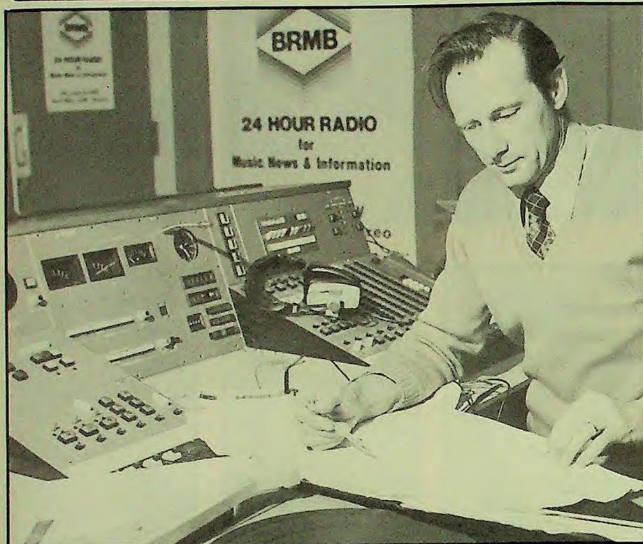
BRMB CHIEF engineer, Dave Wood, makes some last minute checks on the station's new studio equipment, custom built to his specifications. Among the many innovations which it boasts are the ability to handle up to 20 inputs from outside sources, a special phone-in system, plus built-in digital and face clocks.
