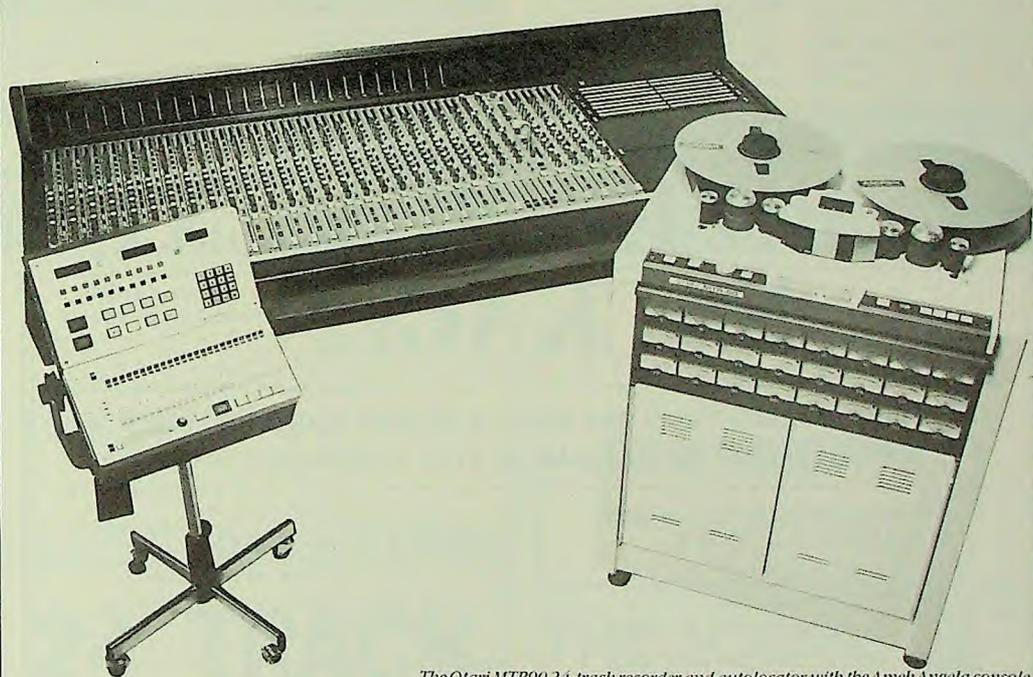
The Otari MTR90 24-track recorder and autolocator with the Amek Angela console
