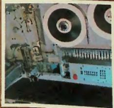
Although the production master is invariably delivered on DAT, most UK cassette manufacturers use analogue duplication. The DAT master is transferred to one inch tape which runs as a continuous loop in a bin master at 64 times normal playing speed. The bin master, running the A side forwards and the B side backwards simultaneously serves up to a dozen separate 'slave machines' which produce the cassette tapes.
