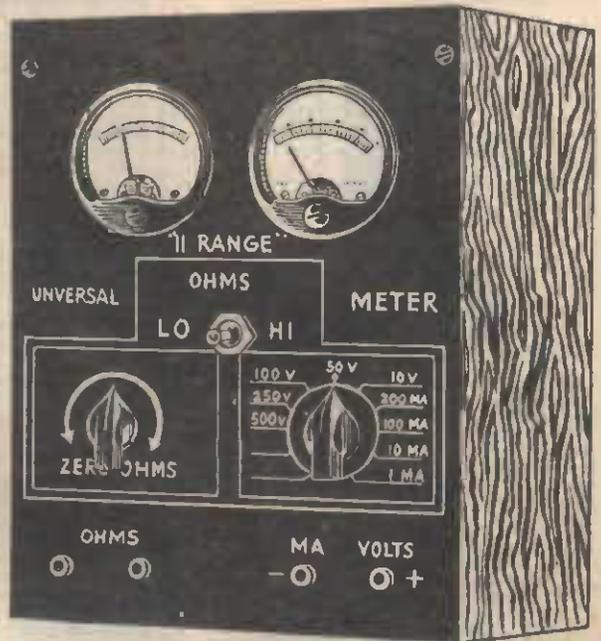
THIS multimeter kit consists of a circuit built around two 0-500 micro ammeters, one being calibrated to read milliamps and volts and the other to read ohms. As these meters have a sensitivity of 2000 ohms. per volt it will be seen that this multimeter is capable of giving quite accurate readings in any work it is liable to be put to by radio men. The following ranges are available:—
