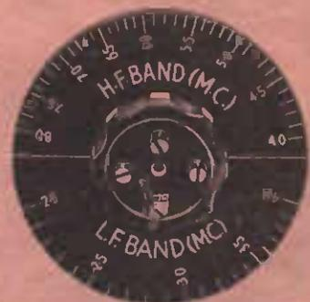
As used in ZCI Transceivers. Suitable for receivers or transmitters. Can be set for two preset frequencies, with flick tuning mechanism. Cat. No. AX1090/4 **1/6**
