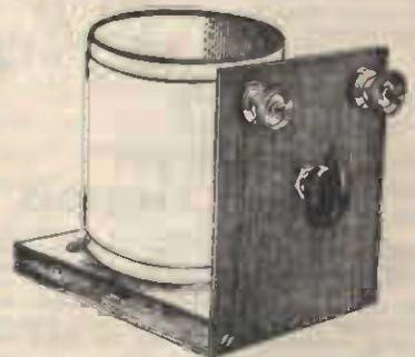
Used to separate stations which interfere or overlap each other. Gives sharper tuning to all size Receivers from Crystal Sets onwards. Will also act as a booster for strengthening weak stations.
