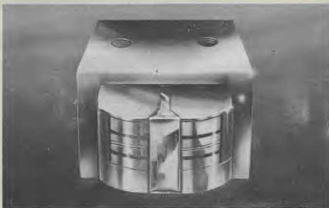
THE FIRST GLASS FERRITE TAPE HEAD: AN ORIGINAL.
