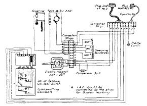
quick brown fox jumps over the lazy dog + ... Assuming that the duplex circuit is already balanced, the sending test is made first in one direction and then in the other, and finally in both directions simultaneously.
