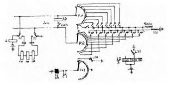
trolled by relay LS which, in turn, controls relay LD. So long as battery and earth are connected to the junction at the manual exchange, relay LS remains operated; relay LD is also operated. When the call indicator apparatus is ready to receive the call, the battery and earth are removed and substituted by the three decoding relays. Relay LS now releases and, after an interval, relay LD releases and closes the driving circuit of the pulse send switch.
