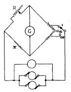
ance is read directly from the scale, the range of the instrument being from  $r_{1,000}\Omega$  to 20 M $\Omega$ .
