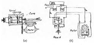
speed. The phase relationship is the angular displacement between the brushes at the correcting and corrected stations required to ensure correct reception of signals.
