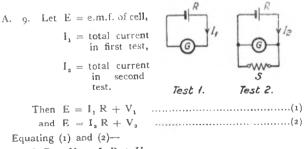
$$I_1 R + V_2 = I_1 R + V$$
