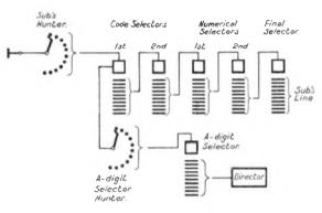
The A-digit selector returns dialling tone to the calling line and, on receipt of the first train of dialled impulses, steps its wipers to the level dialled and searches for a free director. Should all the outlets be engaged, the selector steps its wipers to the 11th position and connects busy tone to the caller.
