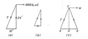
this condition, can be resolved into horizontal and vertical components; the horizontal component, though small, is in the opposite direction to the pull of the line wires and hence the effective stress in the line wires, to be counteracted by the tension in the stay, is less than when the pole is vertical.
