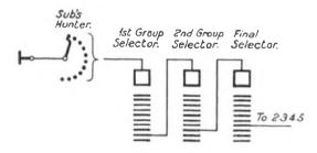
(b) Ringing tone is connected to the calling line from the final selector on completion of dialling and the seizure of the called line.
