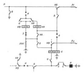
If the first outlet is engaged, the earth on the P1 wiper is extended through contacts of HA and B relays to one side of relay HA; the other side of this relay is also connected to earth through contacts of relays HB and B, and the off-normal springs. Relay G operates via the rotary interrupter springs to the earth on the P-wire.
