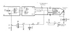
circuit incoming from a trunk exchange. Relay AC, operated by ringing current from the Trunk exchange, operates relay R which, in turn, applies ringing current to the called subscriber's line.
