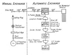
exchange is designed to place complete control of the setting up of the call in the hands of the A-operator. The diagram here reproduced represents the through circuit in schematic form.
