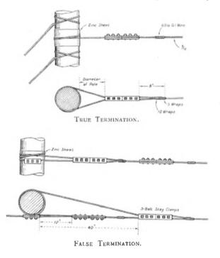
pole provided with line stays, a false termination is made as shown.
