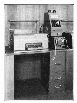
FIG. 3.—AUTOMATIC TRANSMITTER POSITION WITH SIGNALLING UNIT, TG, NO. 23, AND SWITCHING KEY FOR CONNECTING THE AUTOMATIC TRANSMITTER TO ANOTHER POSITION.
