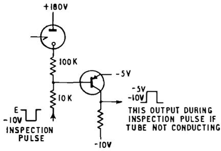
(b) Connexion of Cold-Cathode Tubes to Transistors
