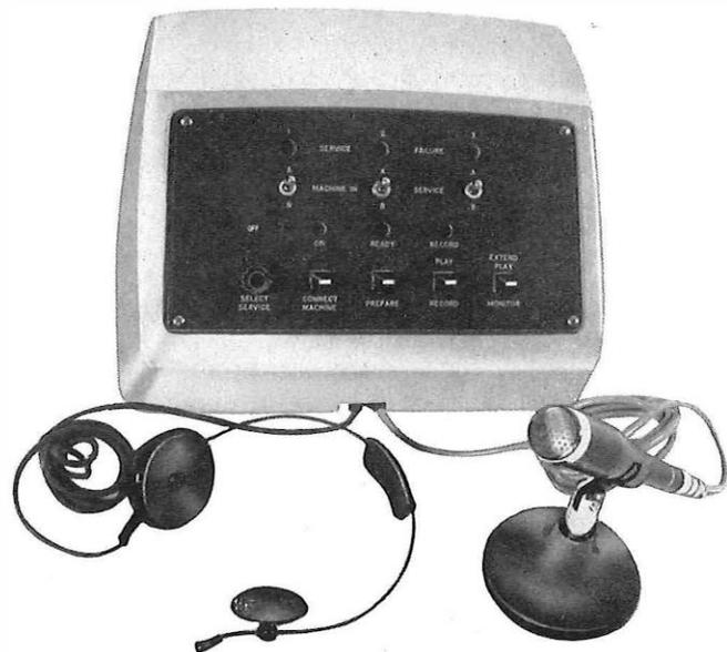
FIG. 4—CONTROL PANEL FOR SMALL CENTRES
