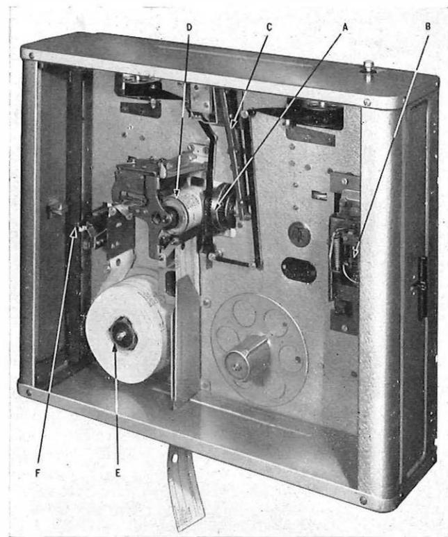
A—Typehead. B—Uniselector. C—Hammer. D—Platen.
