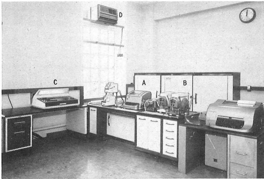
A—Power cabinet B—Logic cabinet C—Keyboard D—Air-conditioning unit
