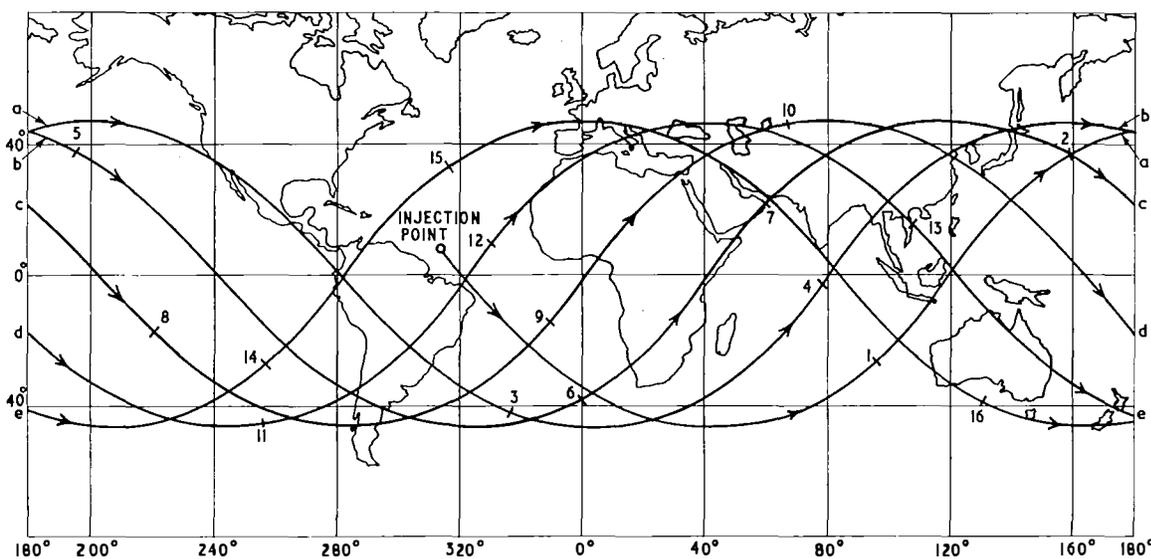
Numbered marks on plot indicate hours elapsed after injection
