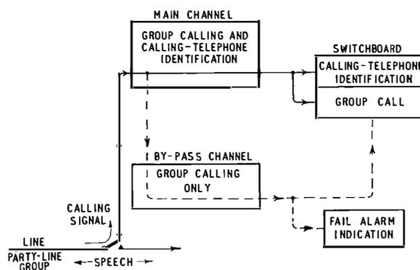
FIG. 1—BASIC SIGNALLING ARRANGEMENT
