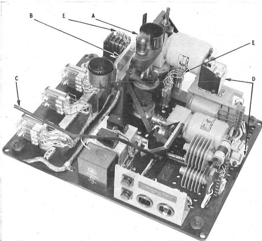
A—Film sprocket. B—Glass pressure-plates.
