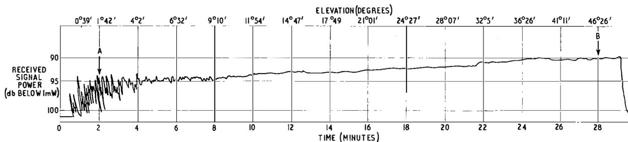
At elevation A the satellite was 10,000 km from Goonhilly
