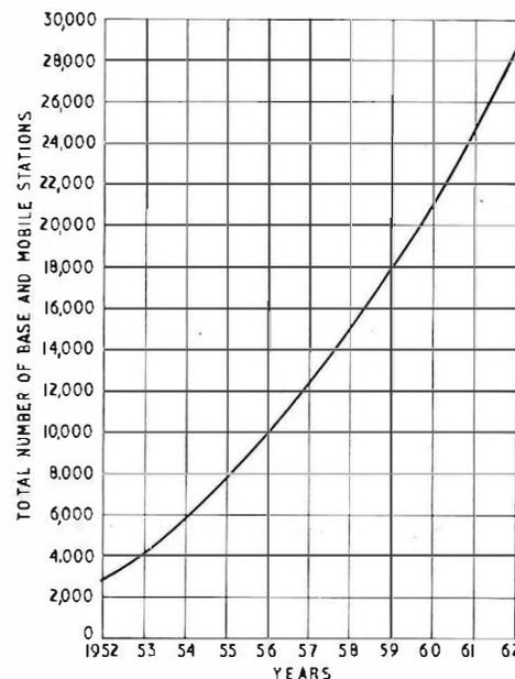
The graph shows the total number of base and mobile stations, the ratio of mobile to base stations being about 10:1.
