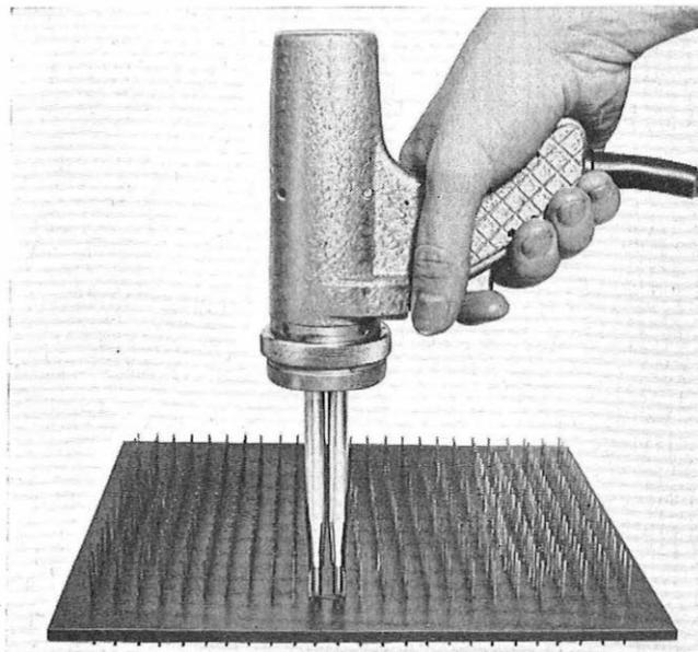
FIG. 3—DOUBLE-HEADED WRAPPING GUN IN ACTION
