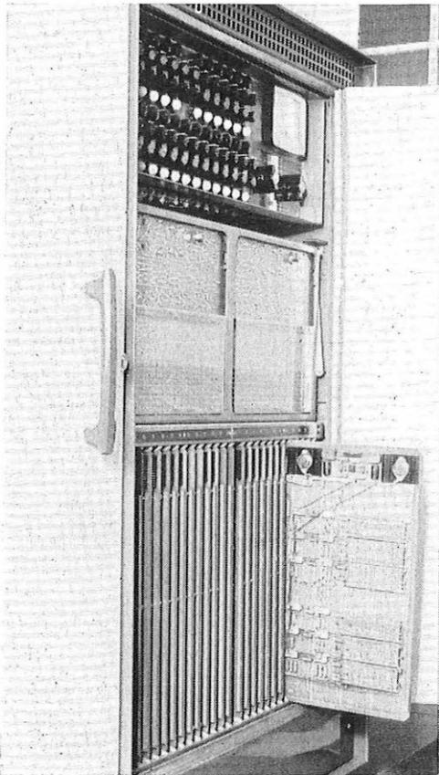
FIG. 2—LOGIC CABINET WITH A LOGIC BOARD WITHDRAWN
