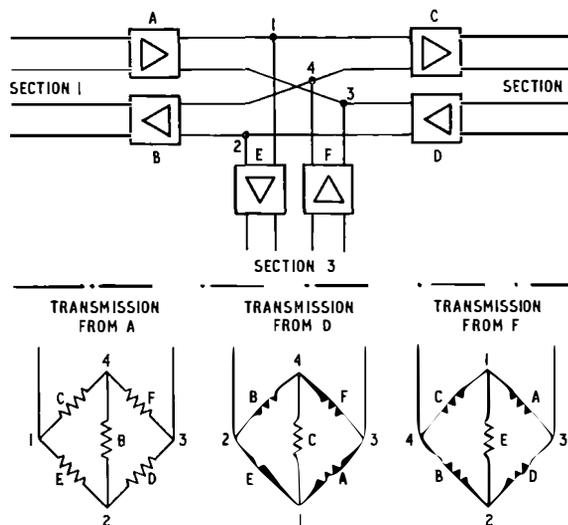
FIG. 1—FOUR-WIRE BRIDGE OMNIBUS CIRCUITS
