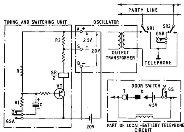
FIG. 3—CIRCUIT OF ROADSIDE-CABINET EQUIPMENT
