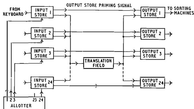
FIG. 4—SIMPLIFIED DIAGRAM OF TIME-SHARING ARRANGEMENT
