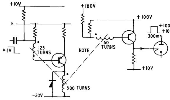
(a) Connexion of Transistors to Cold-Cathode Tubes
