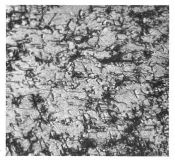
Magnification: × 25 FIG. 4—TOPOGRAPH OF SILICON SLICE WITH DISLOCATION DENSITY OF 10<sup>1</sup> LINES/cm<sup>2</sup>
