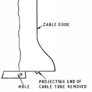
FIG. 3-CABLE TUBE CUT AWAY TO ACCOMMODATE ATTACHMENT A
