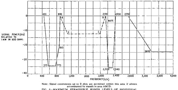
FIG. 6-MAXIMUM PERMISSIBLE POWER LEVELS OF INDIVIDUAL SIDEBAND COMPONENTS TRANSMITTED TO LINE BY DATEL MODEM
