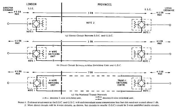
FIG. 7-TRANSMISSION LOSSES ON CALLS BETWEEN LONDON S.S.C.S AND THE PROVINCES
