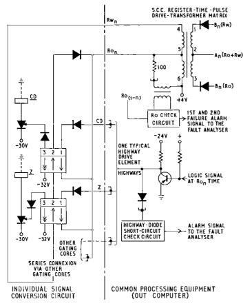
FIG. 6-E.C.E. TO S.C.C. HIGHWAYS SYSTEM
