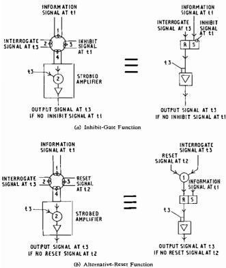
FIG. 15-FOUR-WINDING-CORE FUNCTION CONTROL ELEMENT
