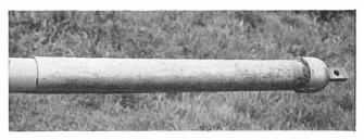
Fig. 4—duct, sleeve and cap ready for attaching to moleplough
