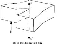
FIG. 2—SCHEMATIC DIAGRAM OF A SCREW DISLOCATION
