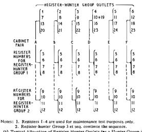
(b) Typical Allocation of Register-Hunter Outlets for a Hunter Group in a 6-Cabinet-Pair Scheme
