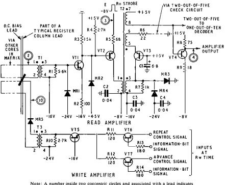
Note: A number inside two concentric circles and associated with a lead indicates the relevant waveform illustrated in Fig. 11 FIG. 13—CORE-TYPE CENTRAL-DATA-STORE. READ-AMPLIFIER AND WRITE-AMPLIFIER CIRCUITS
