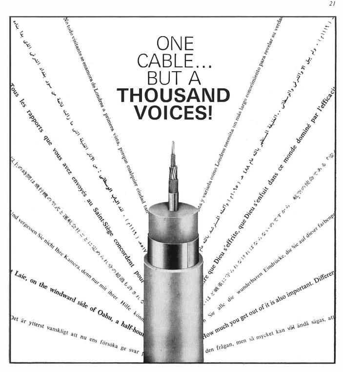
The first submarine cable, laid between England and France in 1891, provided one or two speech circuits. The Atlantic telephone cable system of 1956 provided thirty-six circuits.
