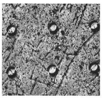
Magnification: x25 FIG. 8—TOPOGRAPH SHOWING DIFFRACTION CONTRAST FROM EDGES OF WINDOWS ETCHED IN OXIDE LAYER
