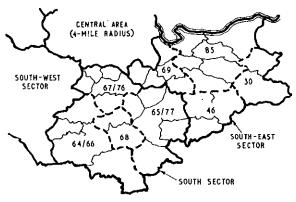
Note: 46, 66, etc., denote the first two digits of exchange codes FIG. 6—ALLOCATION OF ALL-FIGURE NUMBERING CODES IN LONDON
