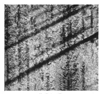
Magnification: ×25 FIG. 6—TOPOGRAPH SHOWING SLIP AFTER EPITAXIAL DEPOSITION
