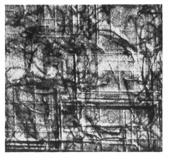
Magnification: ×25 FIG. 9---TOPOGRAPH SHOWING PHOSPHOROUS DIFFUSION-INDUCED SLIP
