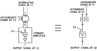
FIG. 14--THREE-WINDING-CORE FUNCTION CONTROL ELEMENT
