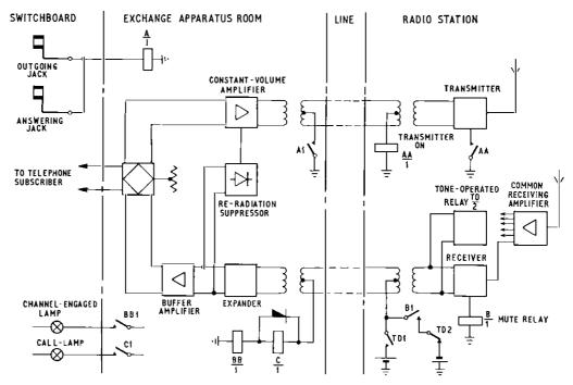
FIG. 2—GENERAL ARRANGEMENTS OF TRAFFIC CHANNELS
