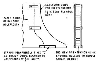
FIG. 1-EXTENSION GUIDE FIXED TO PLOUGH BLADE
