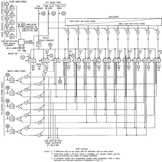
FIG. 12-FUNCTIONAL DIAGRAM OF THE 10-STAGE FUNCTION UNIT
