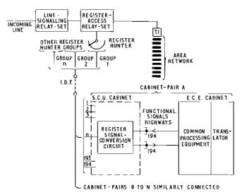
(a) Schematic Diagram of Trunking Arrangements
