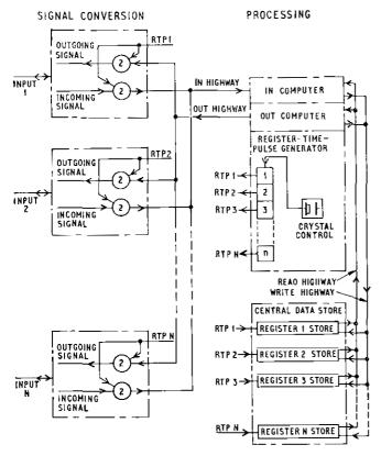
RTP—Register time pulse FIG. 3—SCHEMATIC DIAGRAM OF A TIME-SHARED COMMON-PRO-CESSING EQUIPMENT SERVING N INPUTS VIA T.D.M. HIGHWAYS
