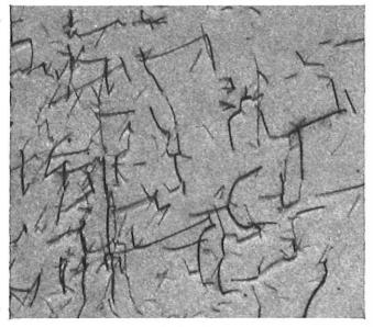
Magnification: x25 FIG. 3—TOPOGRAPH OF SILICON SLICE WITH DISLOCATION DENSITY OF A FEW HUNDRED LINES/cm<sup>3</sup>
