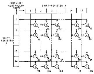
FIG. 4—FUNCTIONAL DIAGRAM OF MAIN SEQUENCING MATRIX
