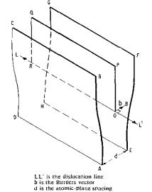
FIG. 1.-SCHEMATIC DIAGRAM OF AN EDGE DISLOCATION
