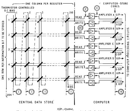
Note: A number inside two concentric circles and associated with a lead indicates the relevant waveform illustrated in Fig. 11 FIG. 9—SCHEMATIC DIAGRAM OF CENTRAL DATA STORE AND COMPUTER-FUNCTION STORE
