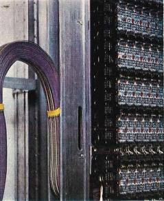
(TOP LEFT) Part of a cross-point switching frame also showing associated electronic modules. (TOP RIGHT) A sub frame withdrawn for inspection showing the method of tape wiring.
