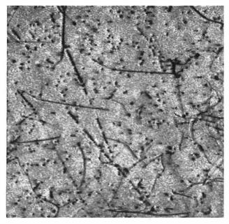
Magnification: × 25 FIG. 7—TOPOGRAPH OF SILICON SLICE WITH OXIDE LAYER 0.8 µ THICK ON BOTH FACES
