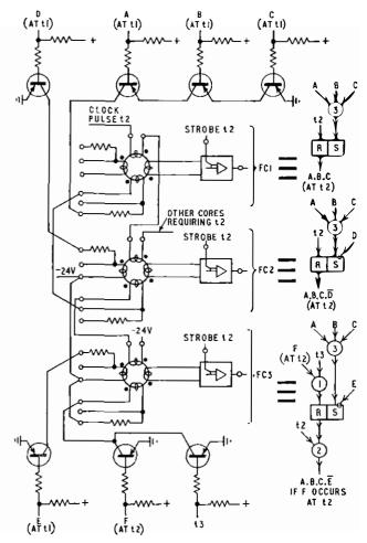
FIG. 17-TYPICAL CORE-TRANSISTOR MANIPULATIVE CIRCUIT
