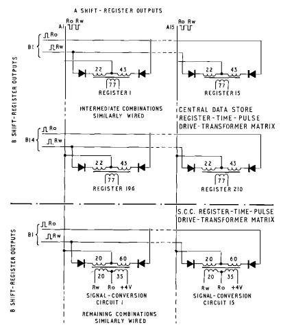
FIG. 5-CIRCUIT ARRANGEMENTS OF MAIN SEQUENCING MATRIX
