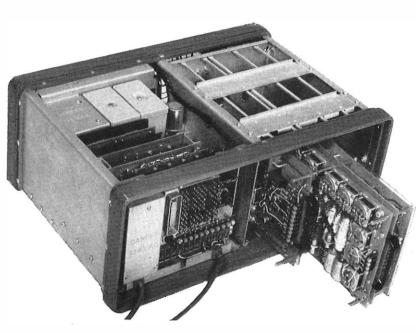
FIG. 4 -DATEL MODEM No. 1A WITH COVERS REMOVED
