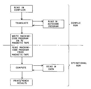
FIG. I-PROCESSING AN AUTOCODE PROGRAM
