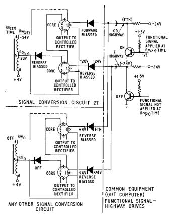
FIG. 7—ANALYSIS OF CONDITIONS DURING RO1T TIME FOR CIRCUIT OF FIG. 6
