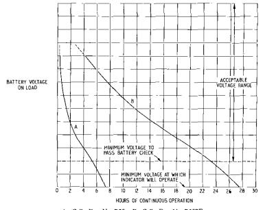
A—Cells, Dry, No. R20. B—Cells, Dry, No. R20PF FIG. 4—COMPARISON OF BATTERY ENDURANCE FOR INDICATOR, GAS, No. 5
