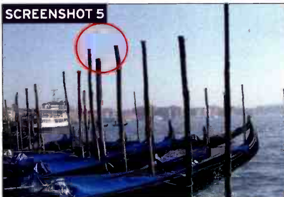
Spot the spot – caused by dust in the Finepix S602 Pro's CCD
