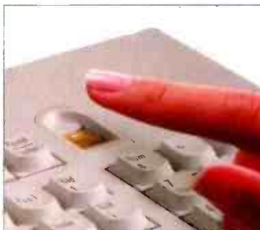
The Sicrypt system from Fujitsu-Siemens uses smartcard or fingertip scanning to recognise a user
