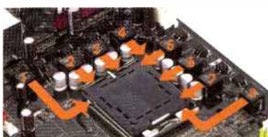
8-phase design operate at 15°C lower than conventional power solution
