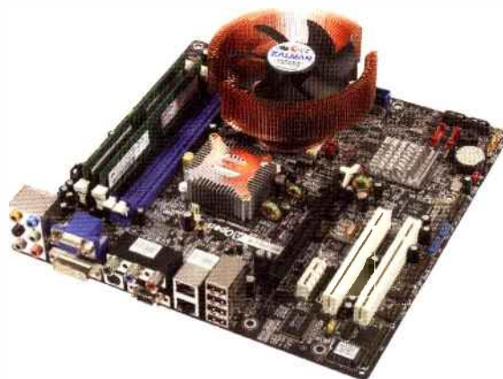
The Aopen i915GMm-HFS motherboard, pictured with a Zalman CNPS7000B-Cu heatsink. This heatsink isn't designed for the Pentium M, but with alternative mounting studs can keep it cool without the need for a fan
