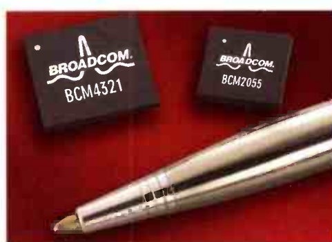
Broadcom is selling its pre-N chipset under the Intensi-fi brand. Its radio chip (on the right of the picture) implements multiple 2.4GHz and 5GHz transceivers; on the left is the media-access controller
