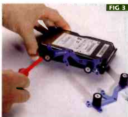
The most important step: physically insulate the hard disks from the PC chassis using a product such as the Noiseblocker NB-X Swing
