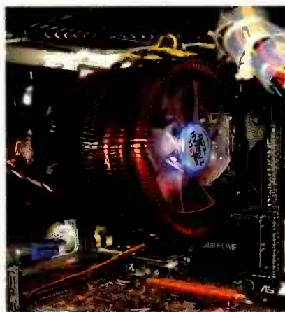
A Zalman fan keeps the Core 2 Duo processor cool
