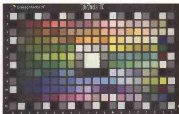
This test target is used to assess colour reproduction
