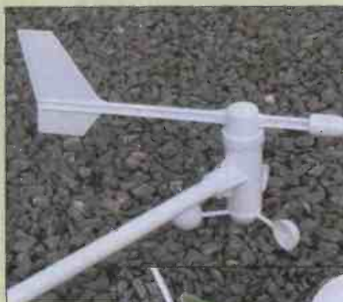
The anemometer has spinning cups to measure wind speed. The vane on top shows wind direction
