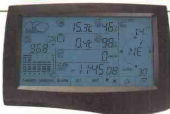
The Oregon Scientific WMR928NX touchscreen base station shows current readings from sensors
