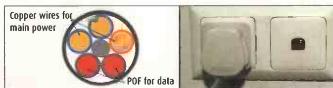
Left: Cross-section of fibre-power cable; right: combined data and mains socket
