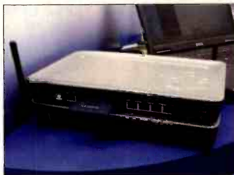
Vendor Trust Eli says a PC Card slot on this router enables it to support secure 3G, Wifi or Wimax links
