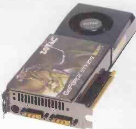
**A** standard GeForce GTX 275 is a cut-down GTX 285, with less memory and a narrower memory interface. The GTX 275 isn't the fastest card around, but is excellent value for money, priced to compete directly with ATI's Radeon HD4890.
