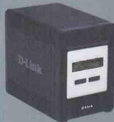
'D-Link's DNS-343 storage device can accommodate up to four SATA disks, but lacks external drive and backup facilities'
