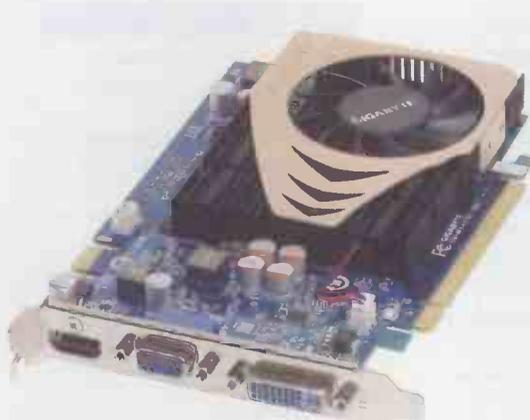
400MHz GDDR2 memory (800MHz effective) running through a 128-bit bus. This isn't nearly as impressive as the more expensive cards on test, and not well suited for modern games, even at lower resolutions.
