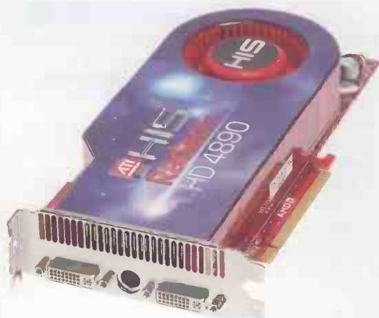
**T**he 4890 is currently the fastest single-GPU card that ATI produces, but it isn't radically different from the 4870. The RV790 chipset is still based on a 55nm process and many aspects of the card are unchanged, such as the number of stream processors. The main difference is that ATI has rearranged the components and tweaked them to coax extra performance from the same design, improving the card's thermal efficiency and allowing it to ship the 4890 with faster clock speeds.
