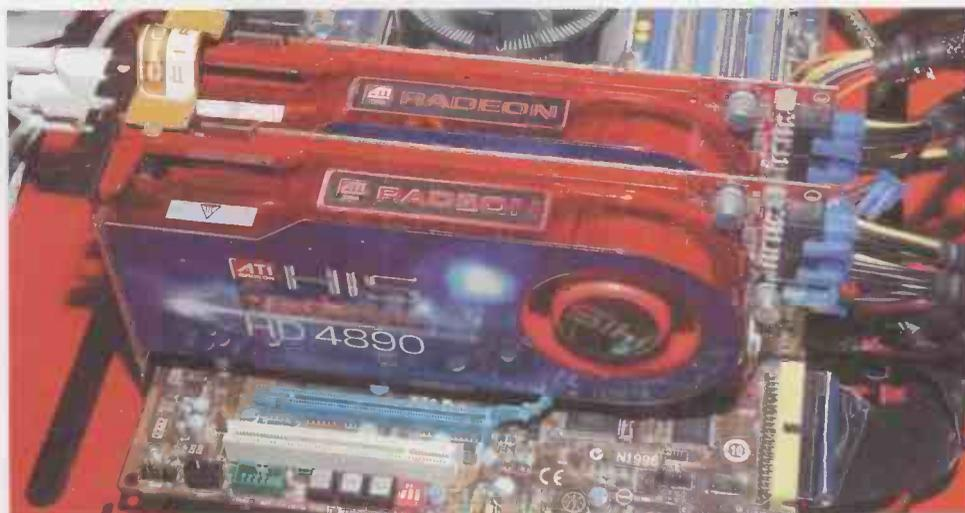
Two Radeon HD4890s, four six-pin power connectors, four monitor outputs, one Crossfire connect, plenty of performance
